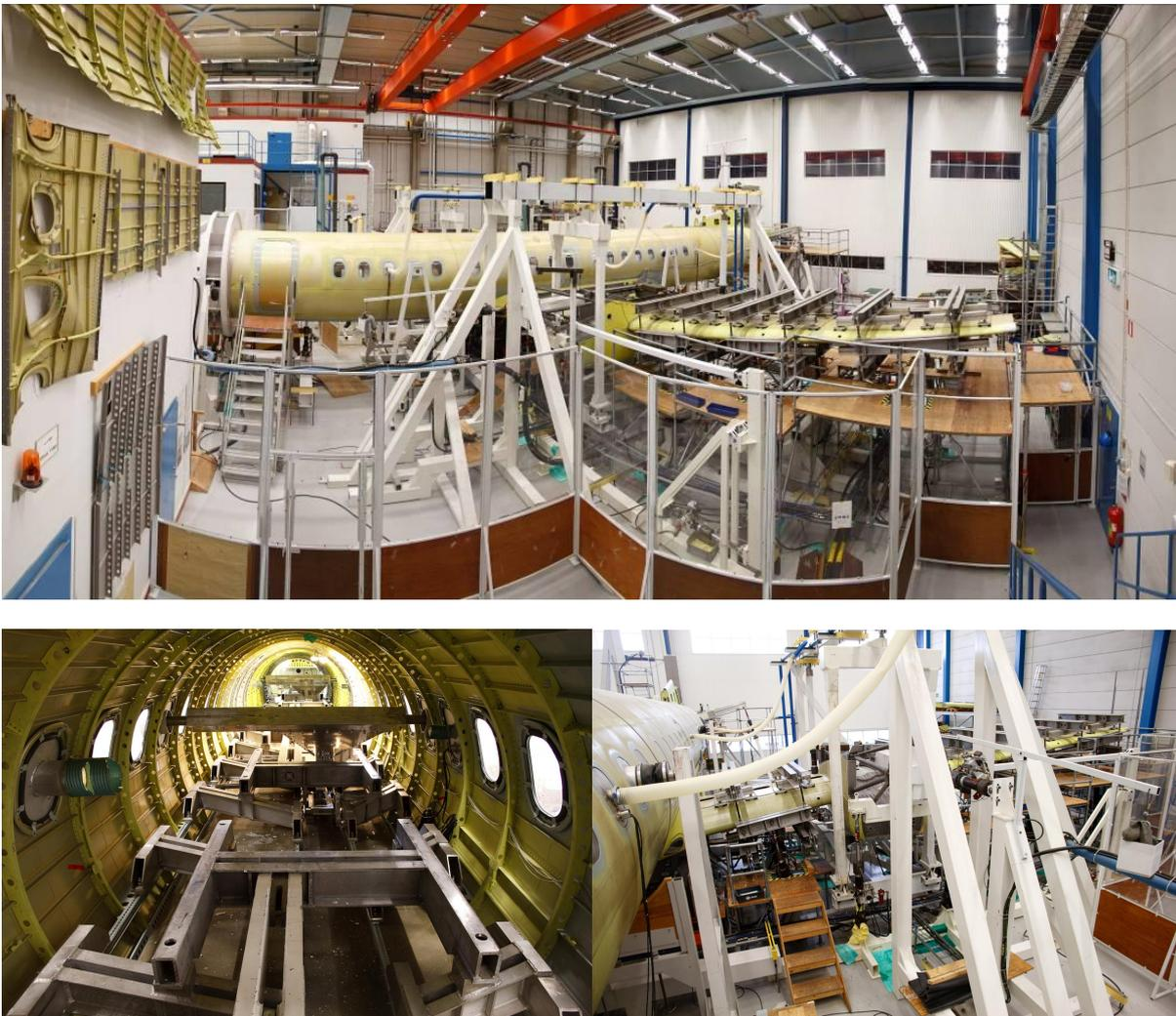
*Figure 3.3.2-1 Saab 2000 Wing/Fuselage Fatigue and damage tolerance test*
