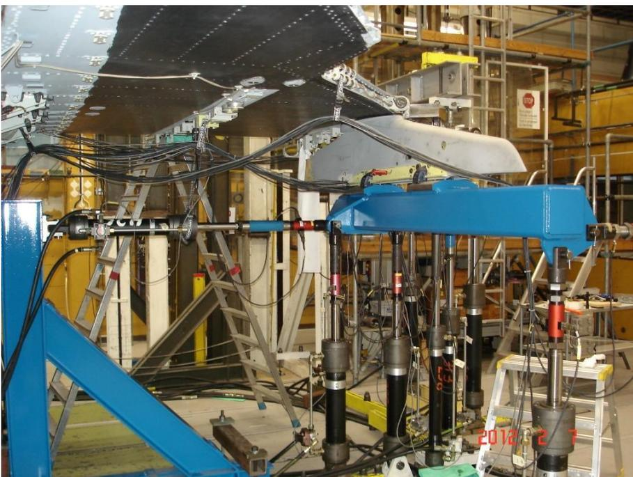
Figure 3.3.4-1. Test setup with loading of pylon station 3.
