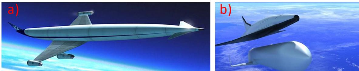
Figure 3.5.4-1: a) LAPCAT A2 hypersonic Mach 5 Civil Transport, b) SpaceLiner hypersonic passenger transport
