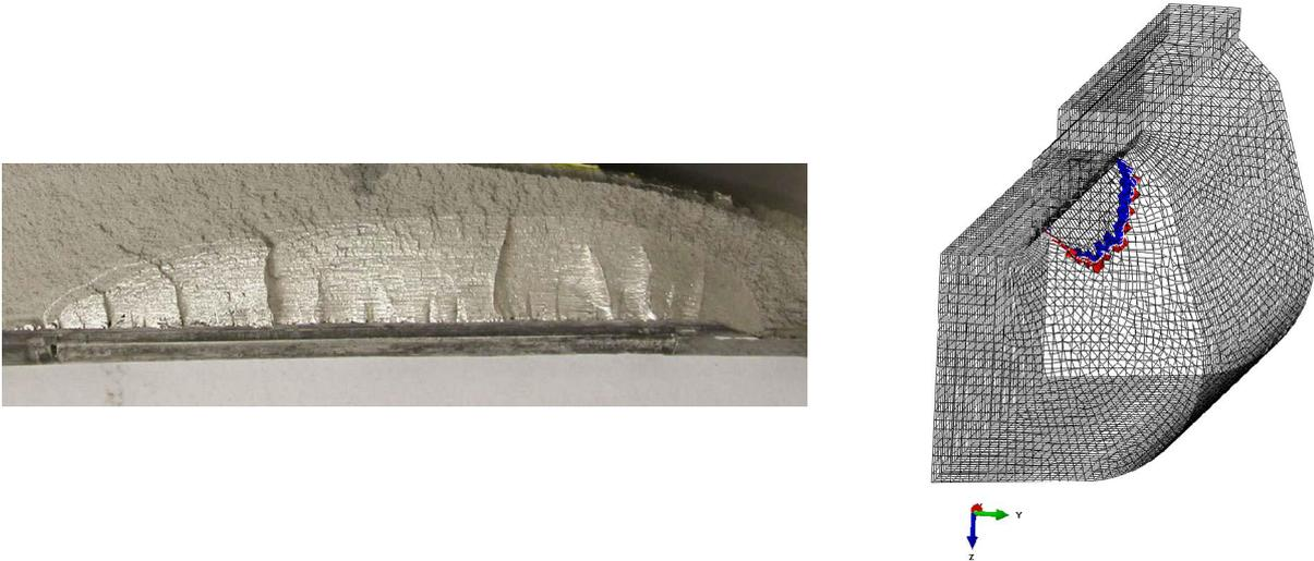
Figure 3.3.6-2. The fracture surface of test specimen and crack growth pattern in the analysis
