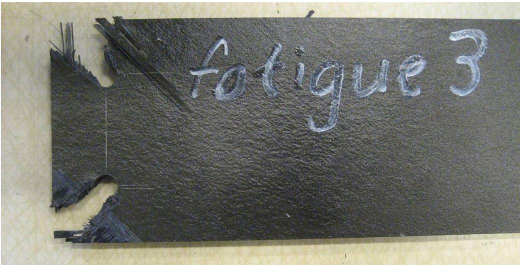
Figure 3.5.1-5 Biaxially loaded specimen after failure.
