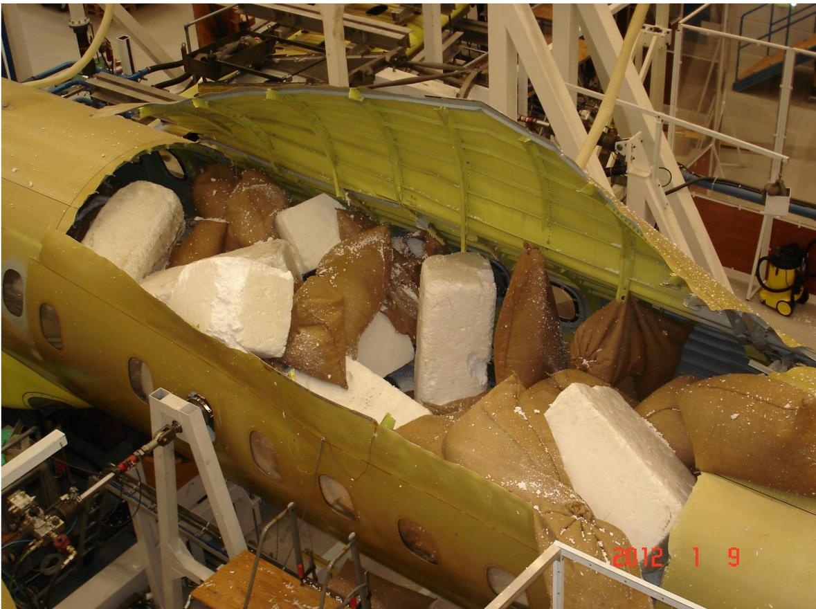
Figure 3.3.2-12 Final failure of the upper portion of the fuselage
