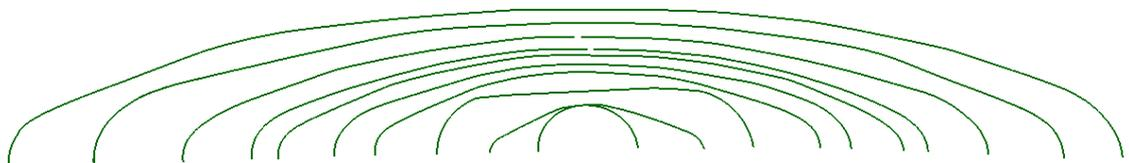
Figure 5 Crack front lines during growth edge crack in a gear tooth
