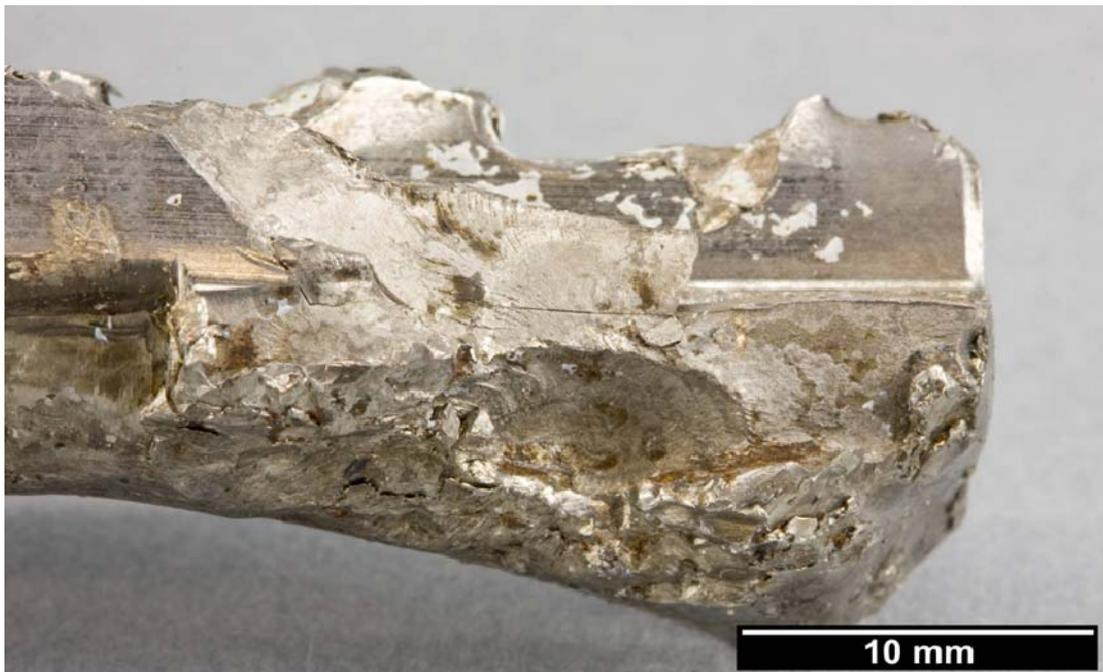
*Figure 2: Fatigue fracture surfaces on a fragment of the failed gear*
