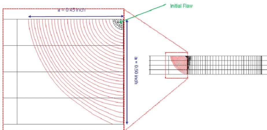
Figure 2 Crack growth with residual stresses
