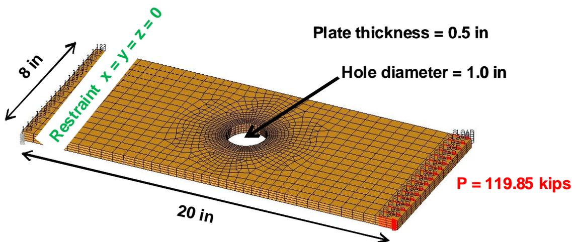
Figure1: Plate with a hole: Model geometry
