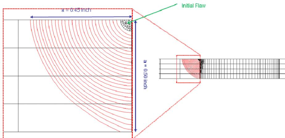
Figure 2 Crack growth with residual stresses
