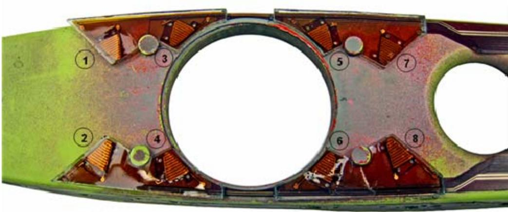
Figure3: Encapsulated sensor elements with their numbering convention on the Gazelle rib
