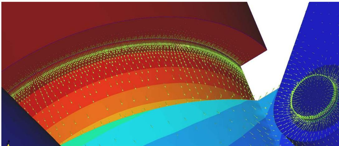
Figure 8 Illustration of tangential current flow and potential gradient through the thin film electrolyte (highest galvanic stress)
