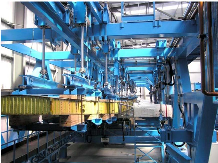
*Figure 1: Wing Fatigue Test Article and Rig Structure*
