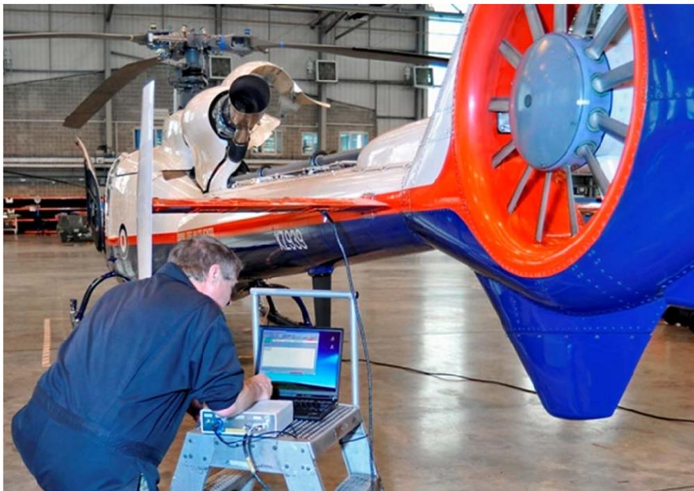
Figure 6. Routine structural health monitoring of the Gazelle stabiliser is now being carried out by aircraft technicians at Boscombe Down.
