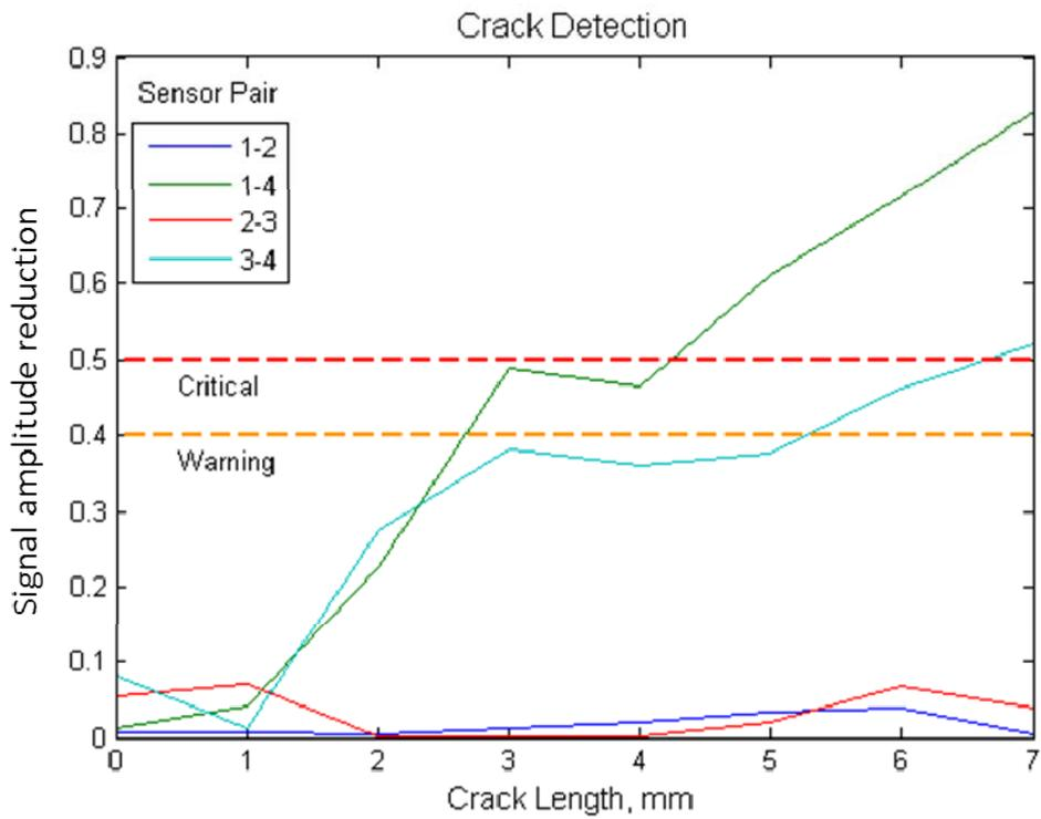
Figure 5: Graph of reduction in the transmission signal amplitude between various sensor pairs with the increasing length of a simulated crack from the spar tube aperture towards the rivet adjacent to sensor 4 (see Figure 3).
