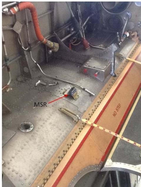
Figure 6: MSR located on Puma fuselage for road transport
