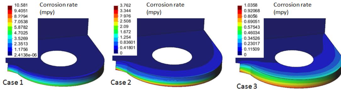
Figure 7 Illustration of corrosion rate (different coating extent on stringer)
