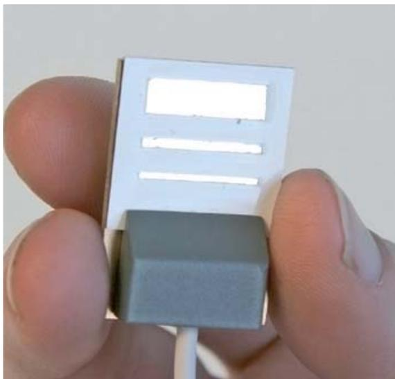
Figure 1: Corrosion sensor - resistive
