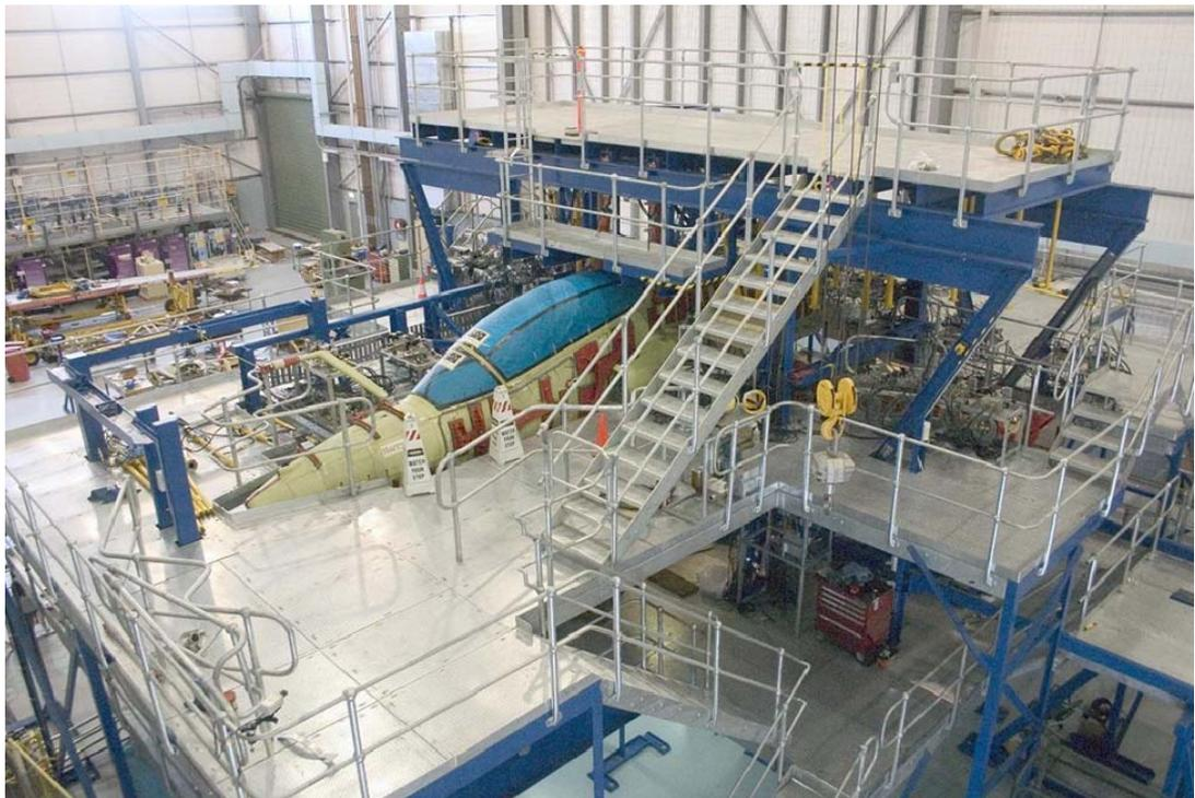
*Figure 1: LIF full scale fatigue test*
