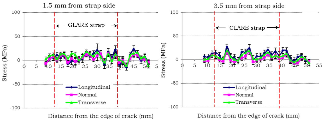
*Figure 1: Residual stress measurements in M(T) specimens due to GLARE strap bonding*
