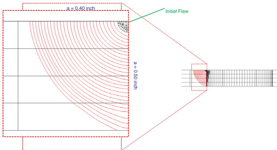
Figure 1 Crack growth without residual stresses
