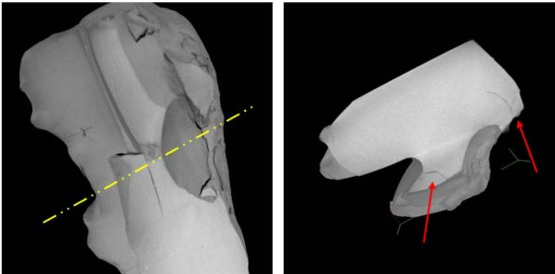
*Figure 3: X-ray tomography images showing a cross-section of the gear fragment viewed in the direction of the yellow arrow. Sub-surface cracks are indicated by the red arrows*
