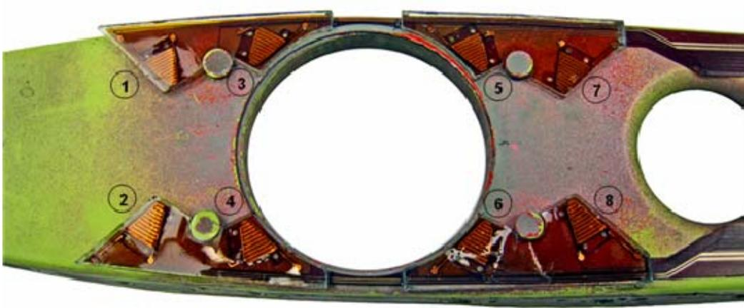
Figure3: Encapsulated sensor elements with their numbering convention on the Gazelle rib
