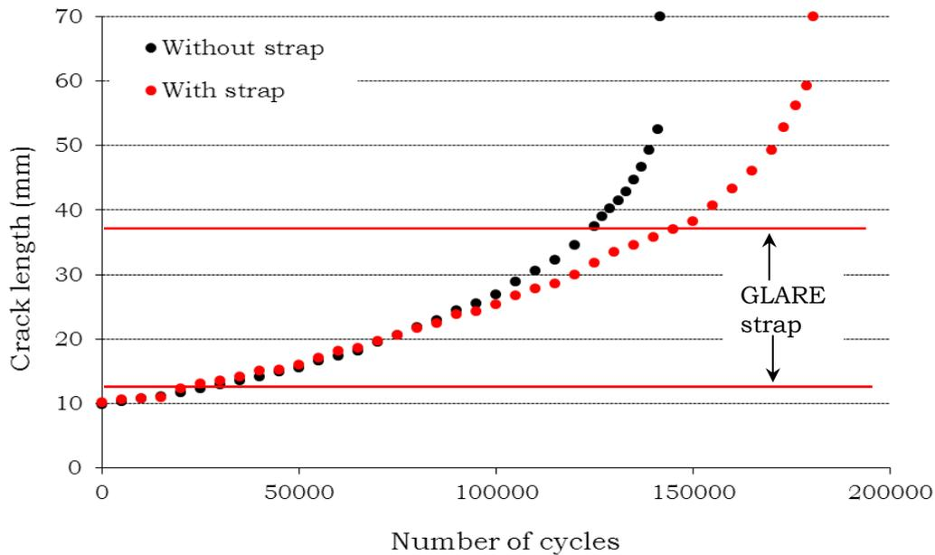
Figure2: Fatigue life of M(T) specimen with and without GLARE strap
