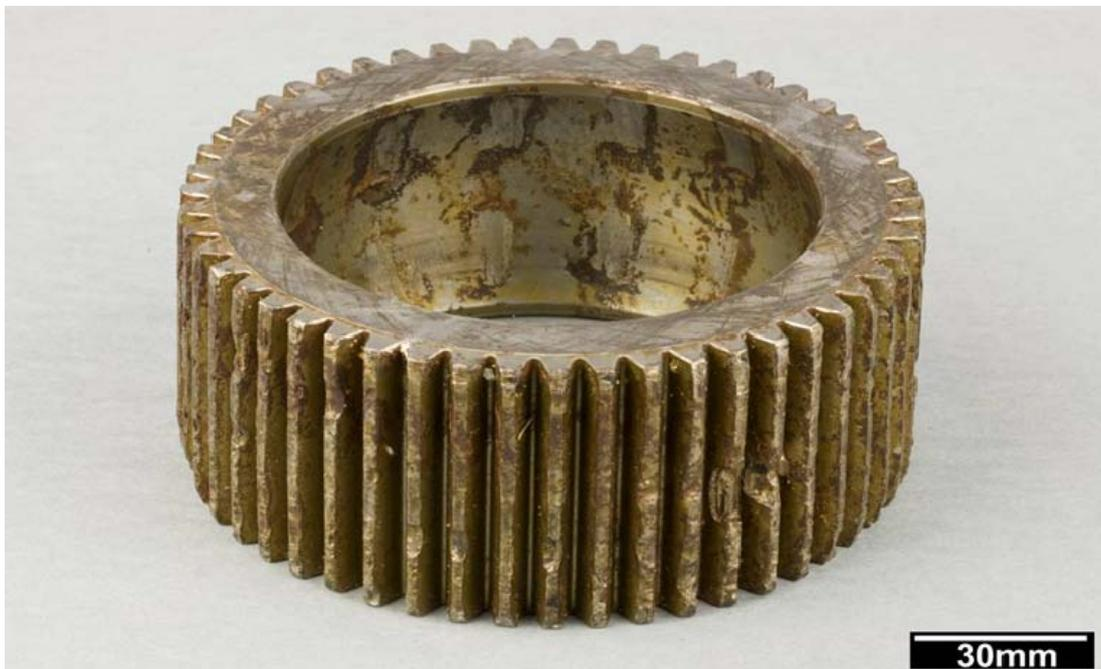
*Figure 1: Intact but damaged gear showing spherical bearing surface inside*
