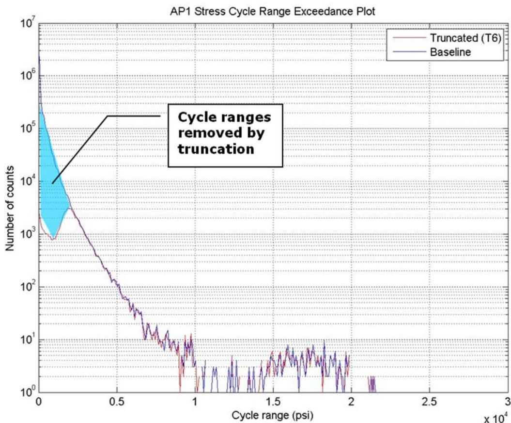
Figure 2: Impact of truncation on an Analysis Point's (AP) retained cycles
