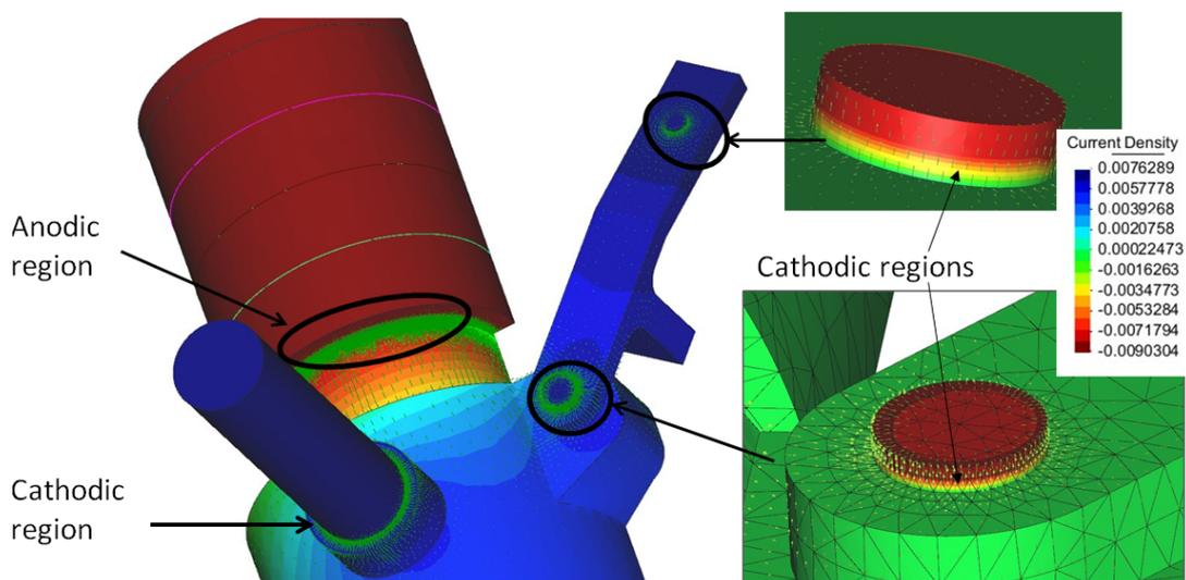
Figure 9 Illustration of the distribution of current density
