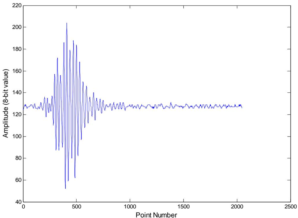
Figure 4: A typical signal from an opposing sensor pair (sensor 4 to sensor 1)
