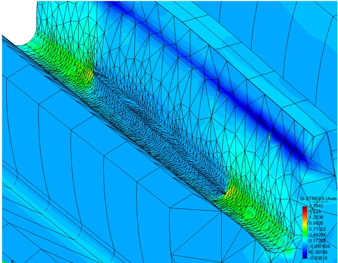
Figure 6 Deformed plot of the crack after a number of crack growth steps
