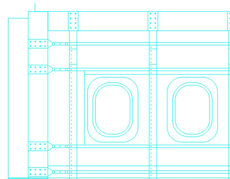
Figure 3 Example of stiffened panel structure (courtesy of R.Citarella, University of Salerno)
