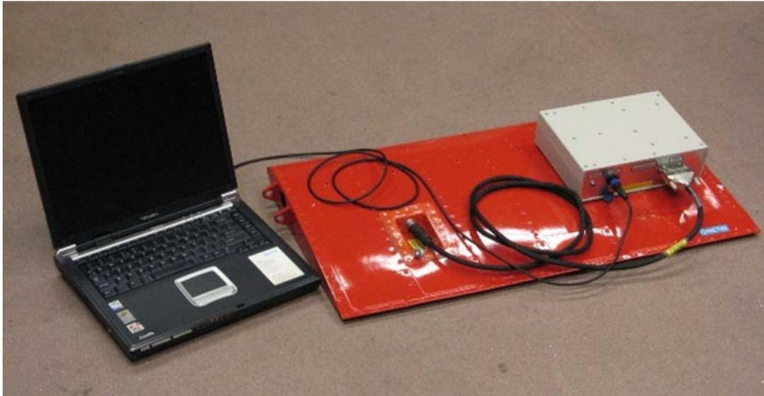
*Figure2: QinetiQ Prototype Gazelle SHM System showing the prototype Hand-Held Transceiver*
