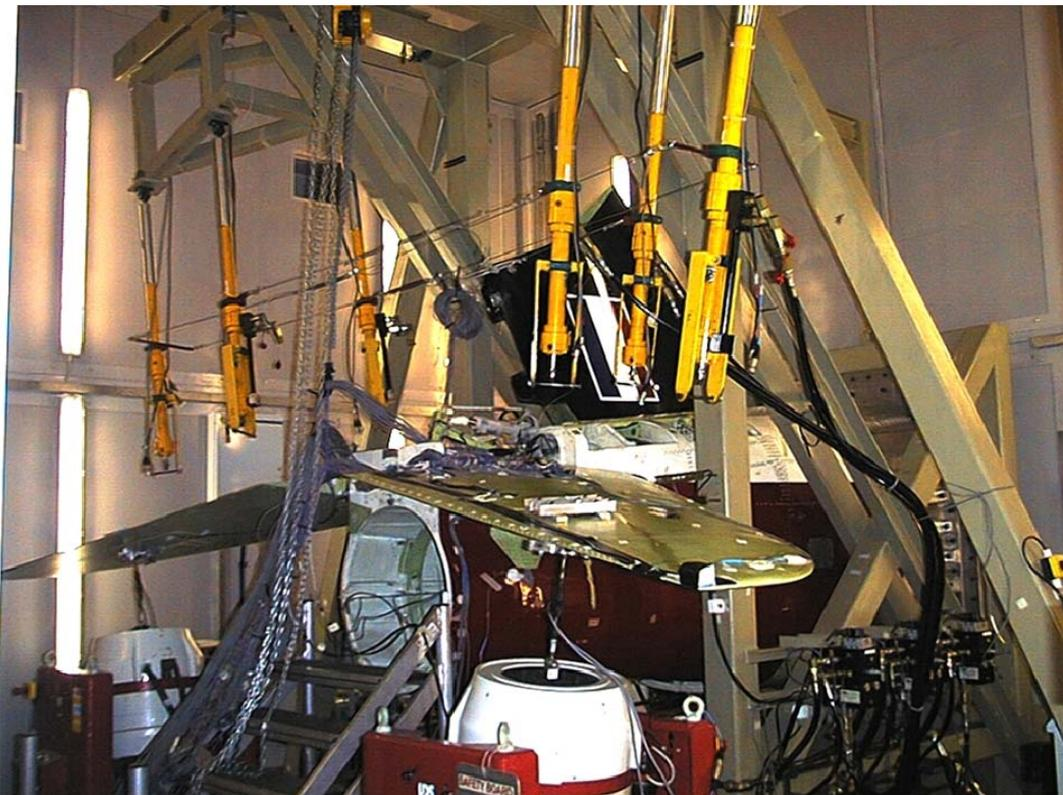
*Figure 1: Hawk tailplane full scale fatigue test*
