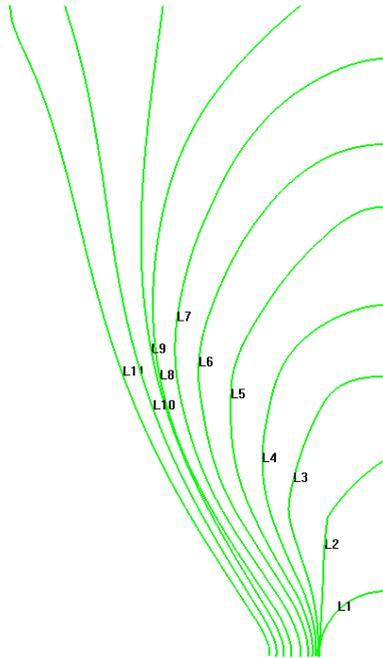
Figure 4 Crack front lines during growth – simple corner crack in a box
