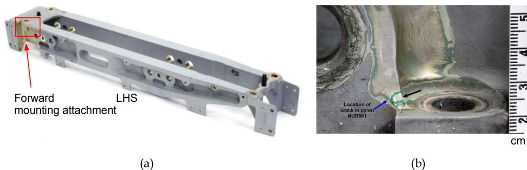
Figure 27. (a) SUU-62 centreline pylon frame; (2) Typical crack locations next to the forward LHS mounting attachment.
