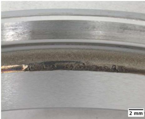
Figure 3 spalling damage on the outer race
