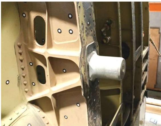
Figure 1 The F/A-18A/B Y508 shear post
