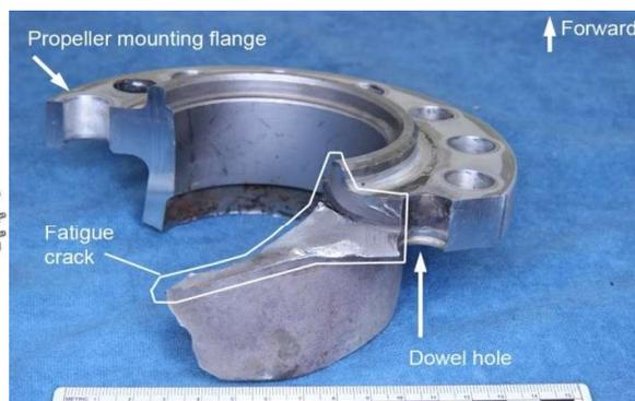
Figure 4 Section of propeller shaft
