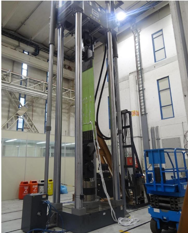
Figure 7 – E-190 E2 wing lower skin panel crack propagation tests.
