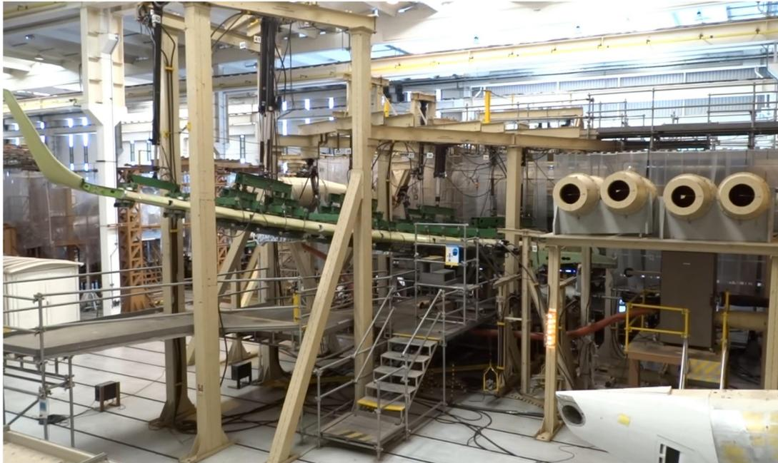
Figure 6 – Overview of the residual strength Test – ERJ-190.
