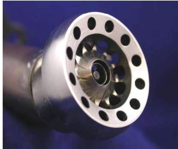
Figure 96 Laser clad repaired fuel nozzle swirler after final machining
