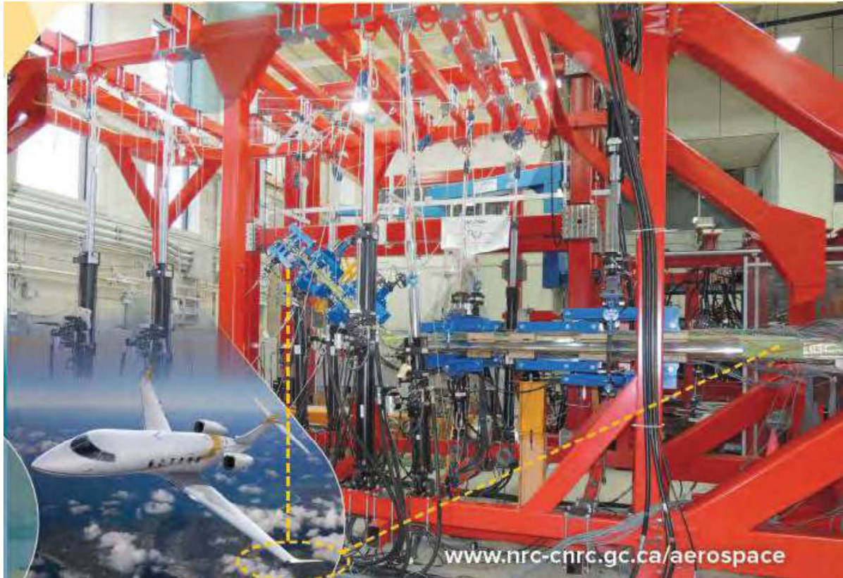
Figure 9 Winglet certification test setup for the Challenger 350
