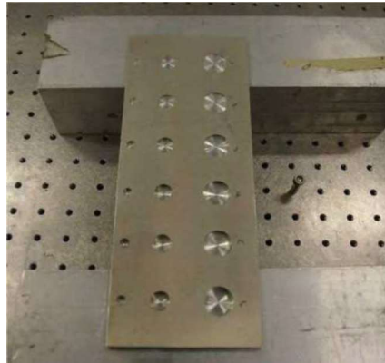
Figure 64 Aluminium plate (7075-T6) used in the experiments
