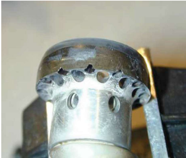
Figure 95 Damaged fuel nozzle swirler
