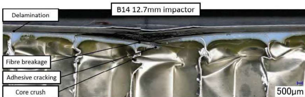
Figure 42 Multi-mode panel damage using a 12.7mm radius impactor
