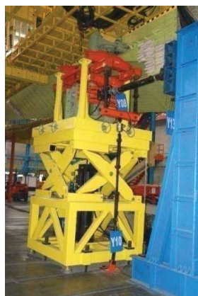
Figure 4. 27 Tracking Loading and Sustain Installation on Landing Gear
