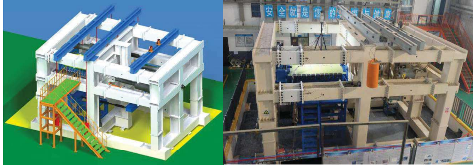
Figure 4. 36 Static/Fatigue Test Device of the Large-Scale Fuselage Panel Under Complex Loads
