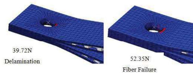
Figure 3.31 Progressive Damage Process of Joint Hole
