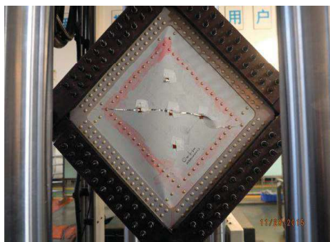
Figure 3. 5 Fatigue Buckling Failure of Structure
