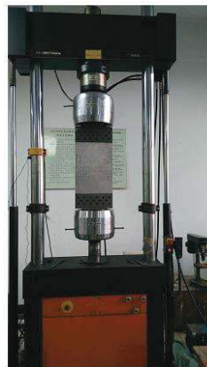
Figure 3.45 Multiple-Site Damage in Riveted Lap-Joints Experiment
