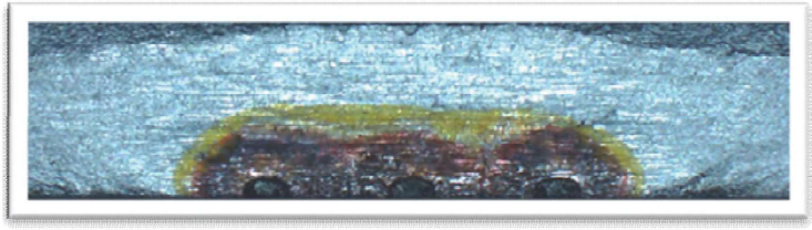
Figure 3: 3 coplanar crack sites configuration – confrontation FEM model/multiple cracks propagation fatigue test
