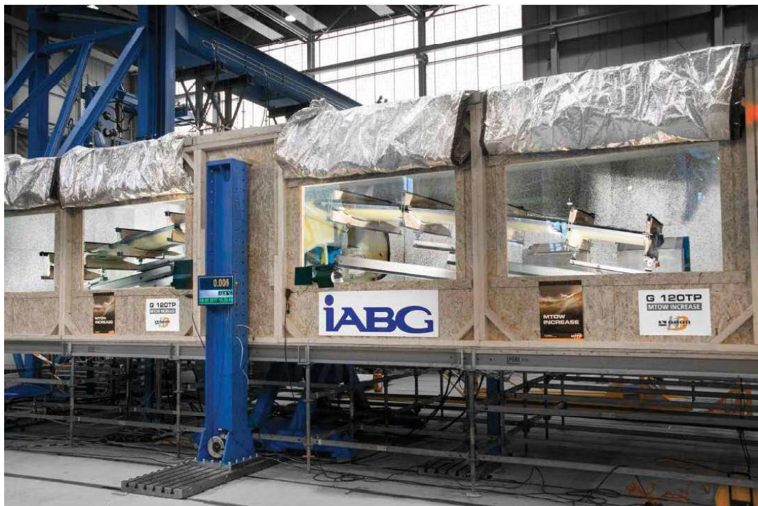
Figure 12: Test Set-up including thermal chamber at iABG
