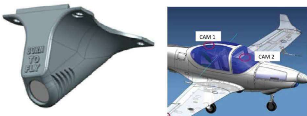
Figure 27: Camera Mount Canopy (cam 1) and mounting position
