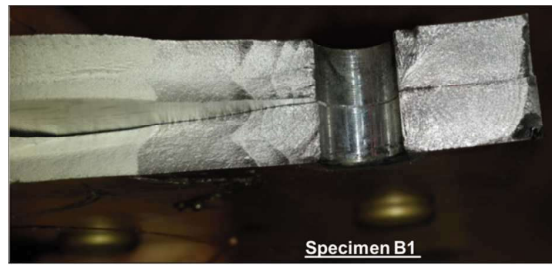
Figure 19. Specimen having transition-fit installed fasteners by hand plastic hammering test results
