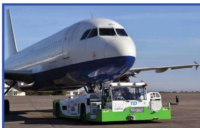
Figure 52. TaxiBot NB prototype towing the Airbus A320-200
