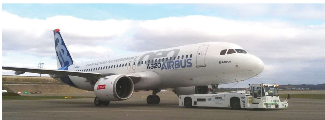
Figure 54. TaxiBot NB, with A320neo during the certification test at Airbus Toulouse December 8, 2016
