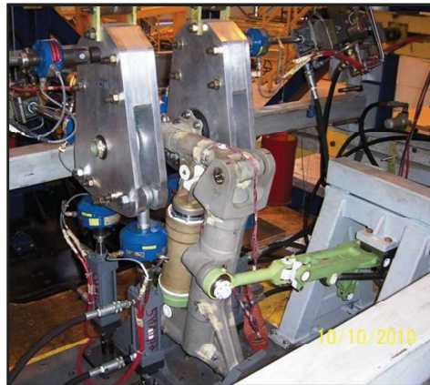
Figure 10. Main Landing Gear Fatigue Testing
