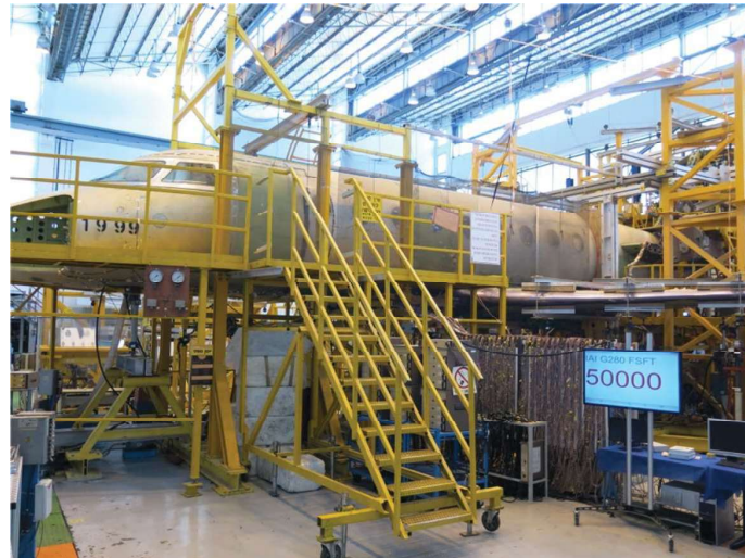
Figure 1. Complete Airframe Mounted in its Fixture upon completion of two and a half lifetimes (50,000 flights)
