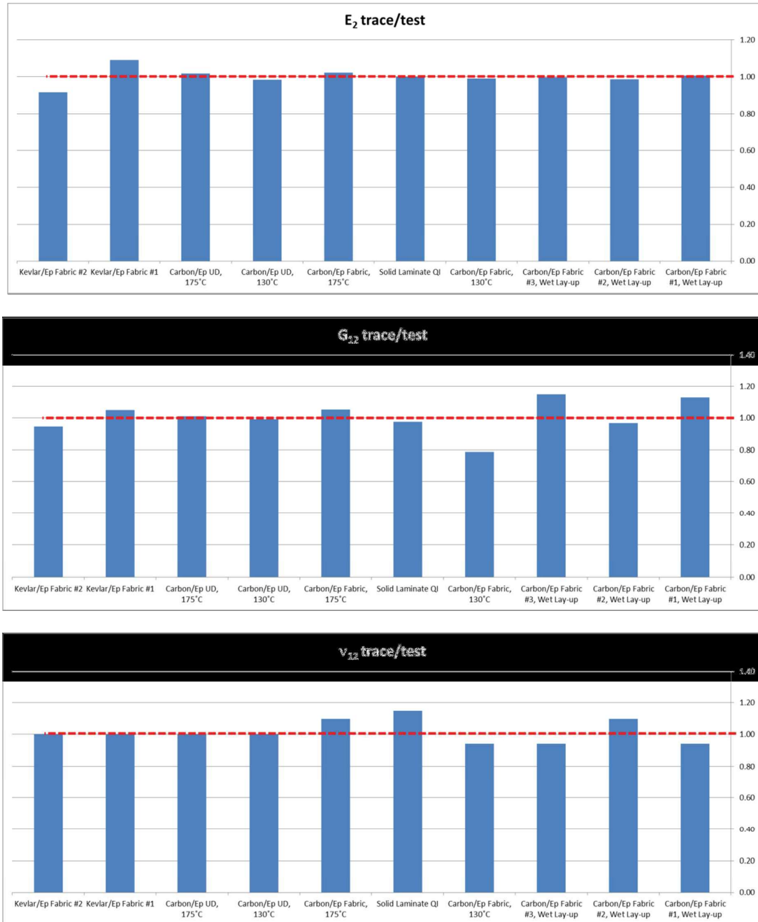
Figure 29. Predictions of transverse Young's modulus versus test results for different Carbon and Kevlar based composites.
