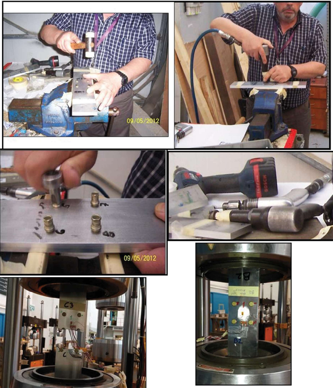
Figure 18. Specimen fasteners installation procedure, tooling and testing via the tensile machine
