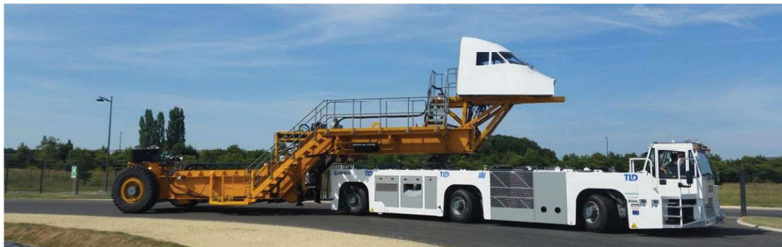
Figure 55. TaxiBot WB, with its testing trailer during maneuvering test
