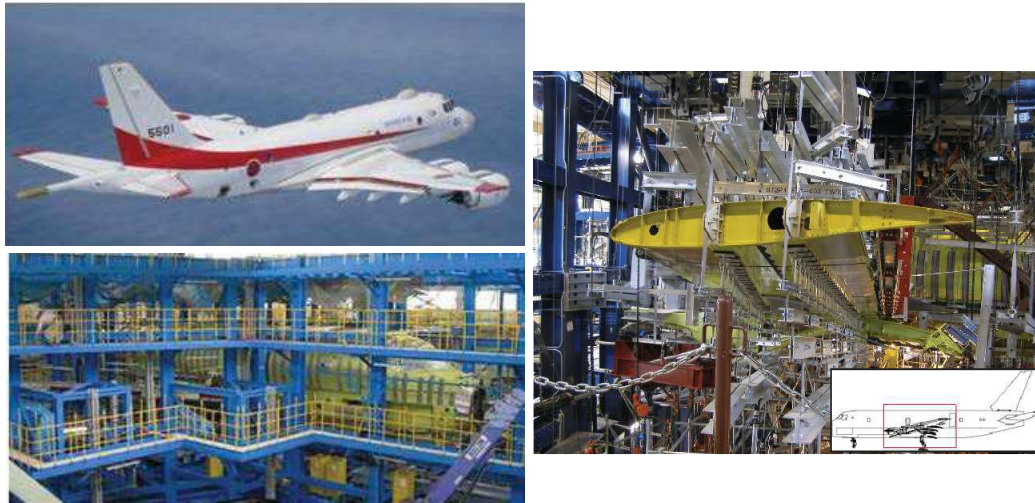
Figure 44 Test fixtures of XP-1 full-scale static test (top left: XP-1 aircraft, bottom left: overview of test rig, right: test fixture of L/H wing)
