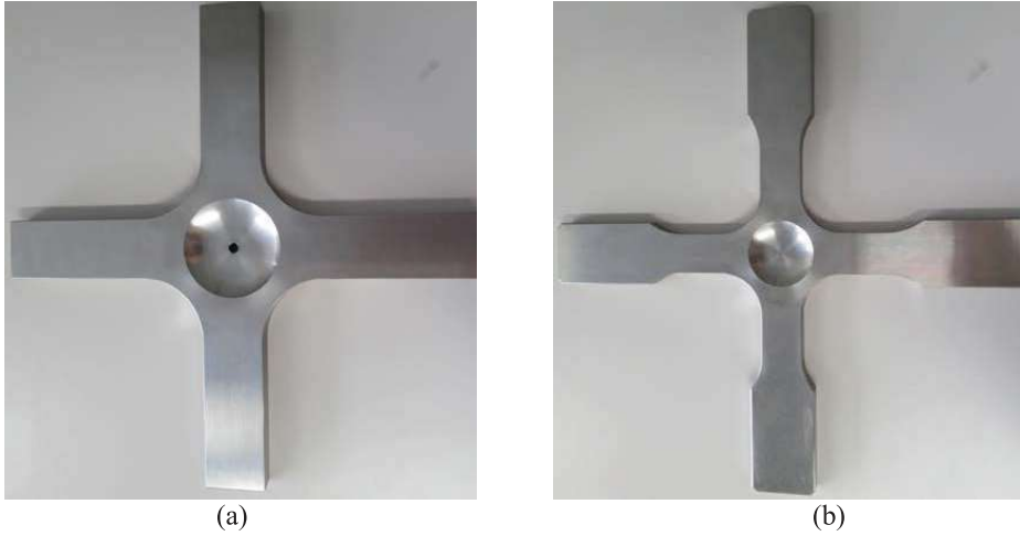
Figure 8 (a) Geometries of hole notch cruciform specimen and (b) smooth cruciform specimen.
