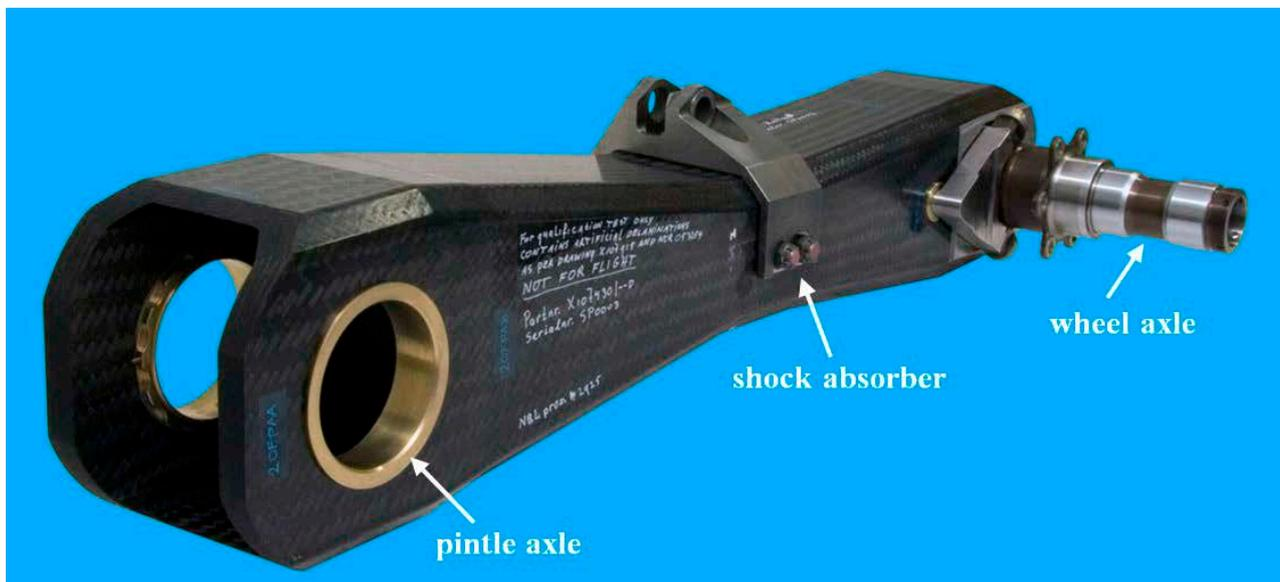
Figure 32: The RTM trailing arm of Fokker Landing Gear that was used as a calibration specimen in the investigation.
