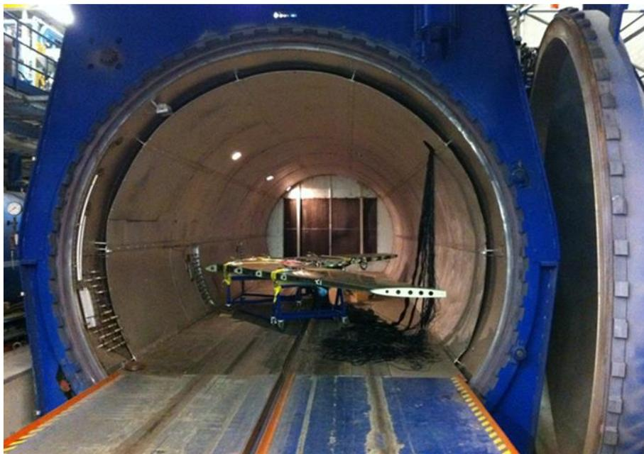
*Thermal test of a horizontal stabilizer in an autoclave at Fokker*
