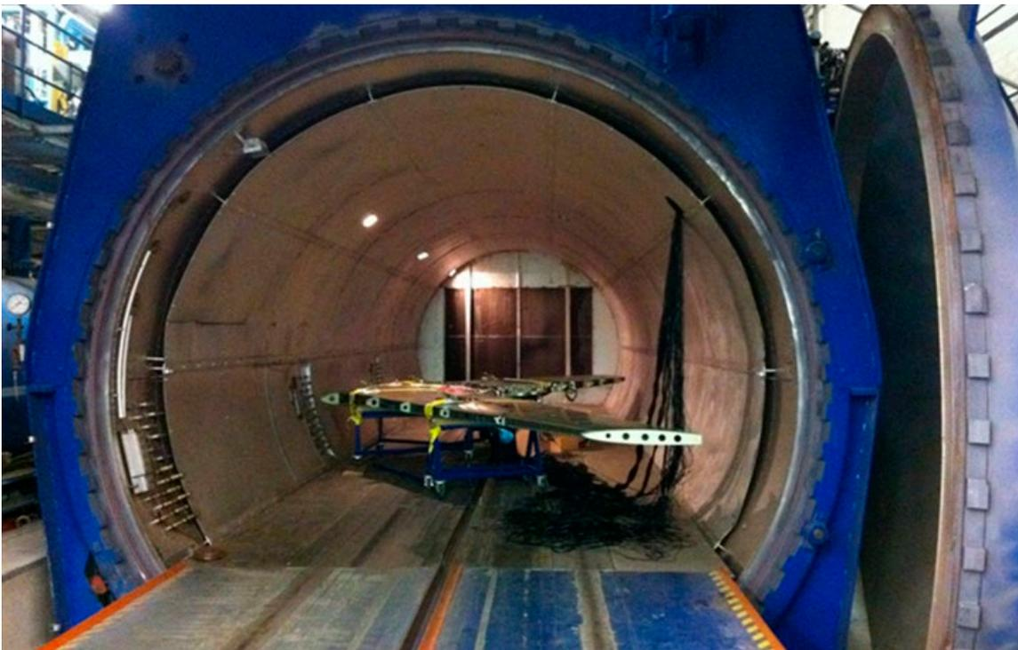
Figure 26: Thermal test on the instrumented horizontal stabilizer static and FDT component test article in an autoclave at Fokker.
