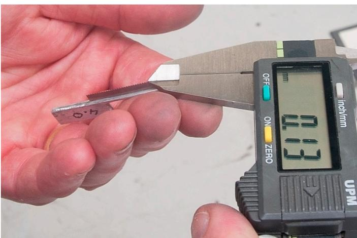
Figure 46: Sawblade thickness.
