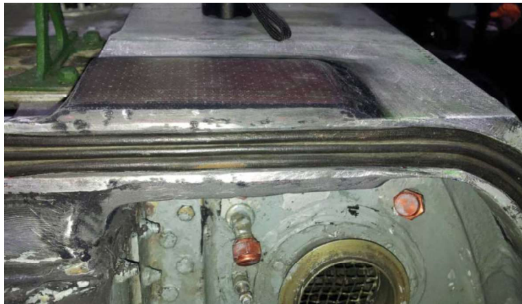
Figure 20. Structure after repair, sealing hose installed
