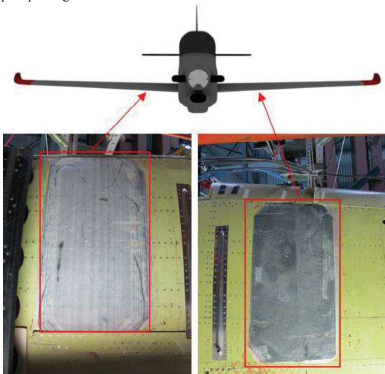
Figure 21. Location of the composite repair patches on the aircraft wing
