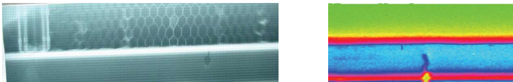
Figure 23. X-Ray (left) and eddy current (right) inspection results of the crack in the main spar
