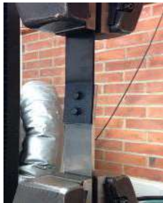
Figure 3.2-9. Test setup for single-shear test
