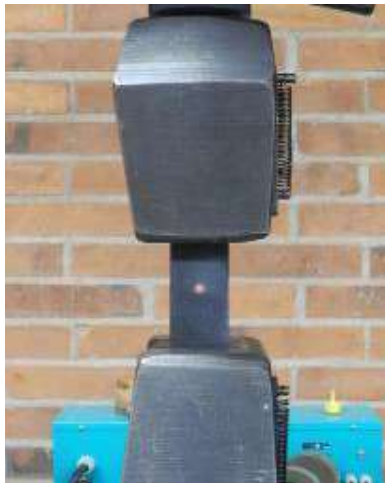
Figure 3.2-6. Test setup for open-hole tensile tests
