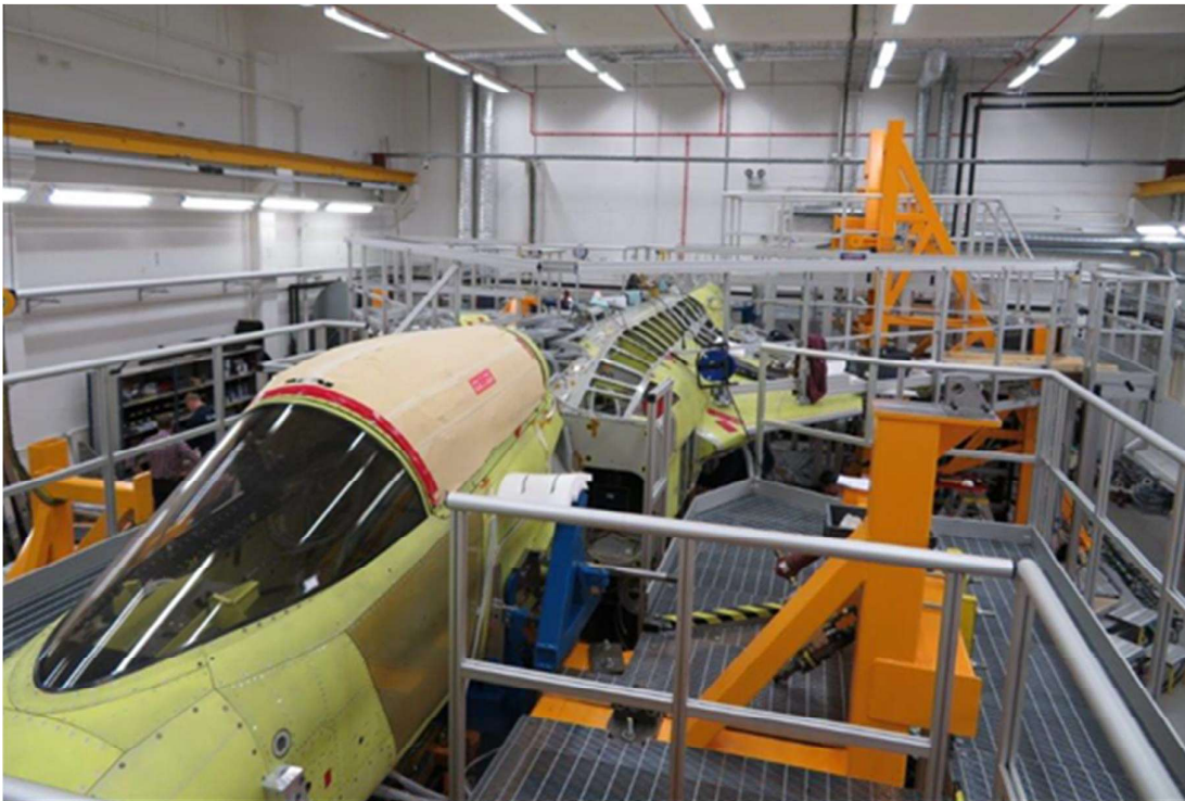
Figure 2.2-4. Static test during assembly of airframe in test rig, top view
