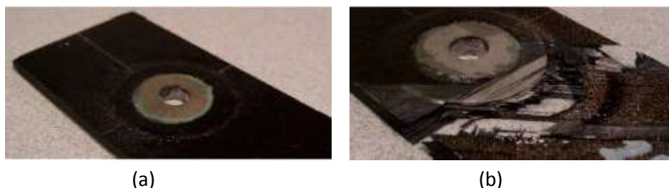
Figure 3.2-5. Bearing failure of the good (a) and premature failure of the poor (b) configurations
