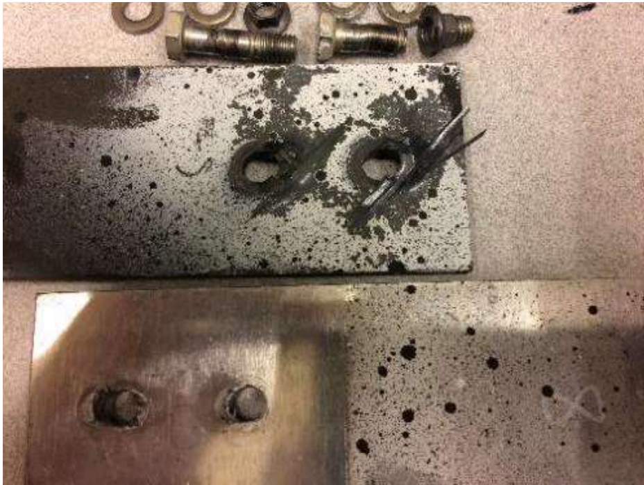
Figure 3.1-7. Broken test specimen.
