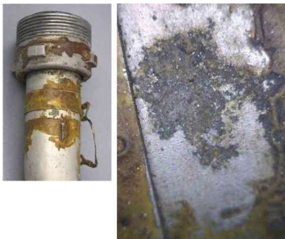
Figure 1: Example electrical bonding related corrosion
