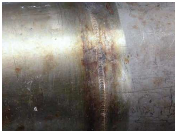
Figure 1: Example hot-air duct corrosion
