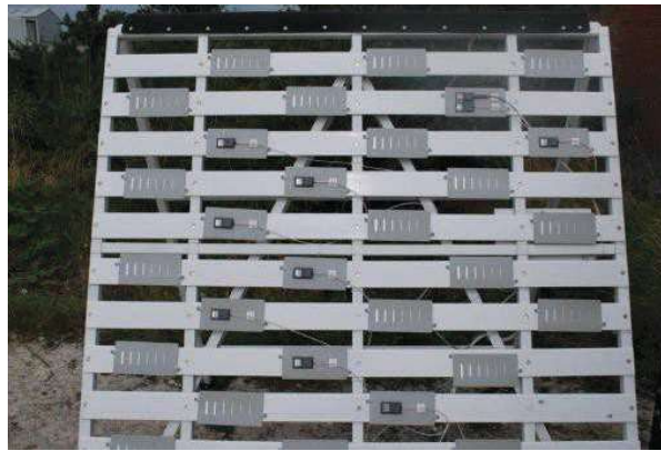
Figure 2: PCD testing alongside bulk material witness plates
