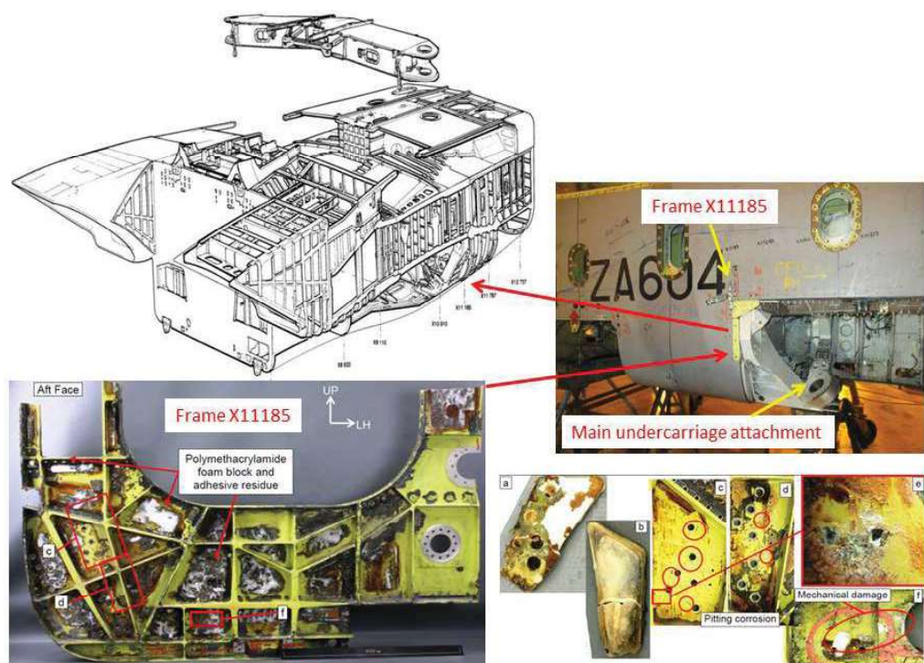
Figure 1: LH Frame X11185 and (a, b) PMA foam block (c - e) corrosion (f) mechanical damage
