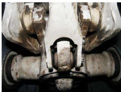
Figure 1: Example undercarriage surface finish damage
