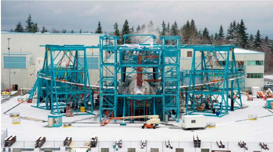
**Figure 9.11-77. 787 Full-Scale Fatigue Test Setup**
