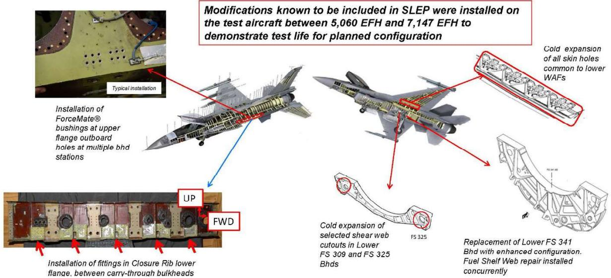
**Figure 9.4-11. Installed SLEP Modification**
