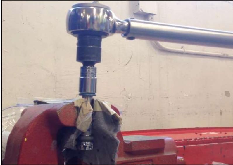
**Figure 9.6-55. Torque Test Setup Example**
