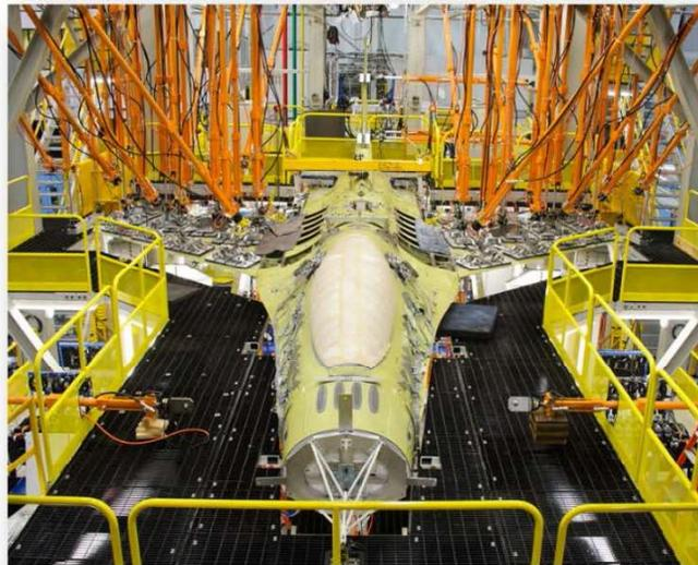
**Figure 9.4-10. F-16 Full-Scale Durability Test Aircraft**
