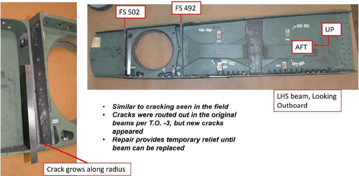
Figure 9.4-14. Horizontal Tail Outboard Support Beam Cracking
