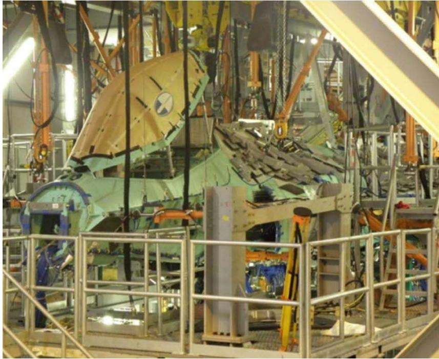
**165 Load Rams, 1849 Strain Gage Channels
