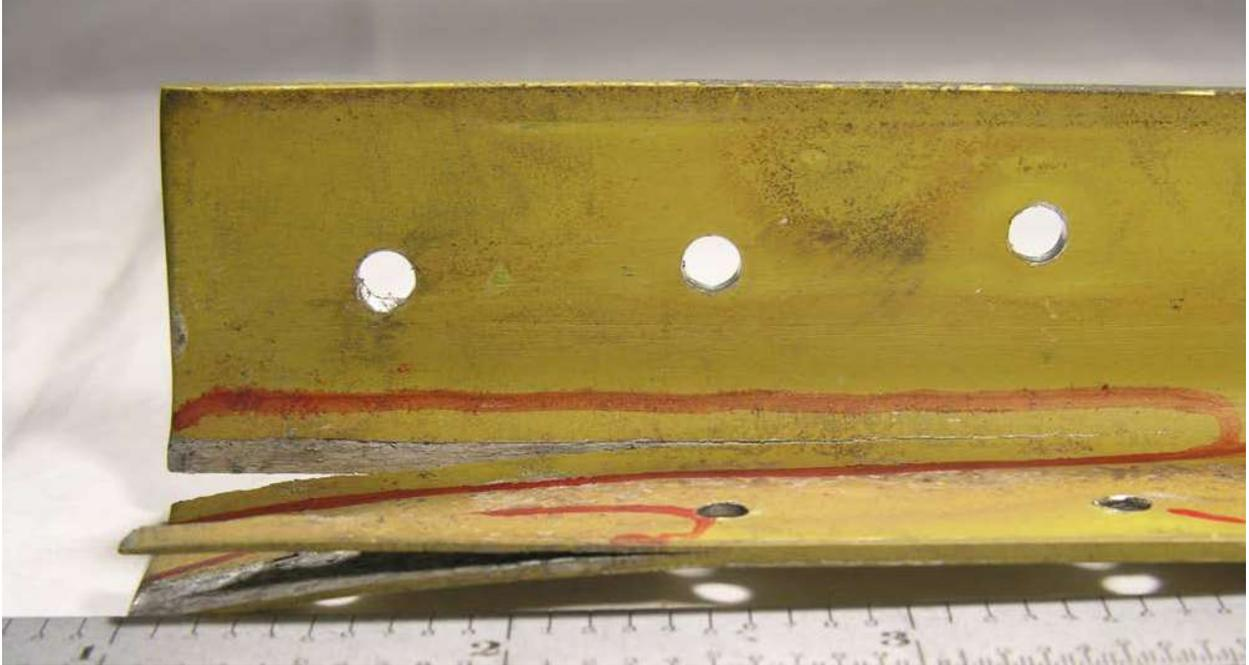
**Figure 9.11-89. Stiffening Element Exhibiting In-Plane Cracks**
