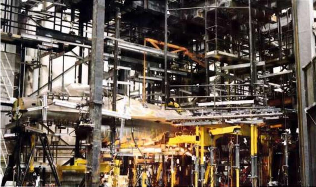
**Figure 9.11-38. F-16A Full-Scale Fatigue Test**
