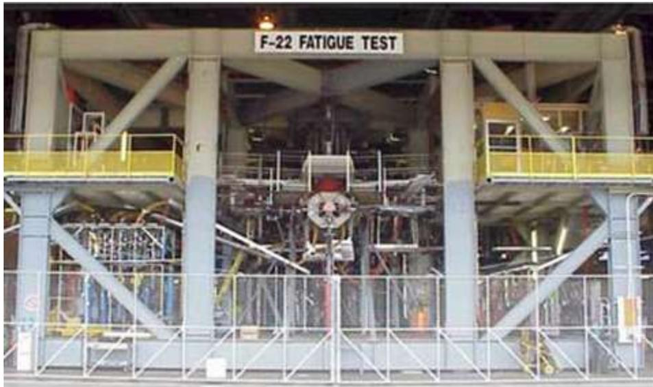
**Figure 9.11-39. F-22 Full-Scale Fatigue Test**
