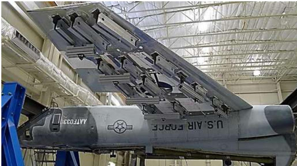
**Figure 9.11-52. Whiffletree Design**
