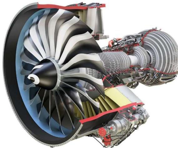
**Figure 9.6-87. CFM LEAP Turbofan Engine Used on Boeing 737MAX and Airbus A320neo Aircraft**
