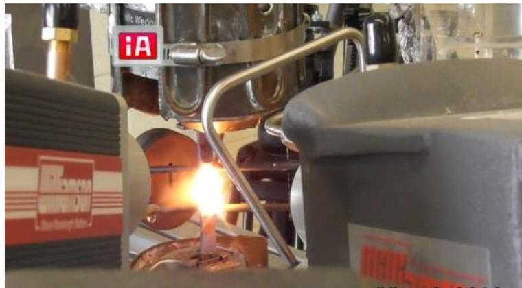
**Figure 9.6-74. An EBC-Coated SiC/SiC Specimen Under High Heat Flux Fatigue Testing in Steam and CMAS Exposure Conditions**
