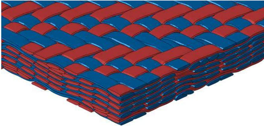
**Figure 9.6-83. Graphical Representation of Three-Dimensional Woven Fiber Architecture Used in the Fatigue Evaluation**
