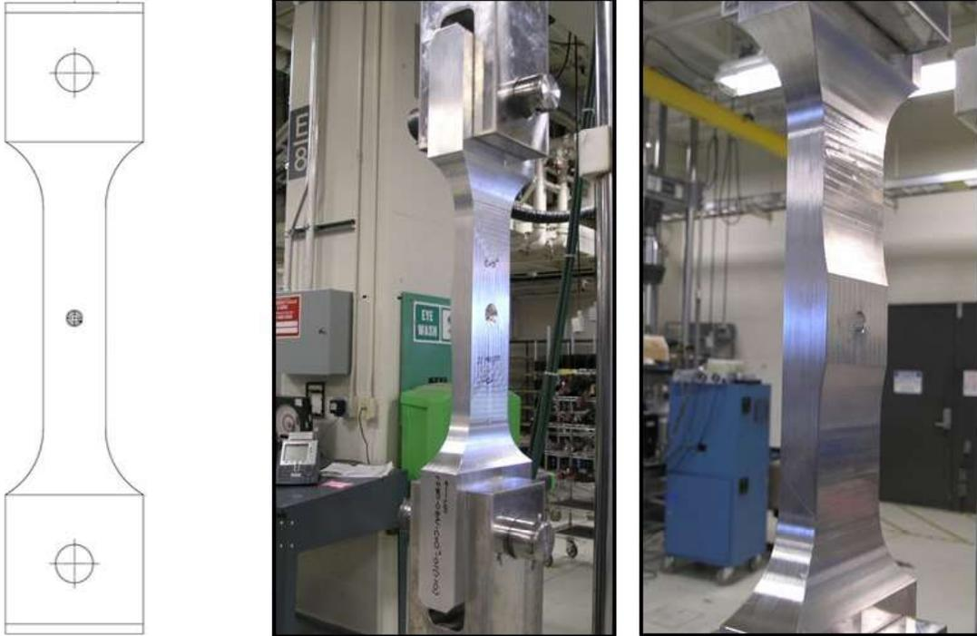
Figure 9.8-41. Phase I Coupon Design
