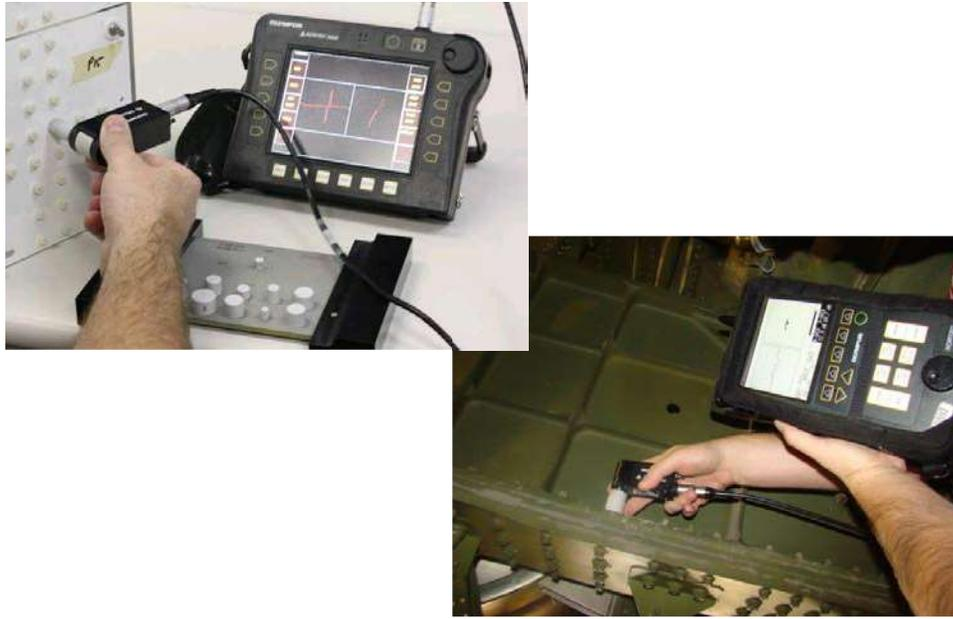
Figure 9.3-2. Manual ET Inspection for Fatigue Cracks
