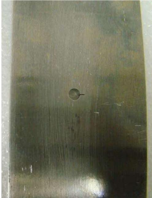
Coupon with hole & EDM notch
