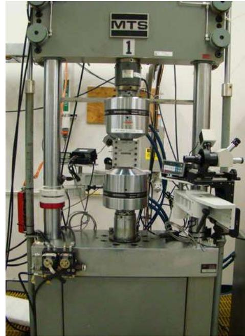
Typical Coupon Crack Growth Test
