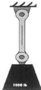
**Figure 9.11-81. Single Load Path Structure**
