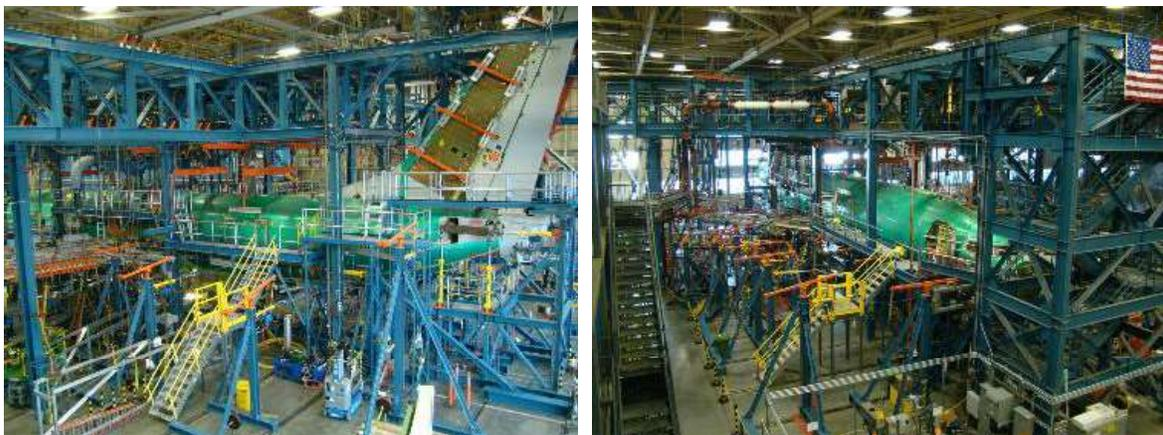
Figure 9.11-76. P-8A Fatigue Test Set-Up
