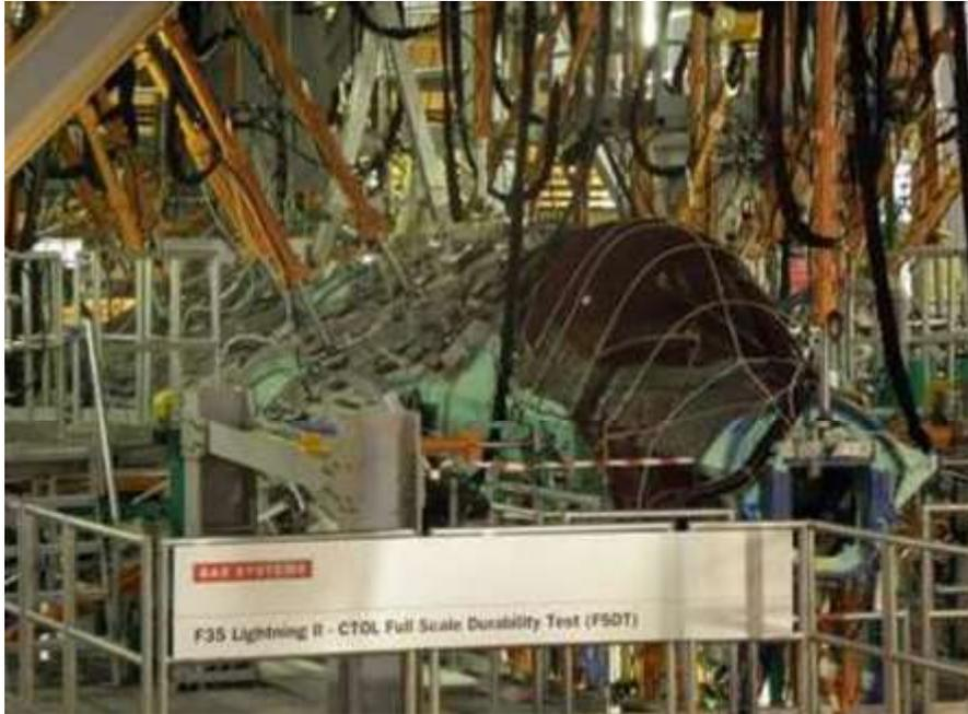
**Figure 9.11-40. F-35A (CTOL) Full-Scale Fatigue Test**
