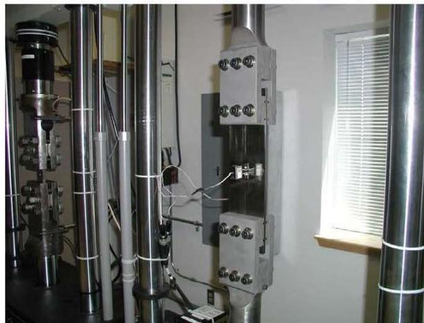
Figure 9.6-15. FCGR Test Specimen
