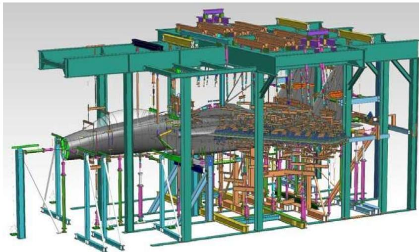
**Figure 9.11-69. F-15 Full-Scale Fatigue Test Setup**
