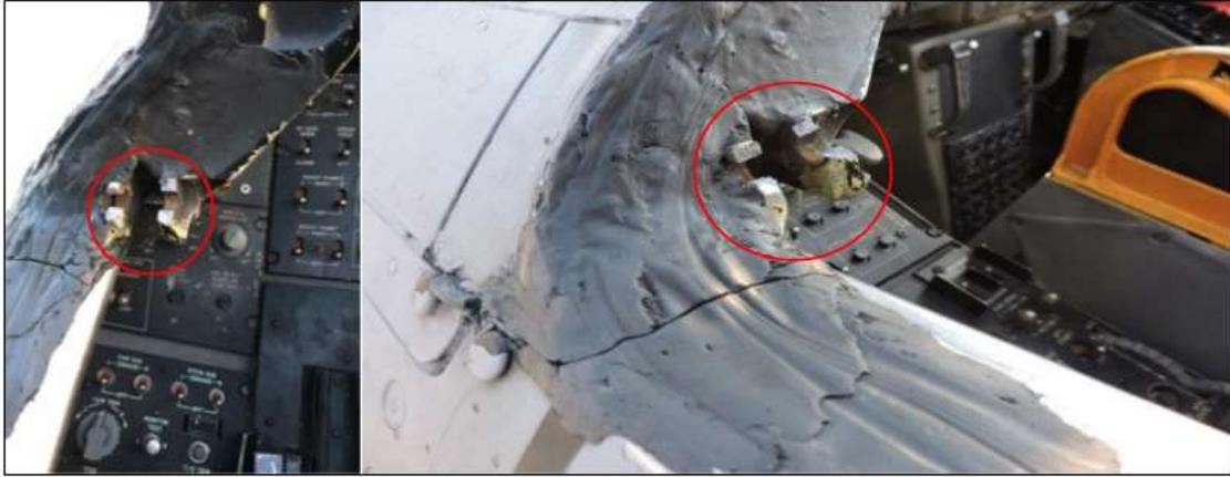
Figure 9.2-19. Failure Origin
