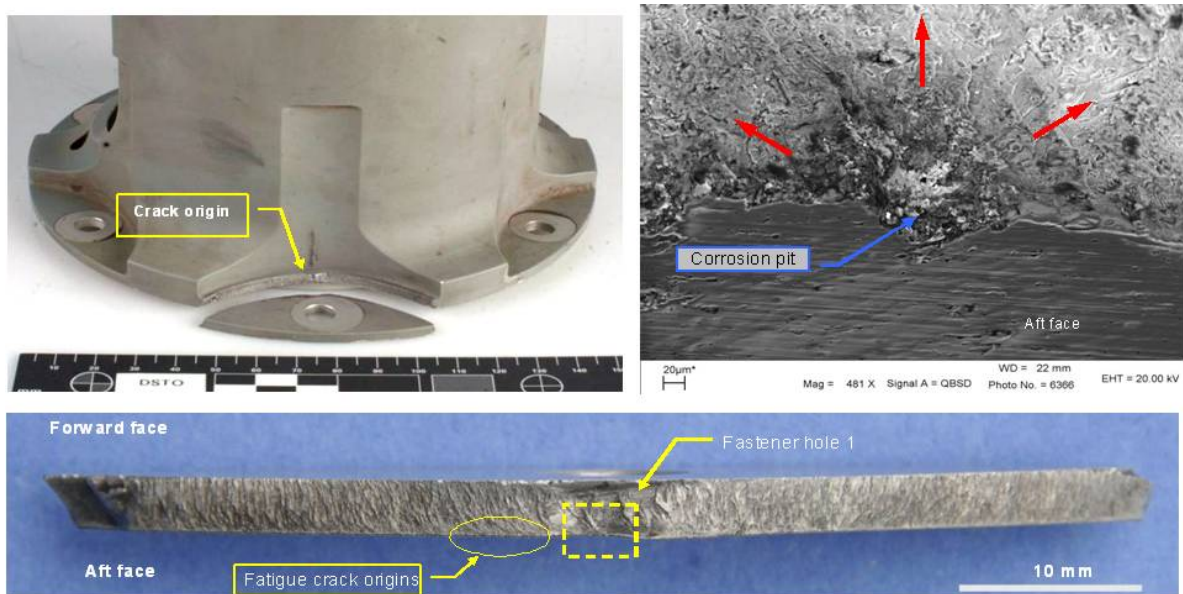
Figure 22 Black hawk high speed shaft tube cracking.
