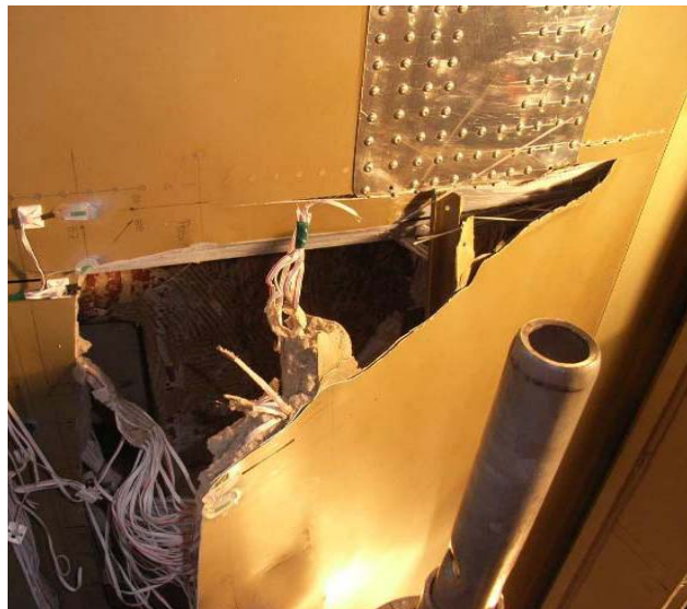
Figure 3.14 Flap after residual strength testing
