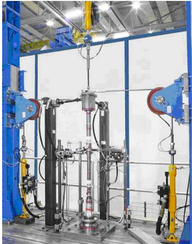
Figure 2.10 MTA with the non-rotating LP shaft and hydraulic actuators
