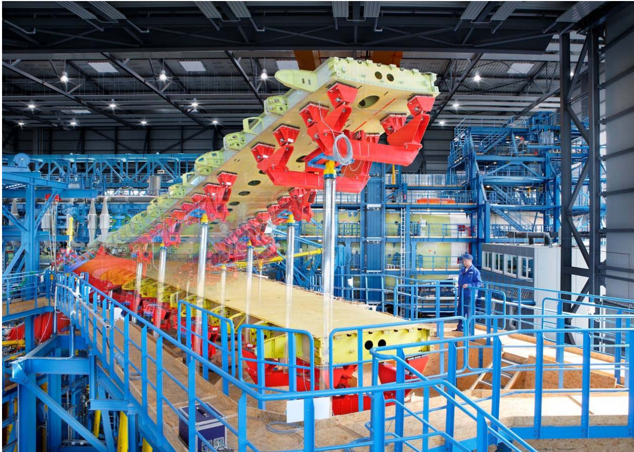
Figure 2.1 Double-shot view of the A380EF wing deflection during fatigue cycling
