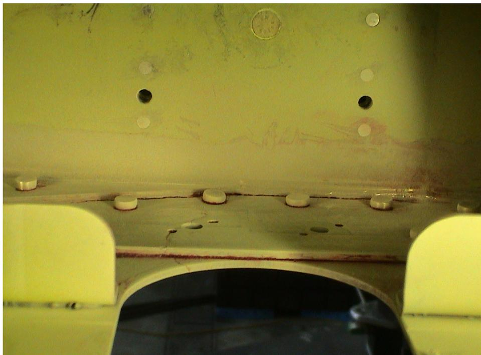
**Fig. 47 - M-346 LH Prototype Wing development fatigue test – crack on the spar cap carrying the flap attachments**
