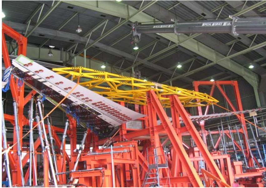
**Fig. 49 – B. 787 Horizontal Tail test rig.**
