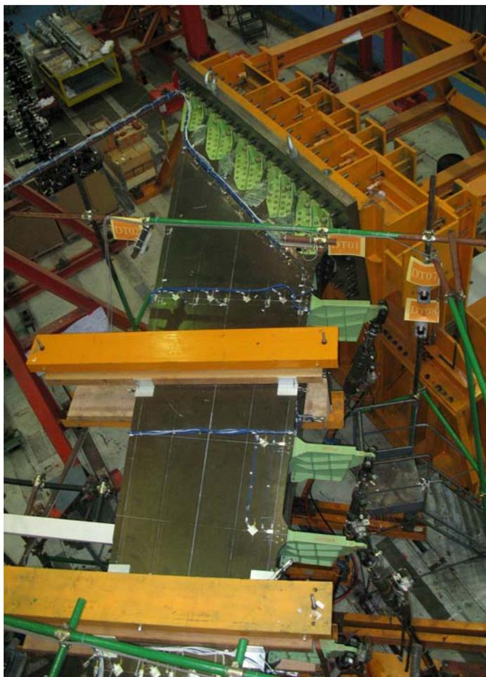
**Fig. 48 - Detail of B.787 Horizontal Tail composite structure in the fatigue test. (Half structure was tested).**
