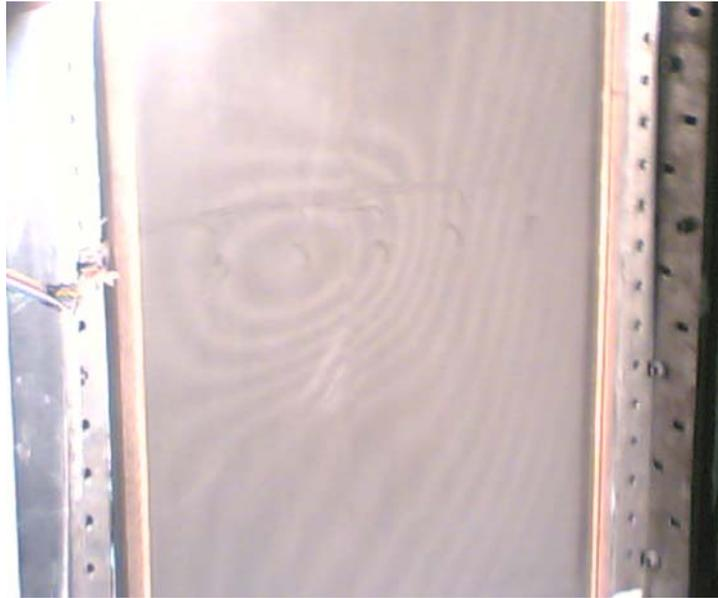
Fig. 38 - Out-of-plane deformation of defective composite stiffened panel under uniaxial compression.
