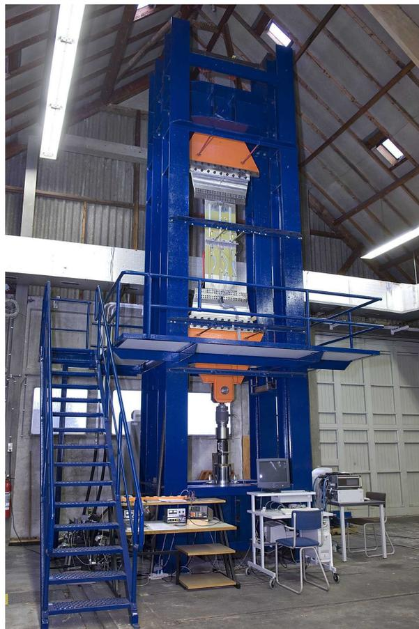
*Fig. 19 GLARE stringer coupling panel during testing at the NLR*
