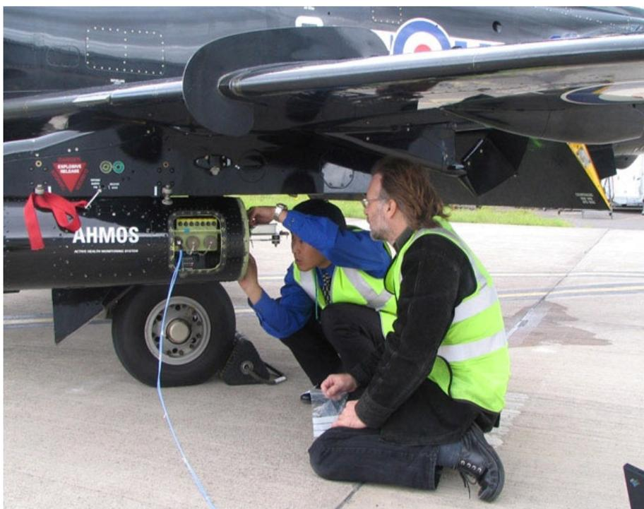
Fig. 9 AHMOS key system components installed in a pod on a Hawk aircraft for flight testing in the UK
