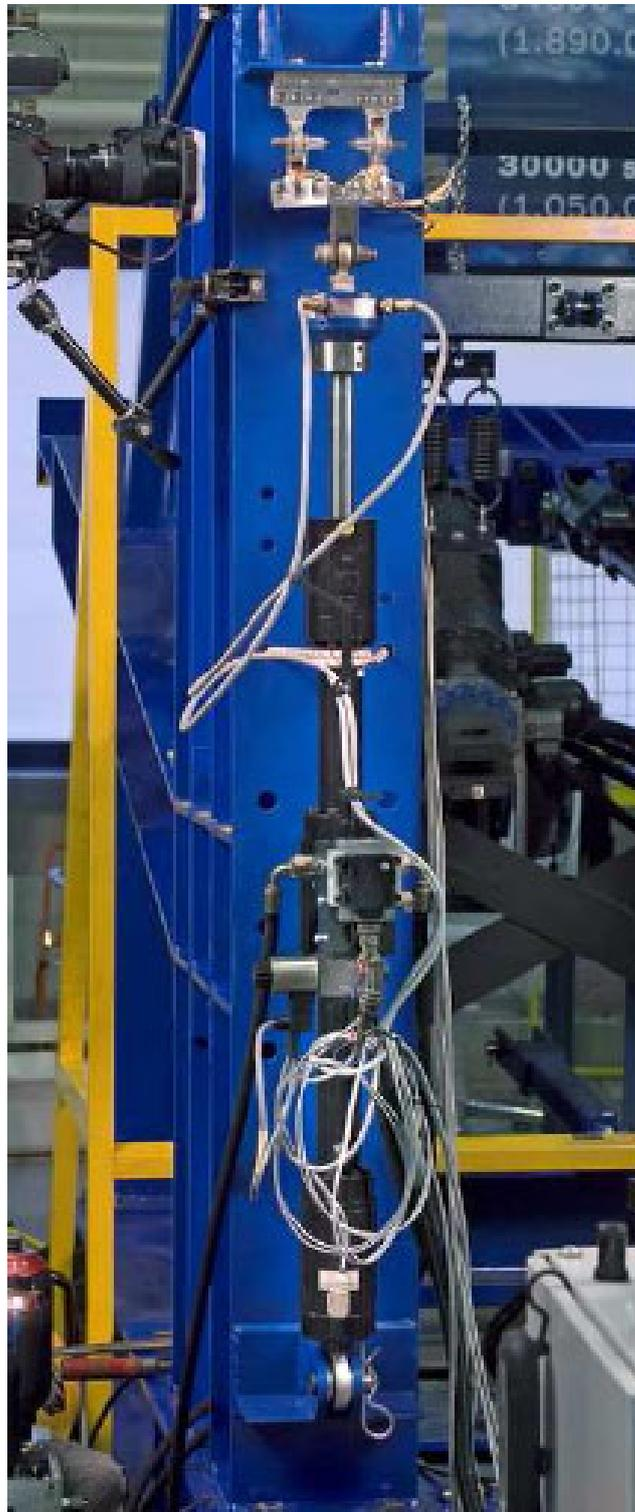
*Fig. 30 ATV panel hinge specimen (at top of picture) in the ad hoc test rig*
