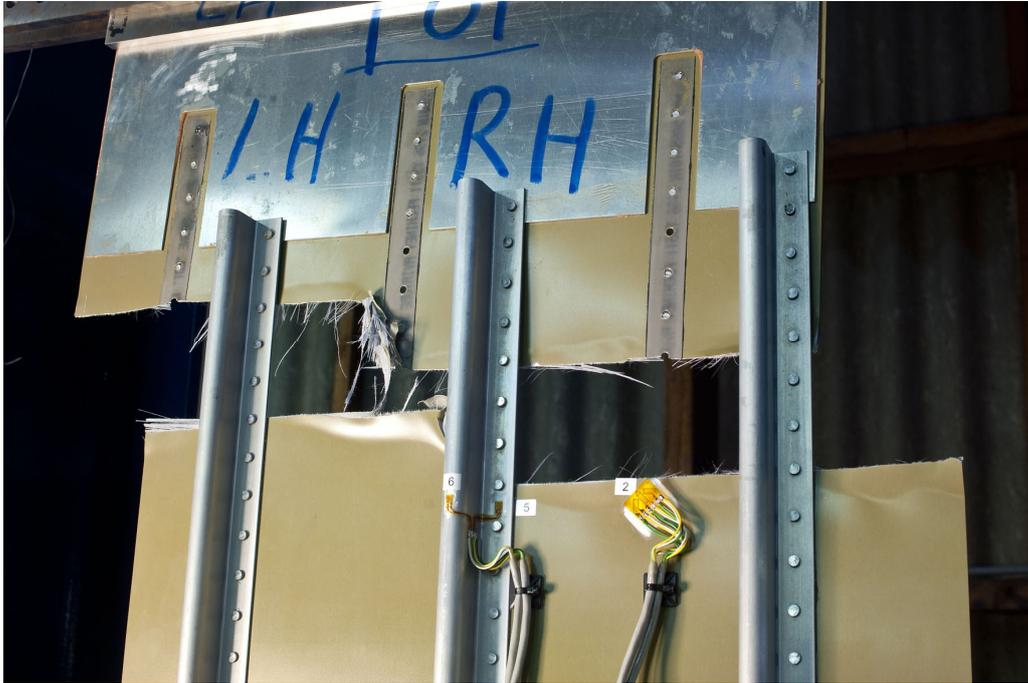
Fig. 20 Failure of the GLARE stringer coupling panel in the stringer runout area
