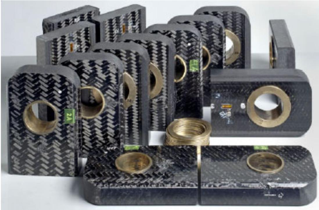
*Fig. 39 Composite lug details for proof of concept evaluation of a generic composite brace*
