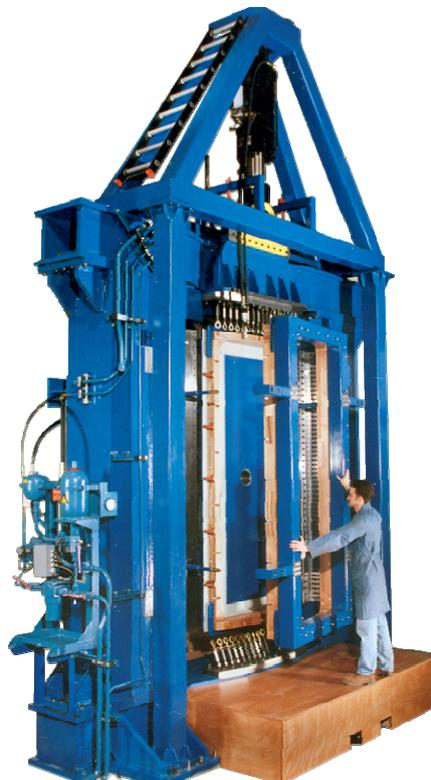
Fig. 17 The NLR fuselage panel test rig
