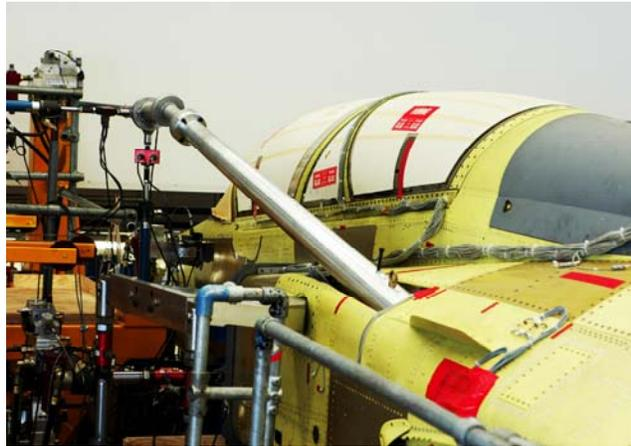
Figure 22. Gripen twin-seater 39D. Schematic drawing and a photograph of the of the forward fuselage with the air-to-air refuelling probe dummy.
