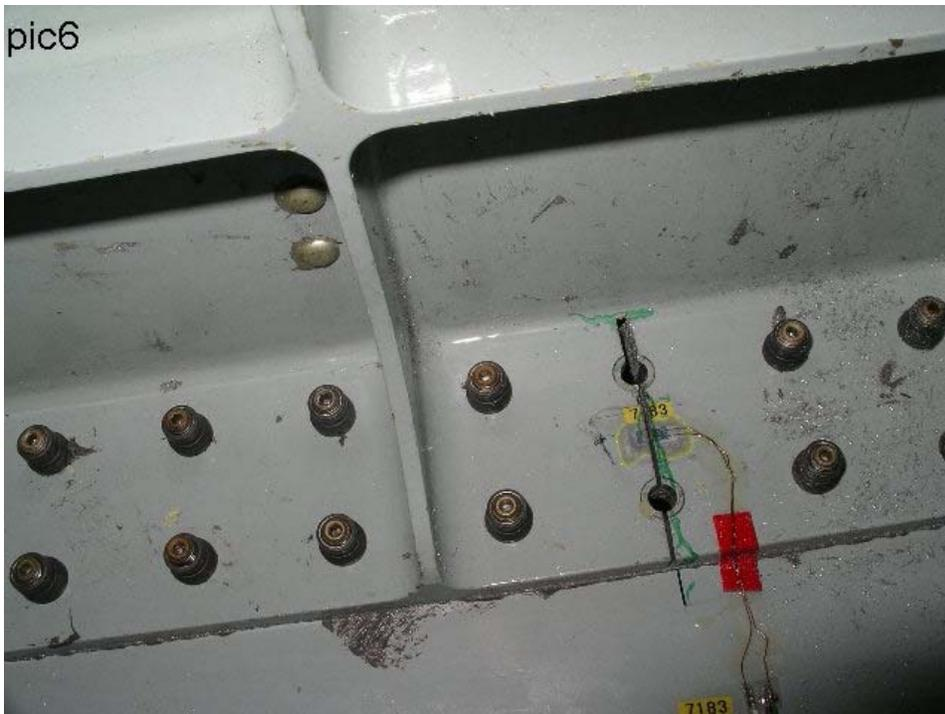
Figure 16. Saab 2000 Artificial crack in lower forward wing spar cap and in skin
