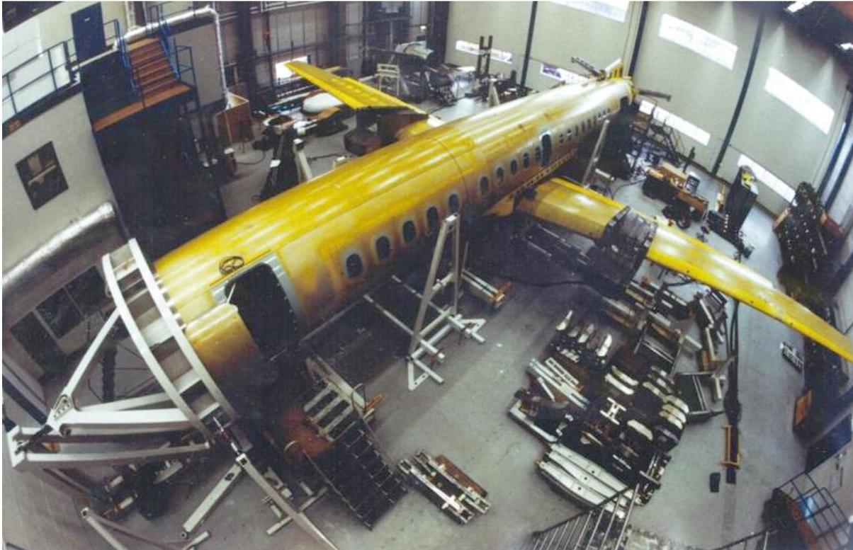
*Figure 14. Saab 2000, wing/fuselage fatigue test.*
