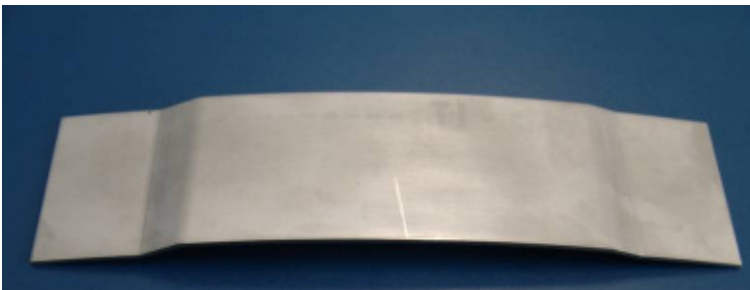
Figure 4.7.13: Feasibility of manufacturing the titanium strap for door #44
