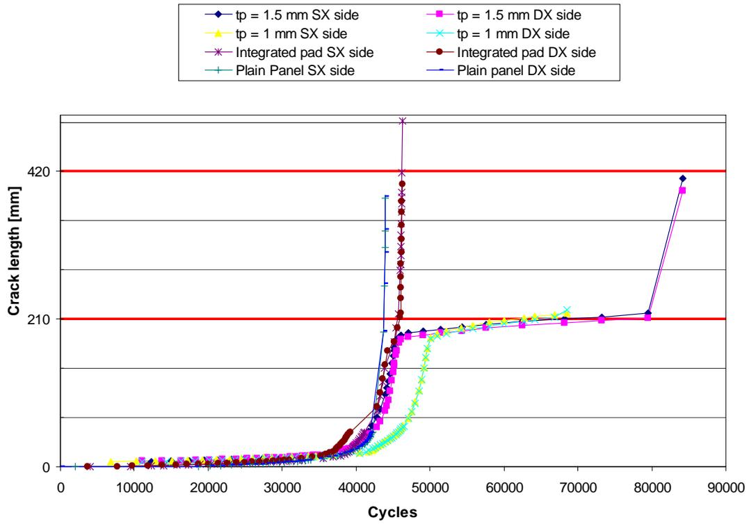
Fig. 23 - Comparison of various crack growth curves obtained.
