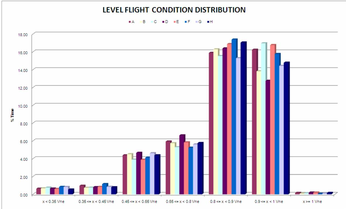
**Fig. 7 - Distribution of level flight speed in the monitored machines of the Danish AW101 fleet.**
