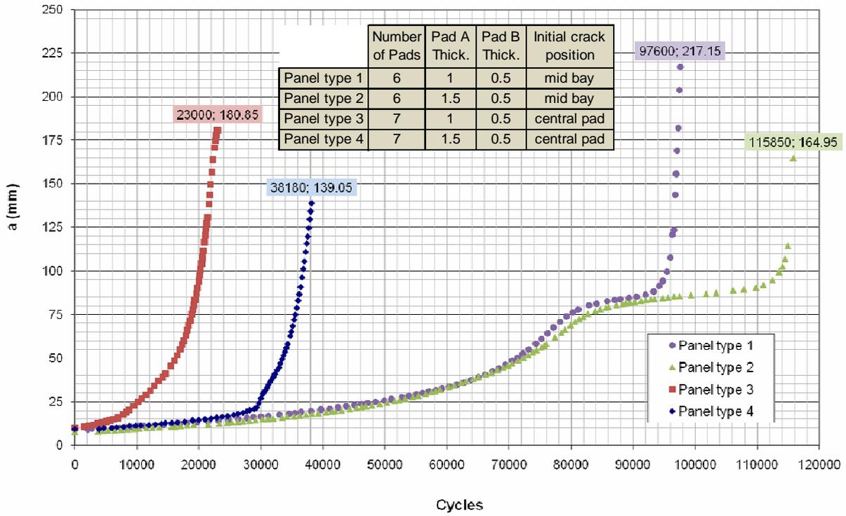
Fig. 19 – Summary of crack propagation results: a vs N curves
