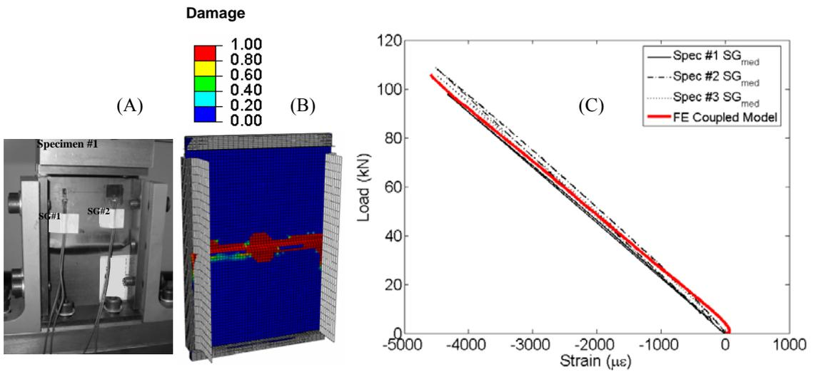
Fig. 30 – Compression after impact test: (A) experimental evidences, (B) final failure mode in the FE Coupled Model and (C) numerical-experimental correlation of the load vs. strain response
