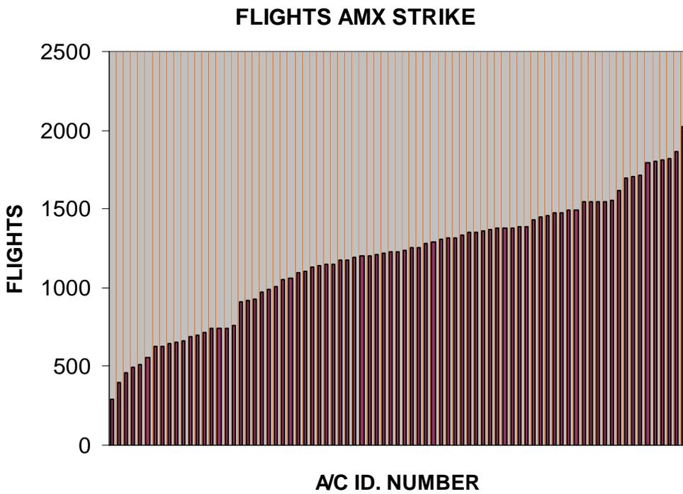
Fig. 2 – Distribution of Flight Hours in the AM-X Strike fleet
