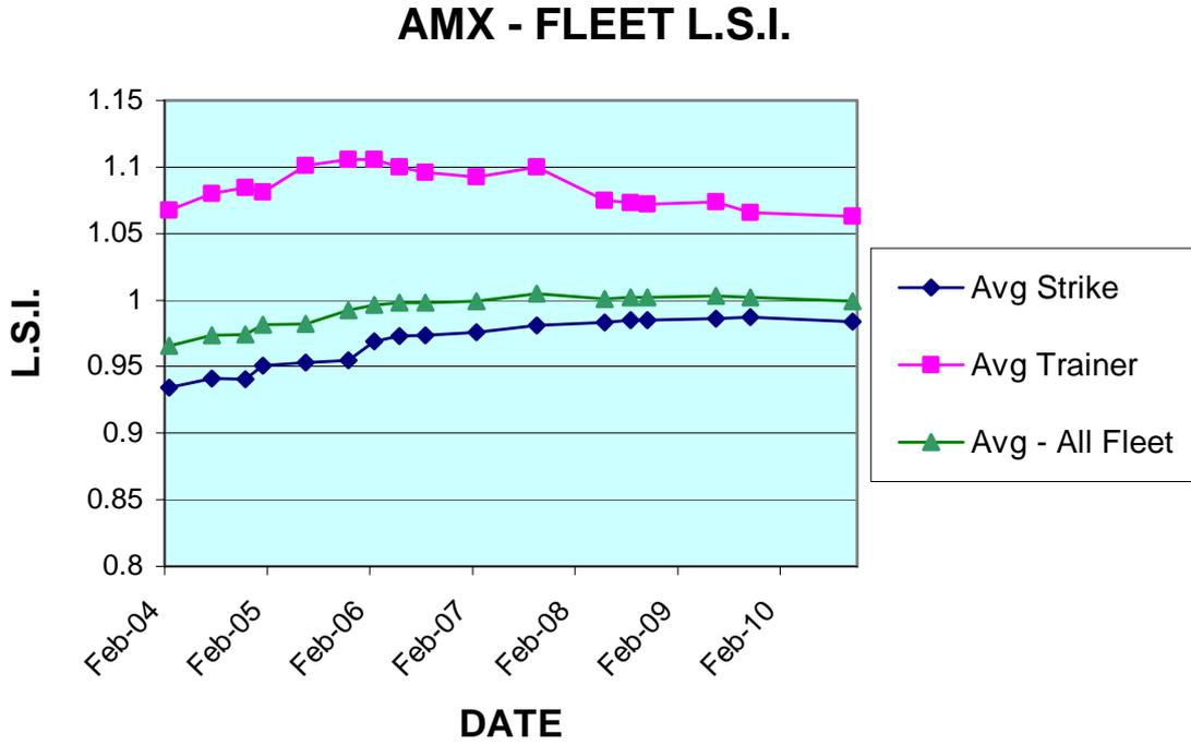
Fig. 1 – Load Severity Index distribution for the AM-X fleet.
