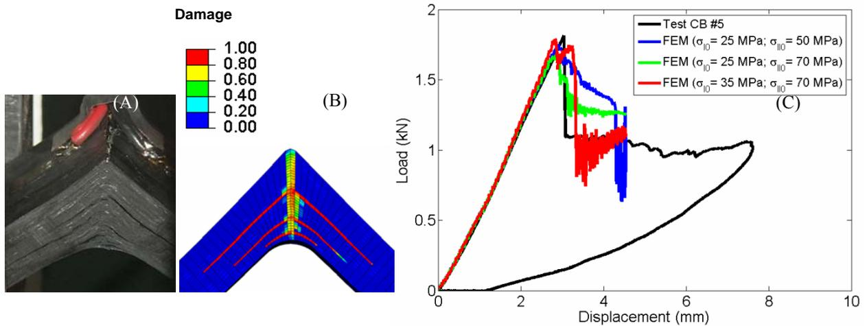
Fig. 28 – Four point bending test on curved laminate: (A) experimental evidences, (B) interlaminar damage in the numerical model and (C) load vs. displacement numerical-experimental correlation
