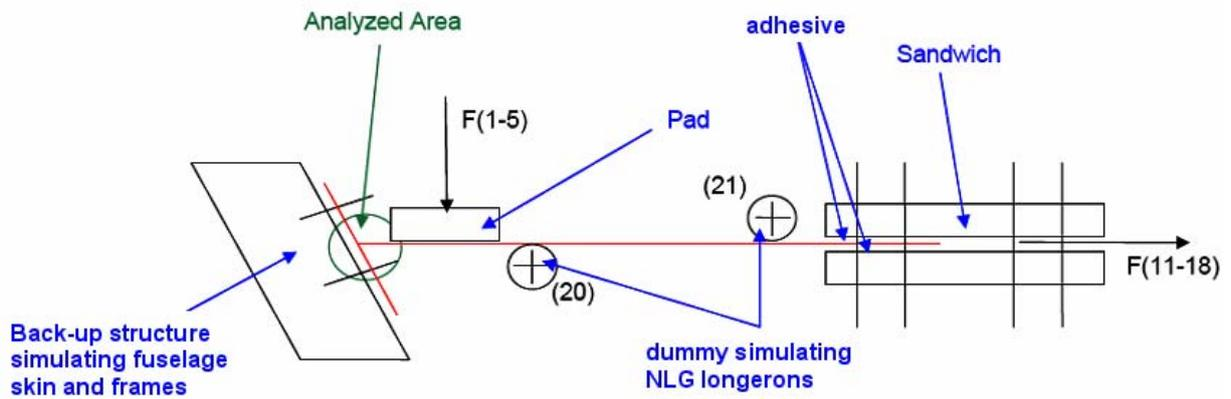
Fig. 33 - Sketch of the set-up for the M346 CFRP cabin floor to fuselage joint fatigue test.
