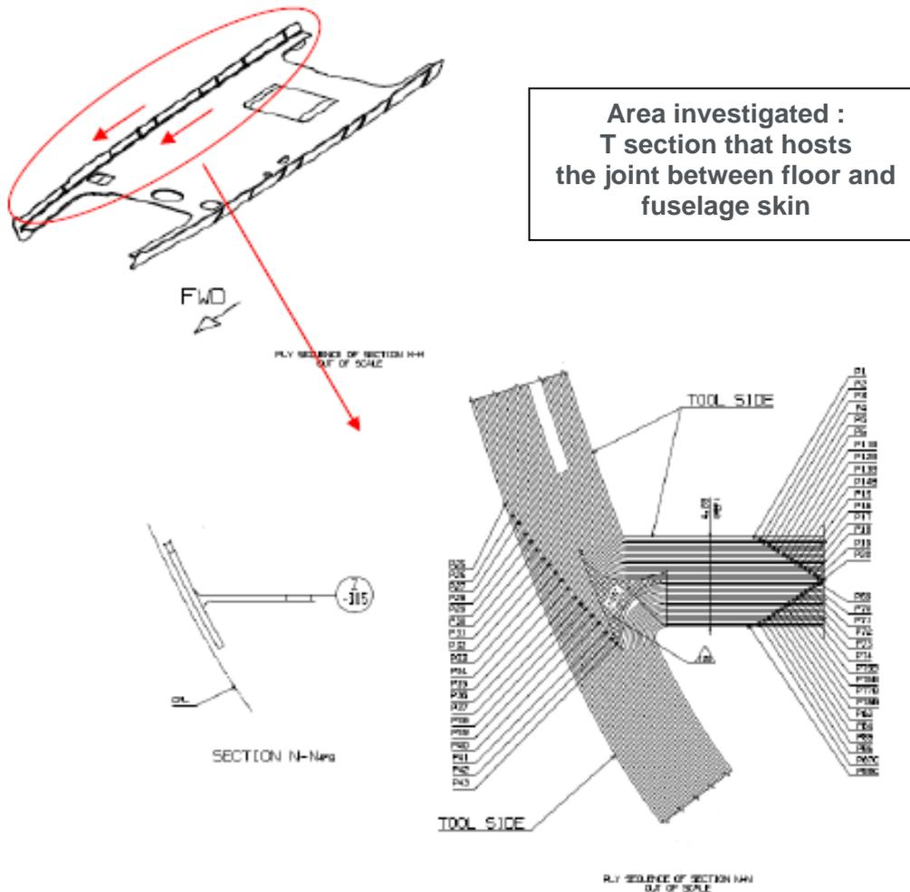
Fig. 32 - M346 CFRP cabin floor to fuselage joint.
