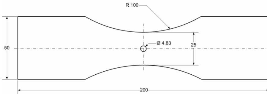
Fig. 14 - Open hole specimen in thin sheet (Laser Shock Peening)
