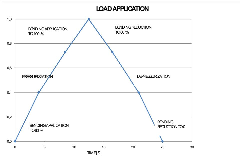
Fig. 27 - Sequence of combined load application in the barrel test.
