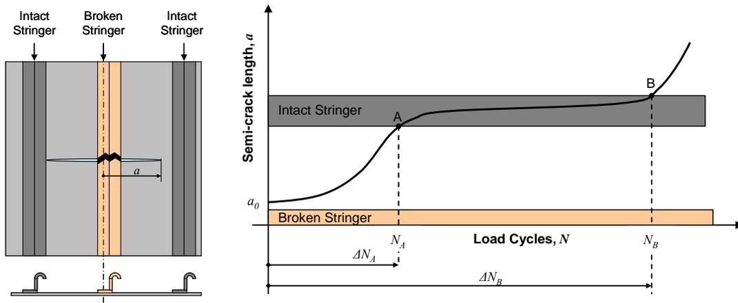
**Fig. 21 - Fatigue Crack Propagation (FCP) through bonded stiffened panels.**
