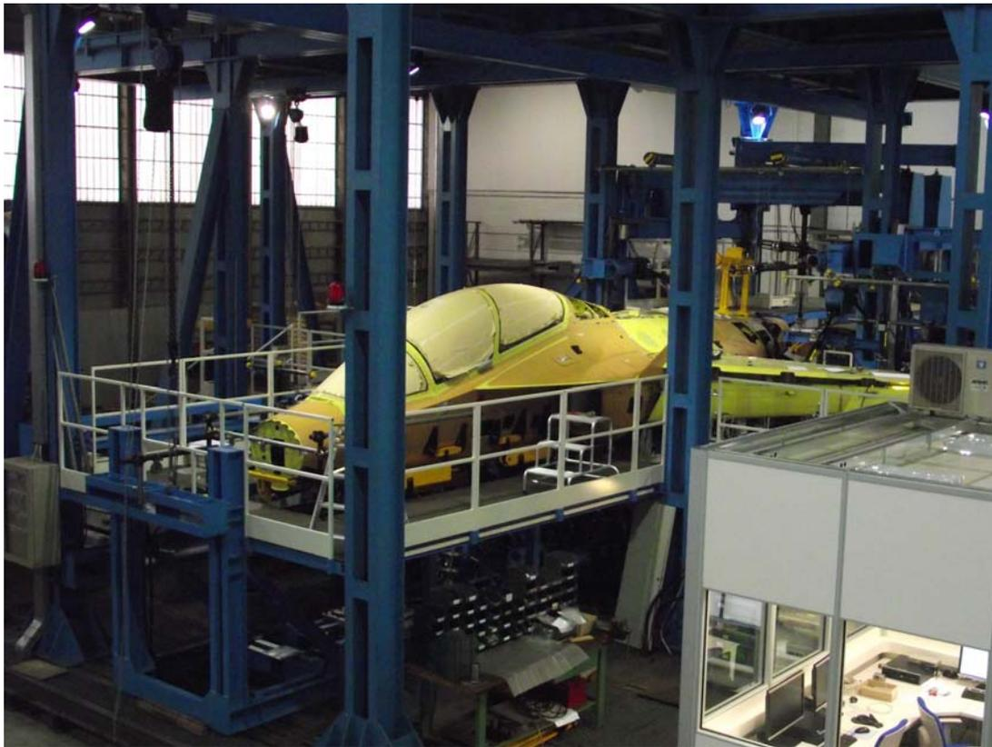
Fig. 34 - Preparation of the M346 Full Scale Fatigue Test
