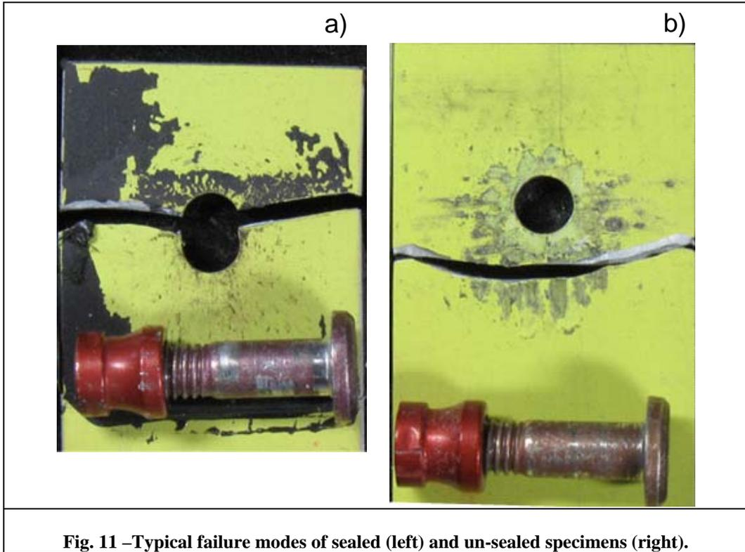
Fig. 11 – Typical failure modes of sealed (left) and un-sealed specimens (right).
