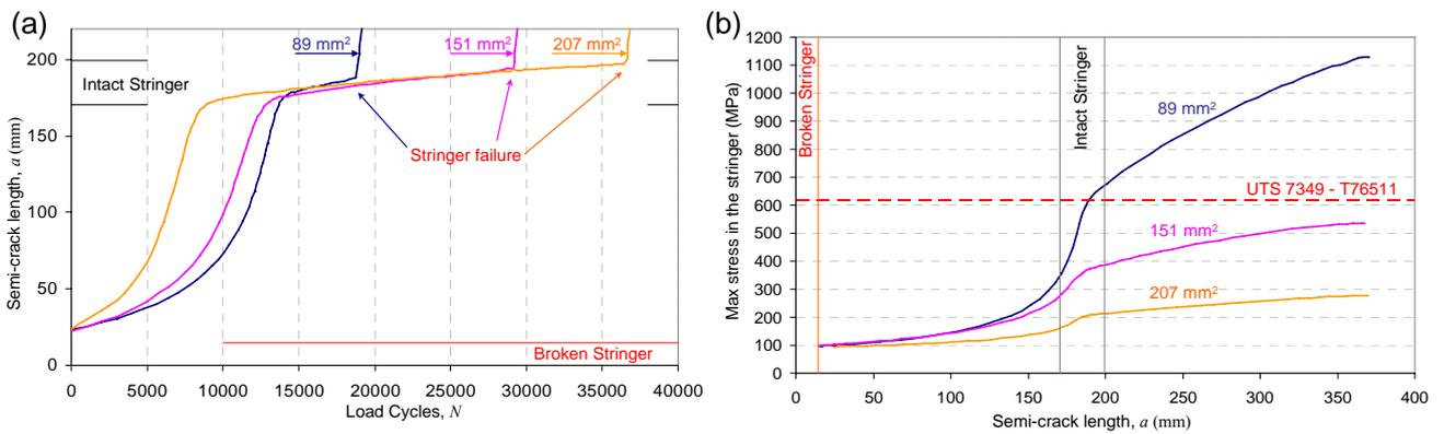
**Fig. 22 - FCP in bonded stiffened panels over a broken stringer: (a) experimental FCP curves; (b) analytically predicted maximum stresses in the stringer adjacent to the broken one. The panels have 7349-T76511, “z-shaped” stringers of, respectively, 89, 151 and 207 mm<sup>2</sup> cross-section.**
