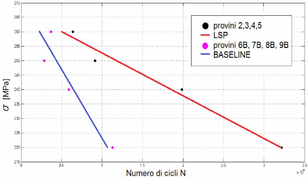
**Figure 18 - Fatigue lives of thick specimens treated with LSP.**
