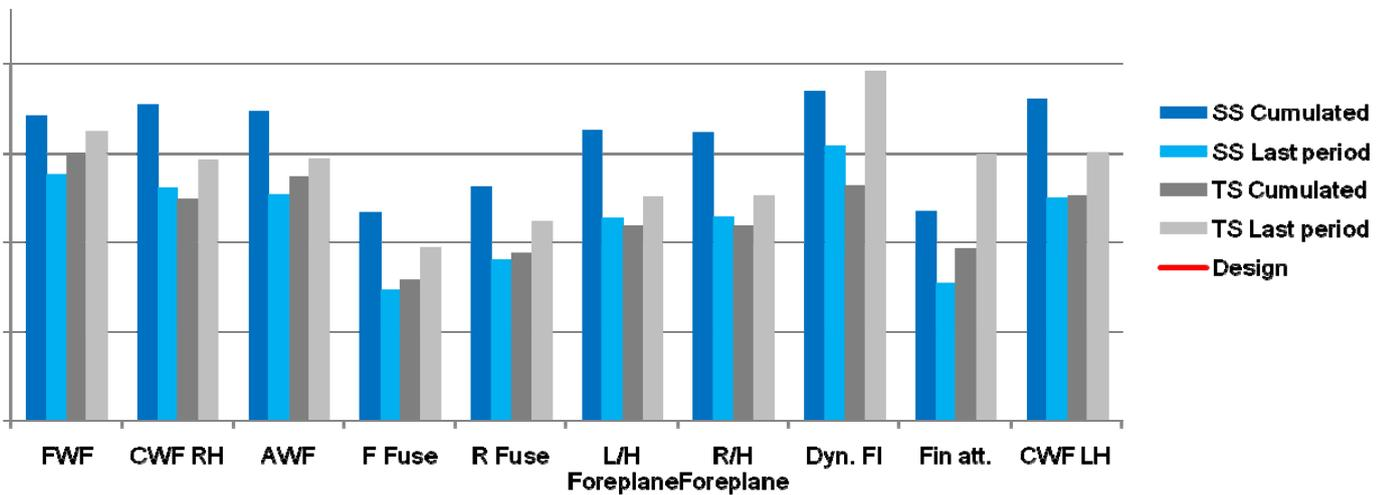
Fig. 4 - Fatigue Indexes values for IAF Typhoon aircraft.
