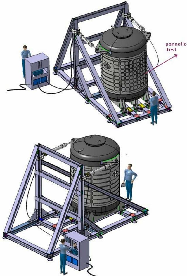
Fig. 25 - Barrel test set-up: sketch of the constraints and load application system.
