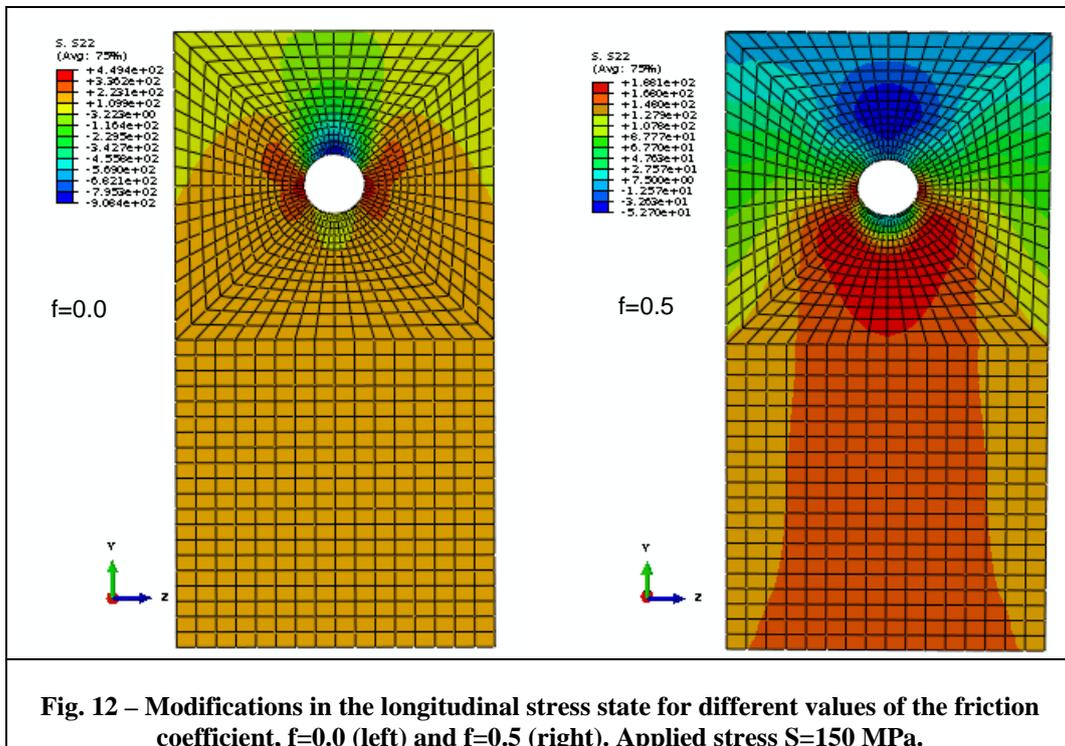
Fig. 12 – Modifications in the longitudinal stress state for different values of the friction coefficient,  $f=0.0$  (left) and  $f=0.5$  (right). Applied stress  $S=150$  MPa.
