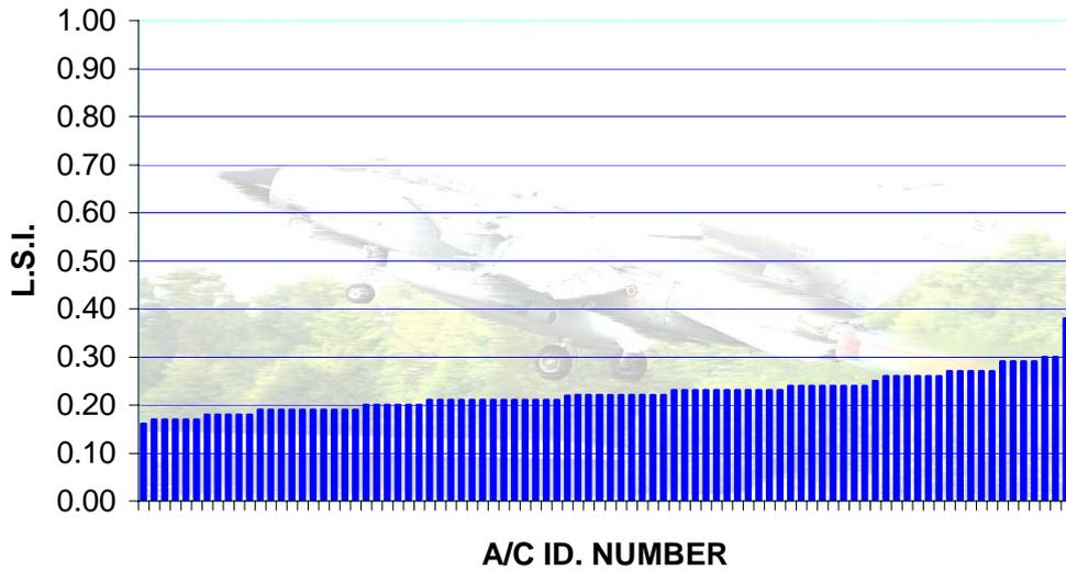
Fig. 3 - Load Severity Index trend for the aircraft of the I.A.F. Tornado fleet.
