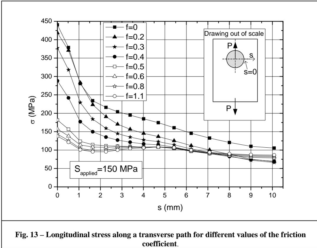
Fig. 13 – Longitudinal stress along a transverse path for different values of the friction coefficient.
