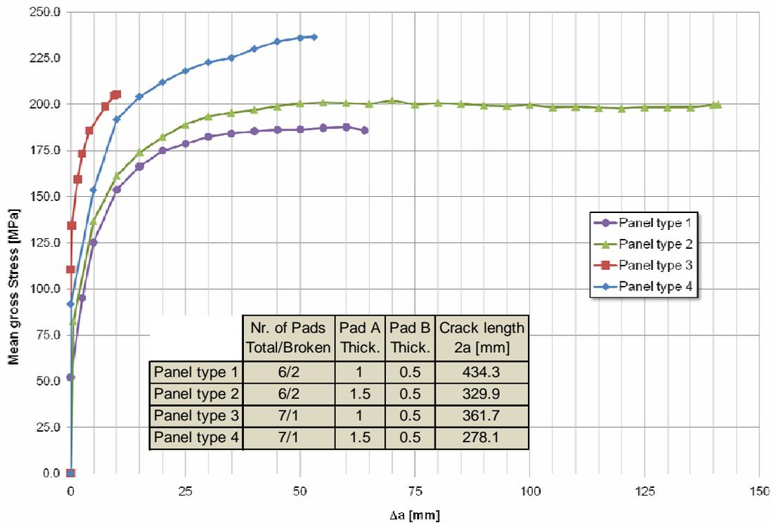
Fig. 20 – Summary of residual strength test results: mean gross stress vs.  $\Delta a$  curves
