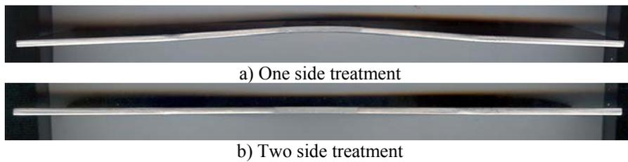
Fig. 16 - Deformation of the LSP treated specimen
