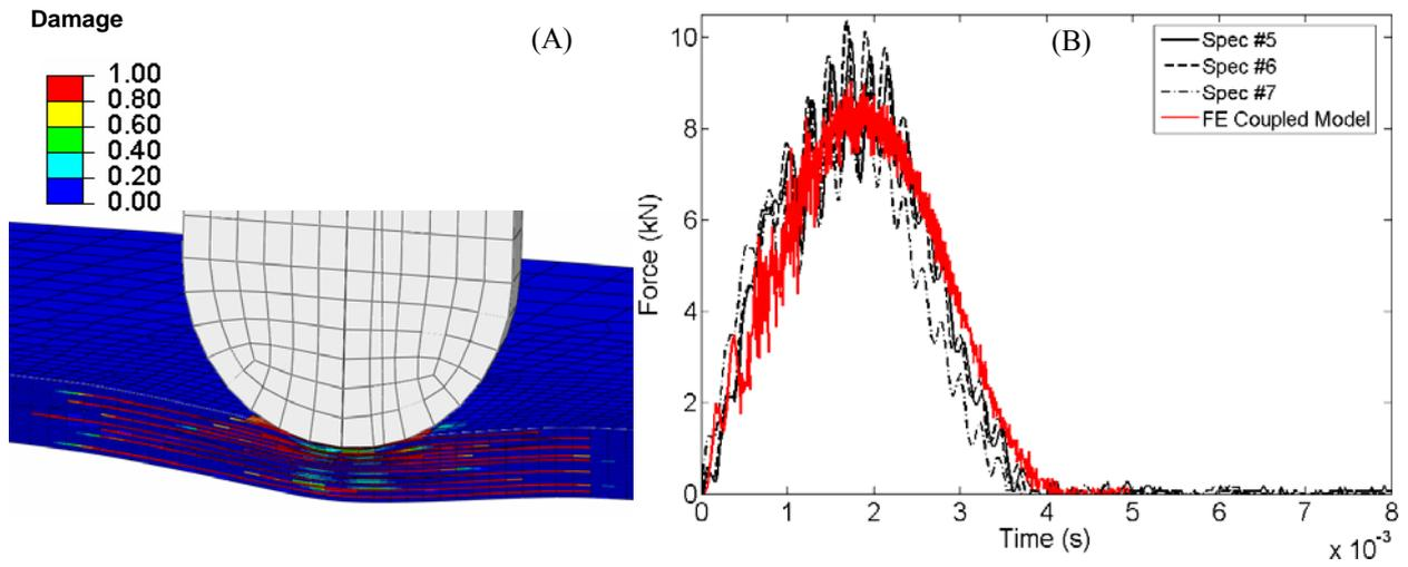
Fig. 29 – Low energy impact test simulation: (A) contour of interlaminar damage and (B) numerical-experimental correlation of the force vs. time history response
