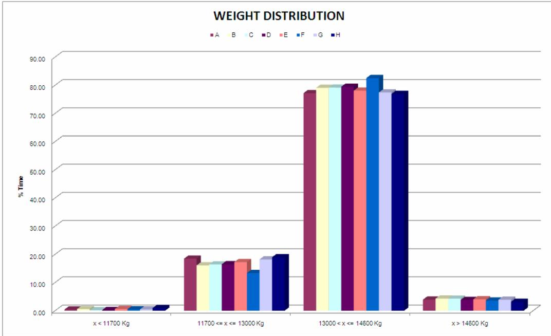
Fig. 5 - Weight distribution of the monitored machines of the Danish AW101 fleet.
