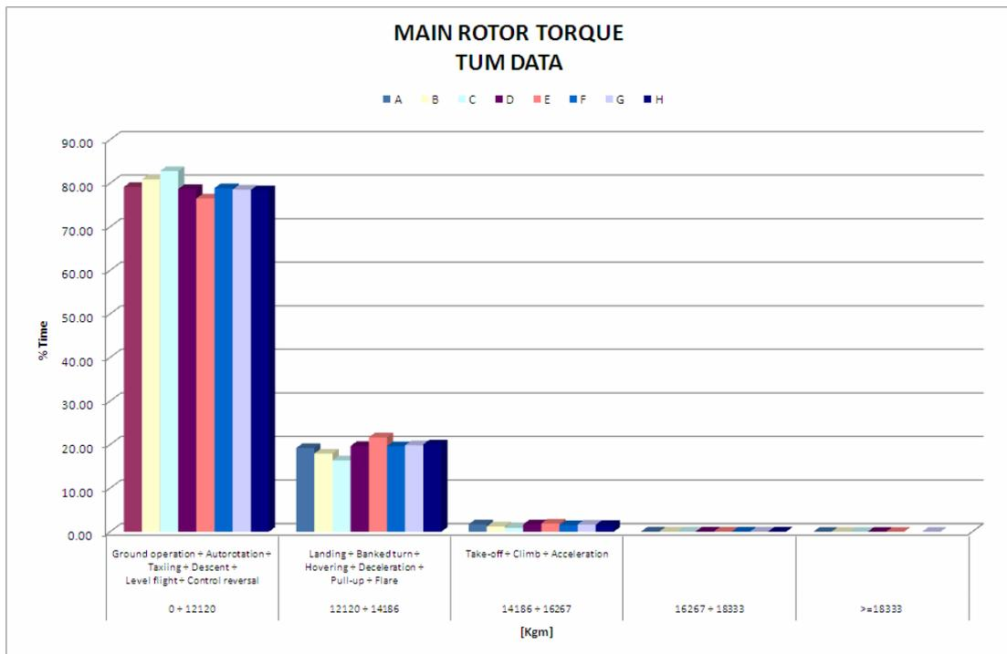
**Fig. 8 - Main Rotor Torque distribution in the AW101 monitored machines of the Danish fleet.**
