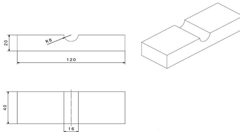
Figure 17 - Geometry of the thick specimen used to assess Laser Shock Peening effects.
