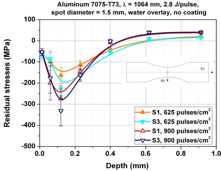
Fig. 15 - Residual stresses introduced in the treated specimen measured using hole drilling method.
