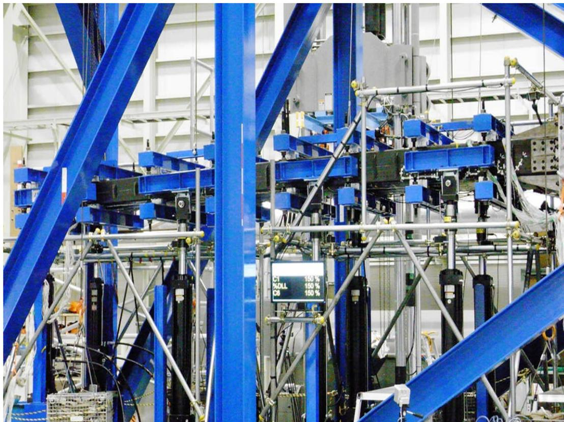
Fig. 42 Full-scale wing box ultimate load test
