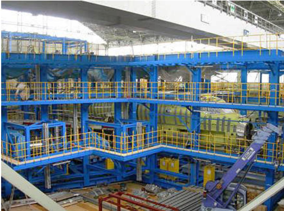
Fig. 40 Full scale static test airframe and loading fixture of XP-1
