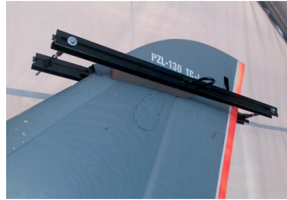
Wing sensors calibration and clamps used for wing and fin loading
