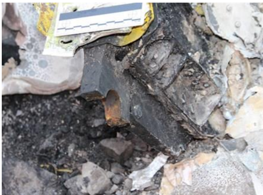
Figure 5: The left hand wing spar and lower attachment lug as found at the crack scene
