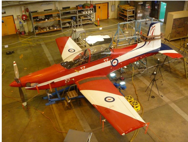
Figure 1: PC-9/A OLM aircraft during ground load calibration testing
