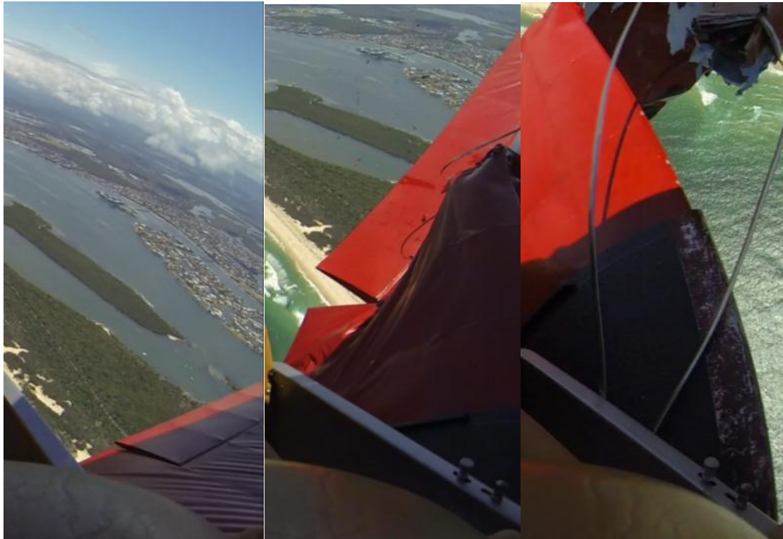
Frame 1: Failure Initiation Frame 2: 0.15 of a second Frame 3: 0.35 of a second
