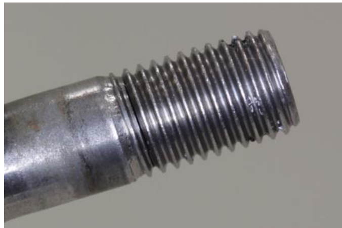
Figure 4: Threaded section of the tie rod. The black line in the base of the first thread is the crack
