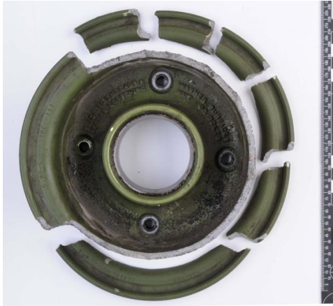
Photograph of the failed wheel and liberated wheel fragments, which encompassed approximately 75% of the circumference
