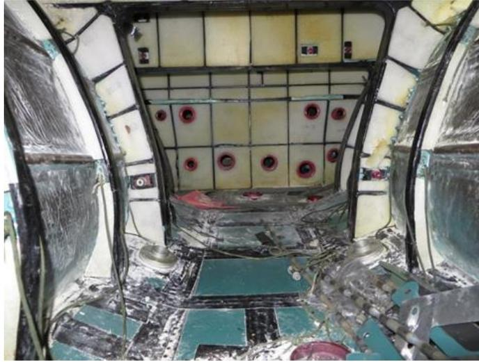
**Figure 4.3 F/A-18 Fuselage Fuel Tank**
