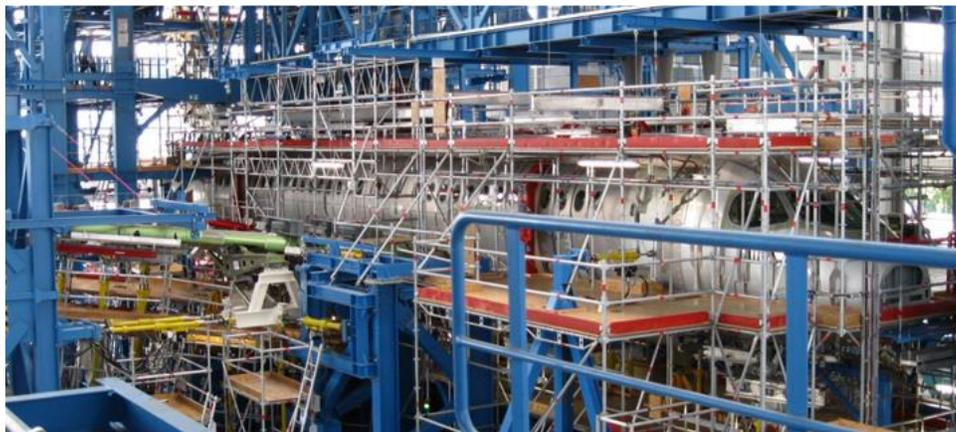
**Figure 2.9 Close of fuselage test setup**
