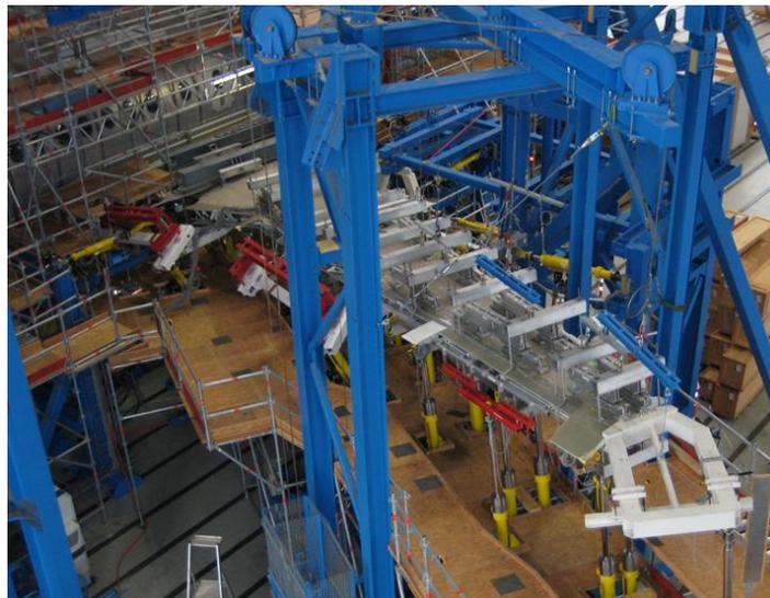
**Figure 2.8 Close-up of wing test setup**
