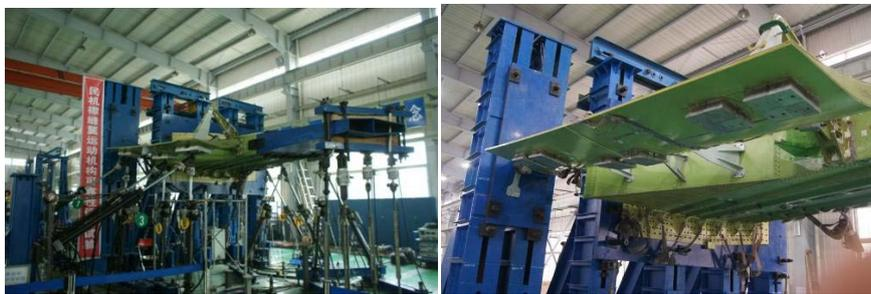
Figure 55. Fatigue reliability test of flap motion mechanism for ARJ21-700 aircraft.
