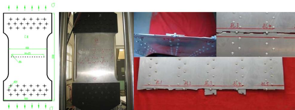
Figure 44. Fatigue and crack propagation of WFD structures.
