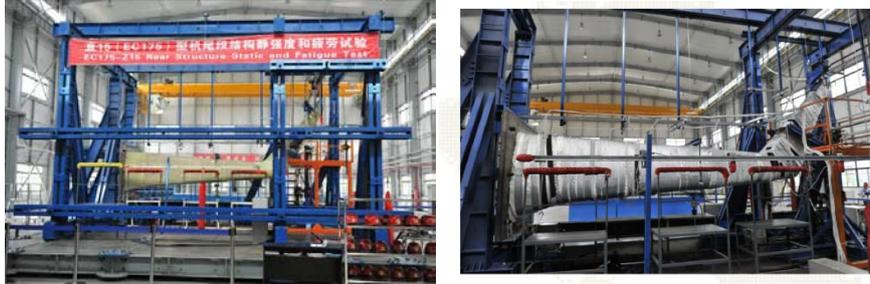
Figure 65. Static fatigue tests on empennage and horizontal tail for EC175/Z15 aircraft.
