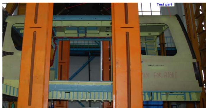
Figure 64. Middle airframe strength test.
