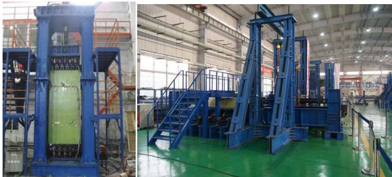
Figure 58. Fatigue and damage tolerance test on fuselage panel for civil aircraft.
