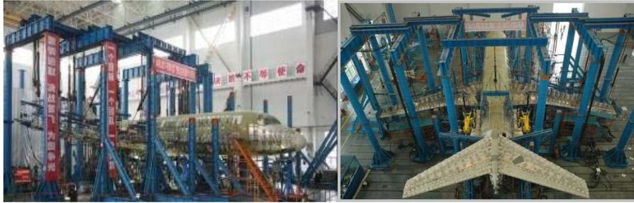
Figure 57. Integration frame loading system of full-scale static and fatigue test for ARJ21-700 aircraft.
