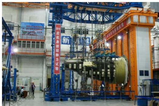
Figure 59. Static/fatigue test on fuselage segments for civil aircraft(airtight loading on positive and negative pressure).
