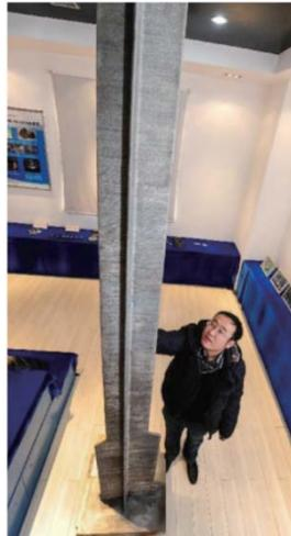
Figure 23. Central Wing flange of C919 aircraft by laser forming.
