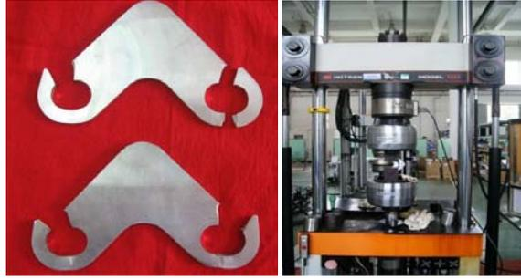
Figure 33. 45°lugs structure test.
