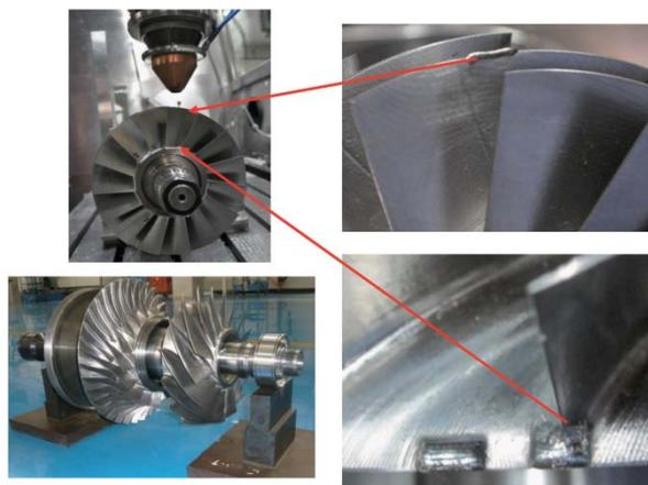
Figure 22. Damage repair of integral impeller by laser engineered net shaping.
