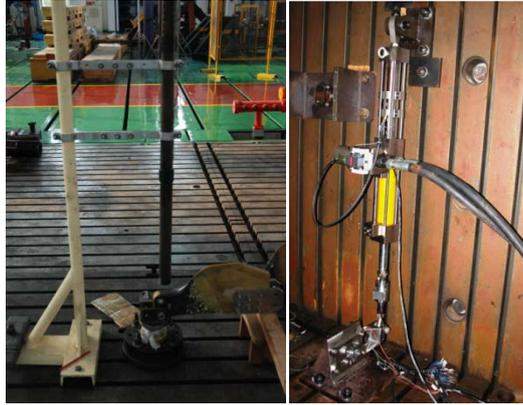
Figure 62. Defect tolerance test of helicopter blade.
