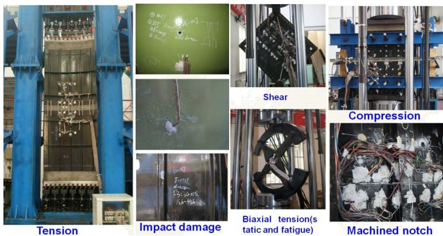
Figure 8. Damage tolerance and fatigue test of composite panels.
