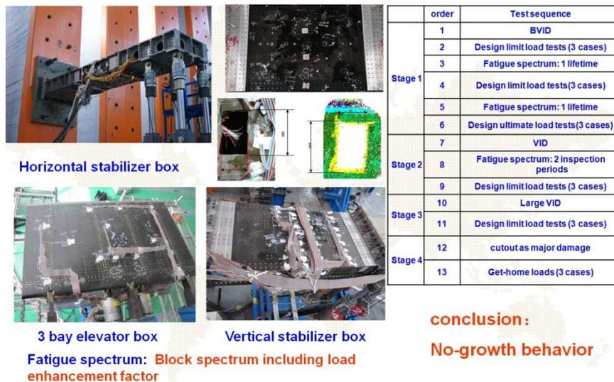
Figure 10. Damage tolerance and fatigue test of composite structure.
