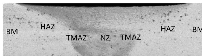
Figure 13. Macro-morphology of 2024-T3 aluminium alloy Friction stir welding joint .
