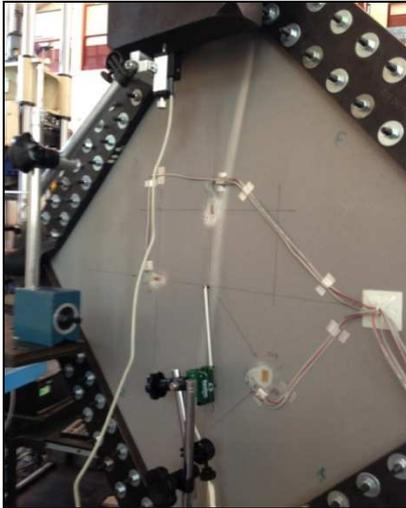
*a) Shear mechanical test*
