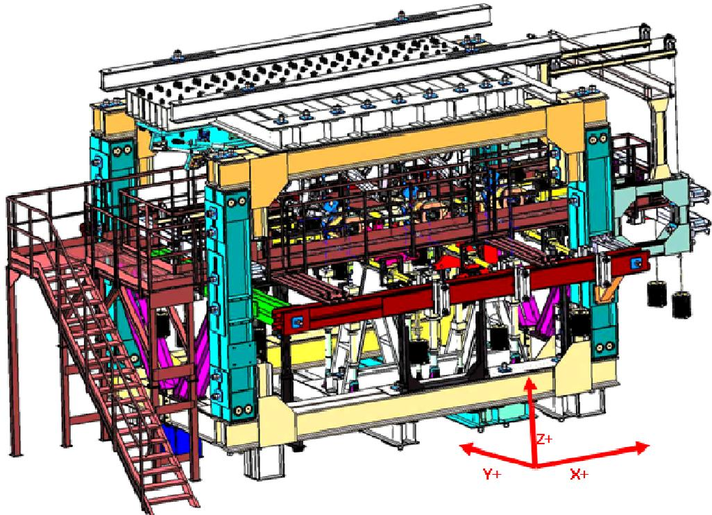
The loading is achieved using twenty four independent load channels (eight per leg), each fitted with spherical bearings at both ends. All load transducers are located as near as possible of the load introduction point to have a load value recorded by the transducer very close to the real load introduced into the specimen.
