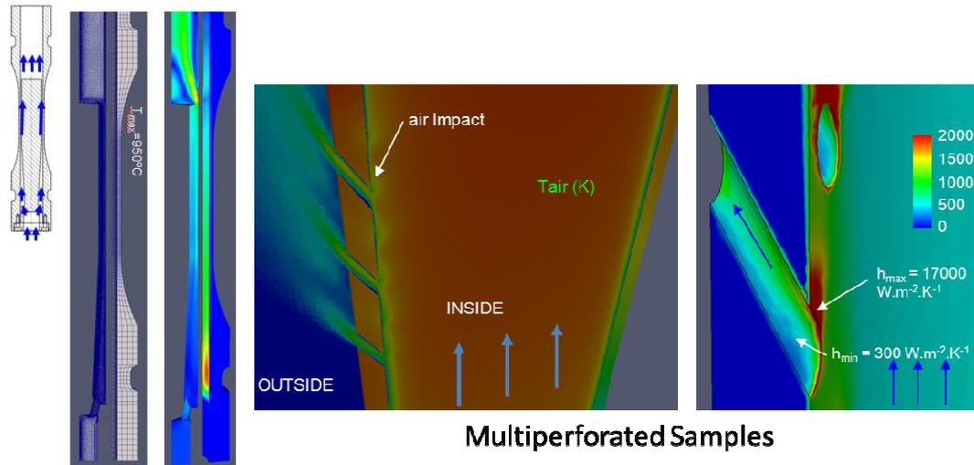
Figure 1: Thermal/Solid/Fluid coupled calculation: smooth specimen (left) and perforated specimen (right). Temperature contours and the convective heat transfer coefficient  $h$  governed by the fluid velocity
