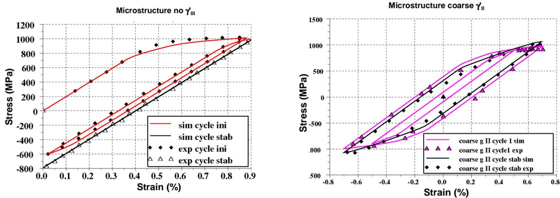
Figure 1: Influence of the precipitate distribution on the cyclic behaviour of coarse grain size superalloy N18 - Comparison of the model and the experimental response (on the first and stabilised cycle)
