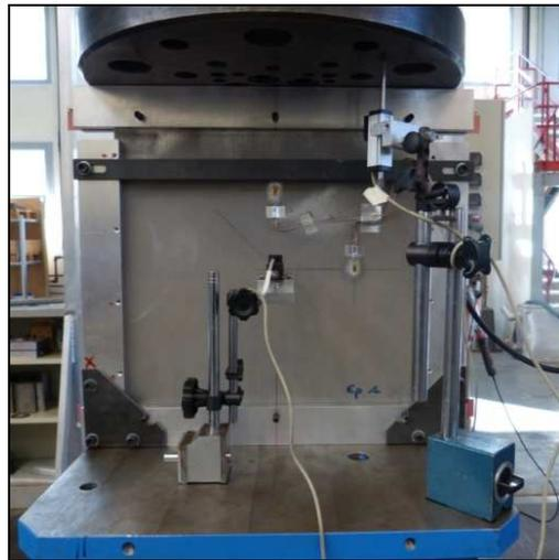
*b) Compression mechanical test*
