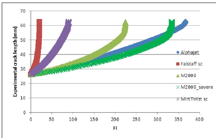
Figure 1: Experimental crack length versus FI
