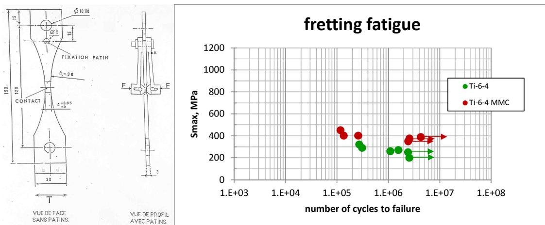
Fretting fatigue specimen set-up and test results.
