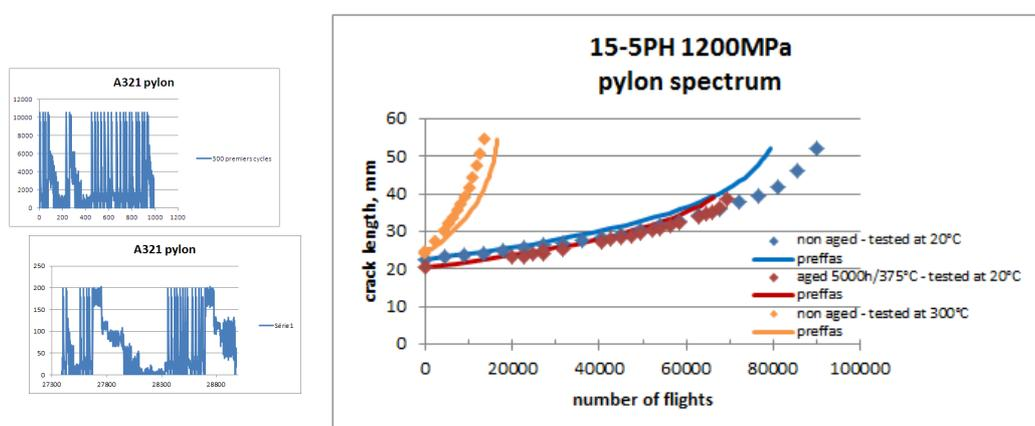
Fatigue crack growth on 15-5PH under pylon flight spectrum loading and PREFFAS calculations. Non-aged material tested at RT and 300°C, 5000h/300°C aged material tested at RT.
