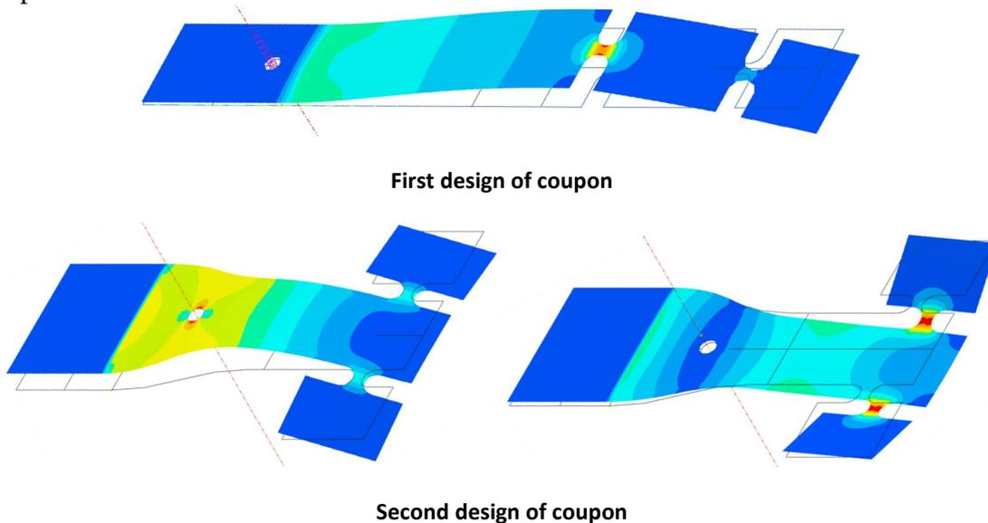
This optimization and the random excitation definition were made thanks to finite elements modelling (FEM) of the coupons and damage calculations with the different previous models. Finally, the first coupons tests enabled to adjust the complete model (FEM and damage calculation) and the second ones enabled to compare the models and to assess the possibility to make this type of damage prediction.
