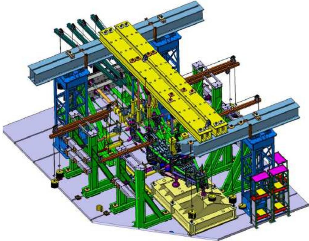
Design goal is 10,000 Flight Cycles with a scatter factor of 3, leading to simulate 30,000 cycles (SF). Load spectrum includes blocks of flights built on 120 different loading cases.
