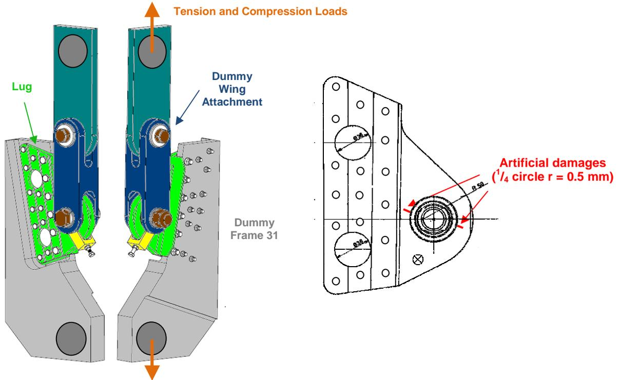
During the test, these damages have been followed up by NDT (US and Eddy Current): more than 10 fatigue lives of 7500 FH have been applied, without any propagation.
