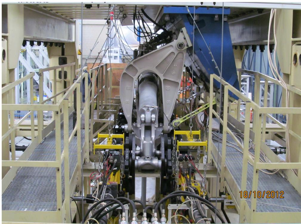
The aim is to simulate 50,000 cycles (SF) to validate 10,000 Flight Cycles (FC) which is the design goal. Load spectrum includes the application of combination of flights grouped in blocks of 200 flights. Load spectrum at the end is in line with the typical aircraft usage (mission mix) defined by a breakdown between four basic missions. Typical ground loads, kneeling actuator loads and extraction retraction loads are simulated.
