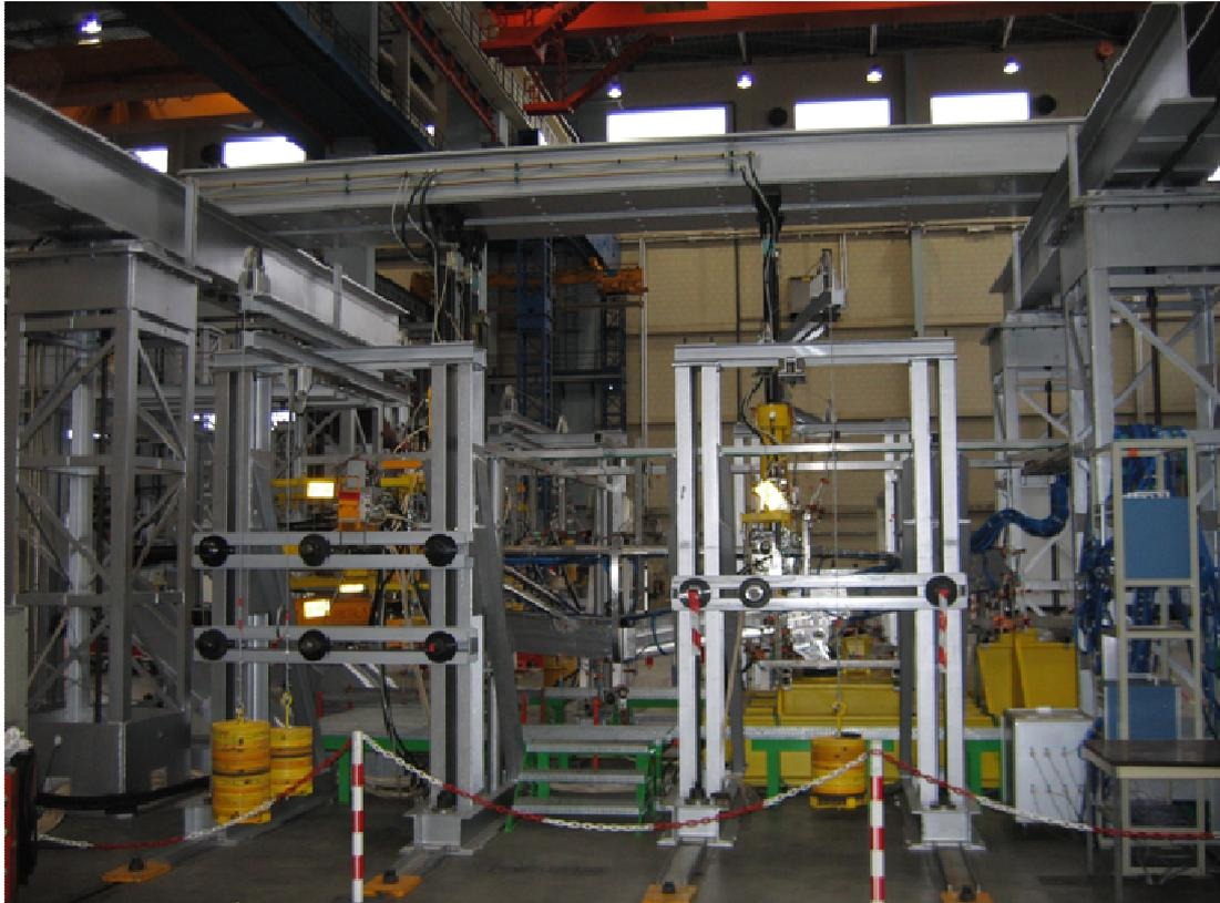
In the frame of A400M certification, DGA TA is performing the fatigue test of the A400M pylon. This fatigue test re-uses a test rig which was the one developed and used for the A400 pylon static test. The test installation includes 16 hydraulic jacks. Specimen behaviour is followed by 26 displacement transducers and by a maximum of 450 strain gages.
