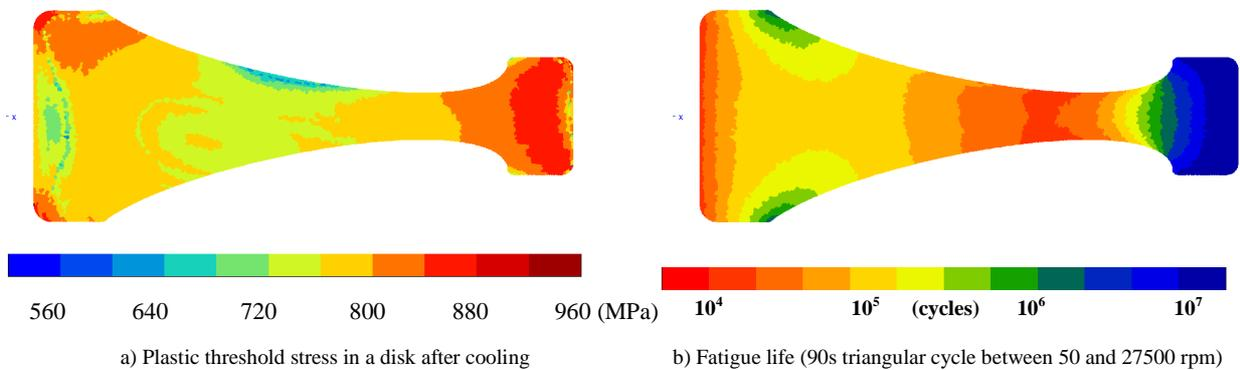
Figure 2: Maps of the different steps of disk calculation from the heat treatment to fatigue life at 450°C (half cross-section, the rotation axis on the left)
