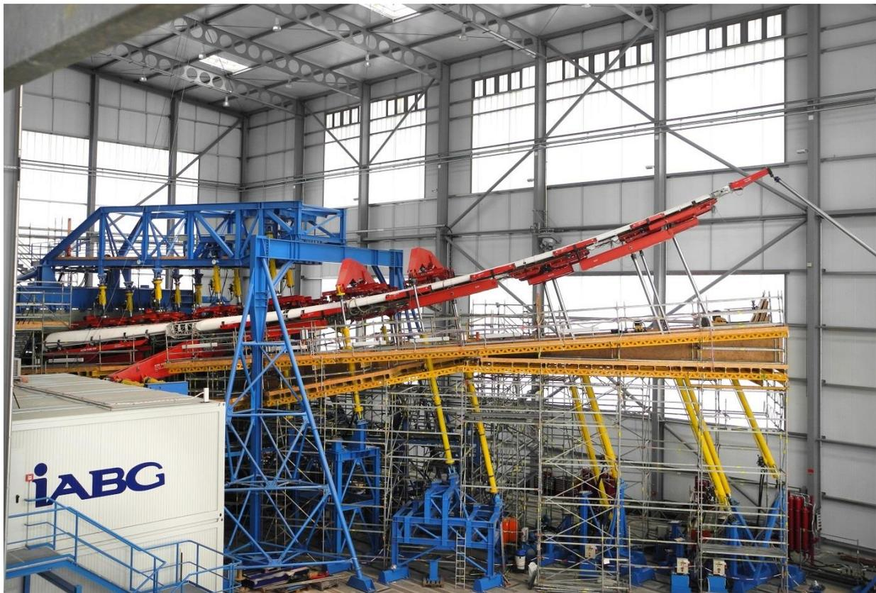
**Figure 2-3: Ultimate load up bend test at the A350 XWB EW test at IABG**
