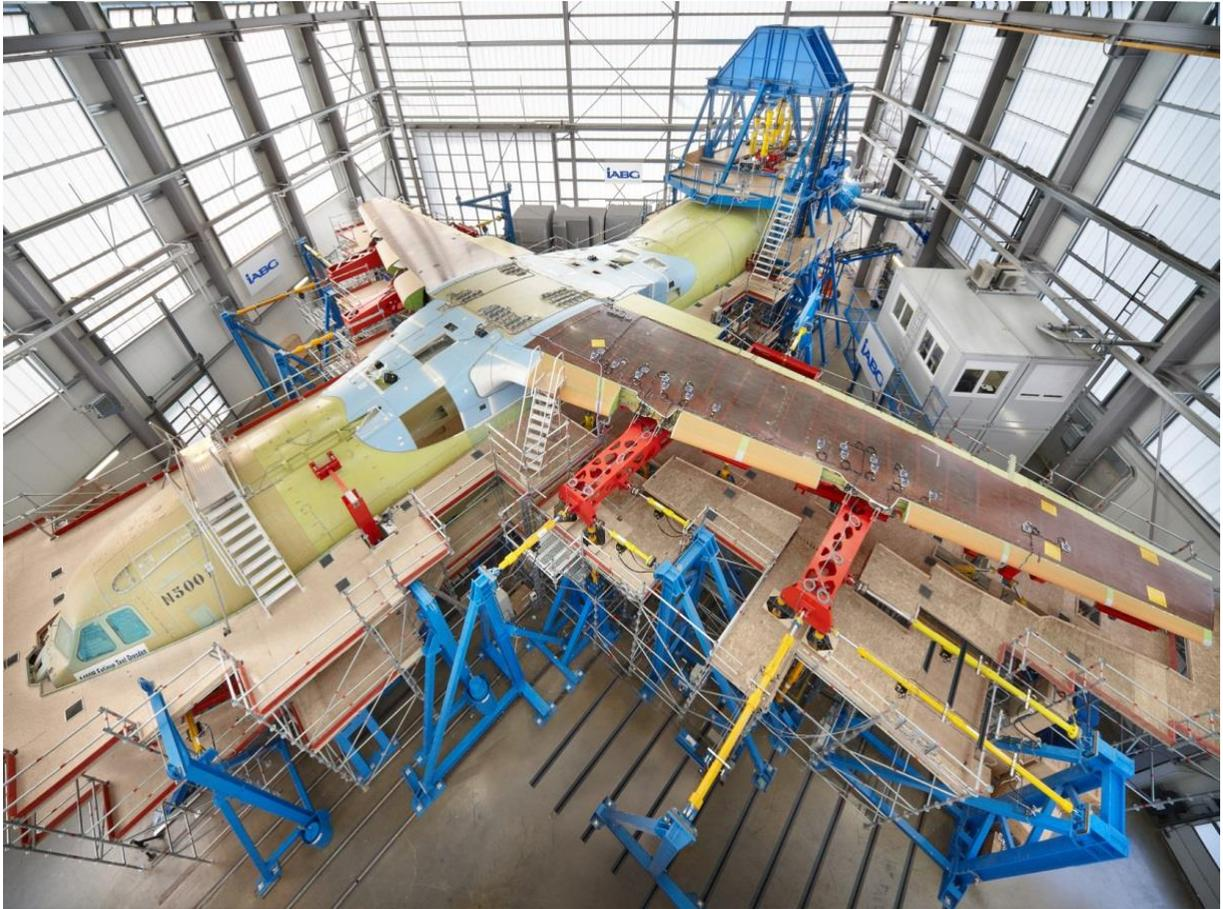
**Figure 2-4: A400M FSFT test set up at IABG**
