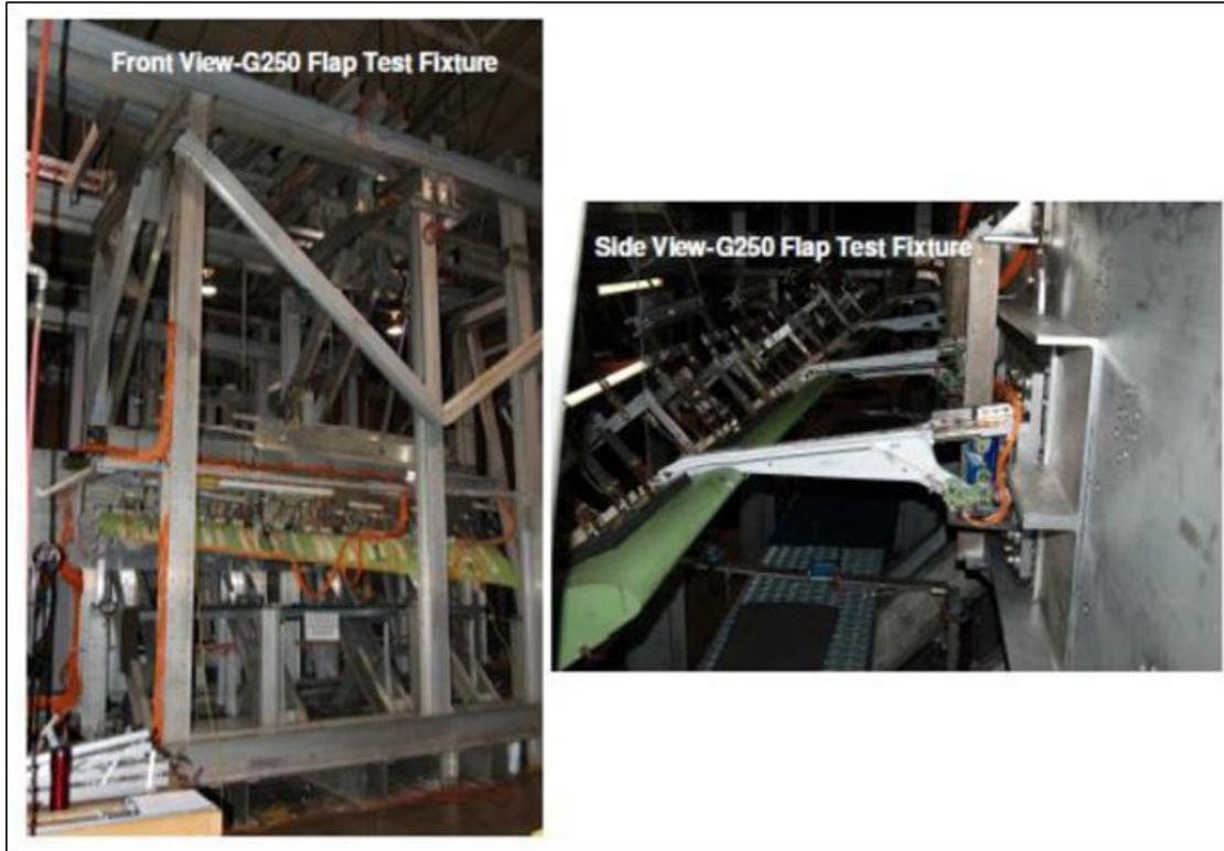
**Figure 9. Flap test setup and the loading system**
