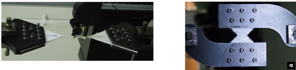
**Figure 27. Left: Bow-tie specimen installed on the tension machine with extensometer; Right: Butterfly specimen assembled with pin holders. The top surface of the sample is randomly scattered with black and white small paint drops for DIC.**
