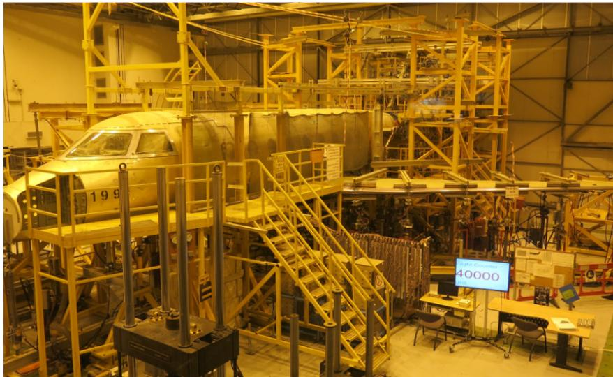
**Figure 3. Complete Airframe Mounted in its Fixture upon completion of two lifetimes (40,000 flights)**
