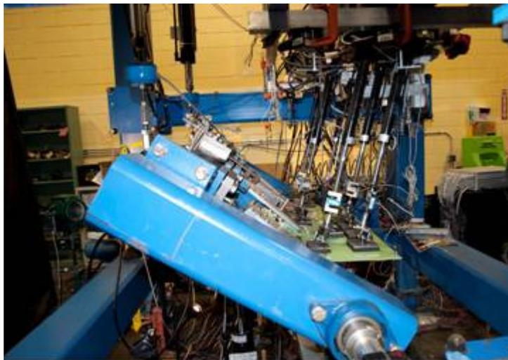
**Figure 7. Spoiler article mounted in test fixture upon completion of residual strength test**
