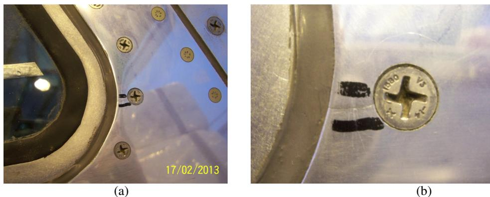
**Figure 1. (a) cracked retainer. (b) Zoomed view of the crack between the window cutout and the nearby fastener hole**
