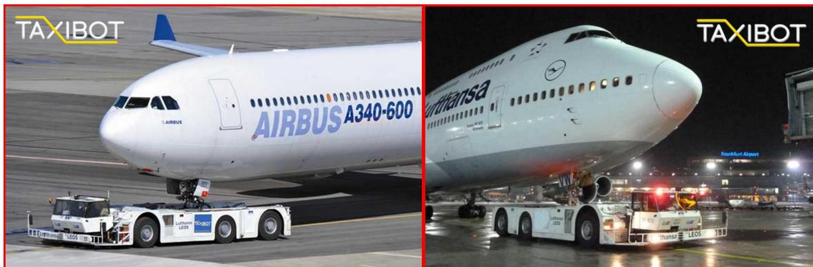
**Figure 39. Airbus A340-600 and Boeing B747-400 towed by TaxiBot**
