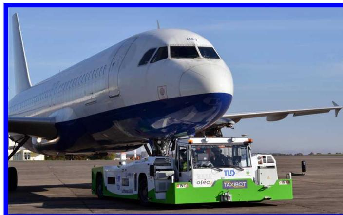
**Figure 40. TaxiBot NB prototype towing the Airbus A320-200**
