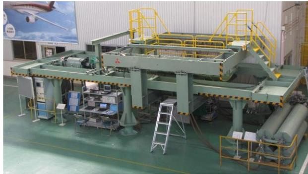
Fig. 39 Curved Panel Fatigue Test Fixture for MRJ200
