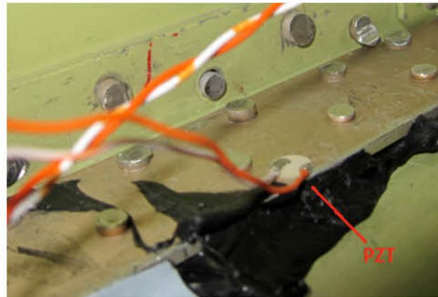
b) Damage developing after PZTs placement
