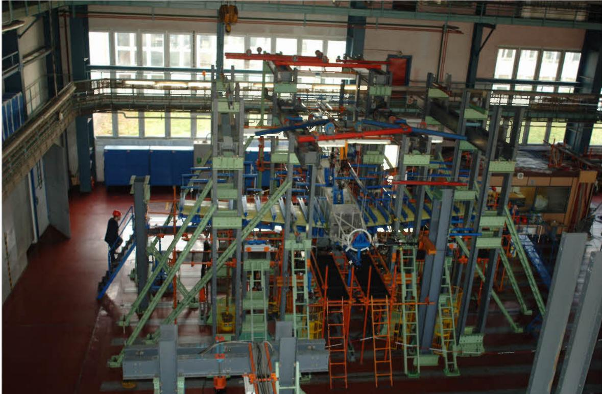
*Fig. 16 Full Scale Fatigue Test Bed*
