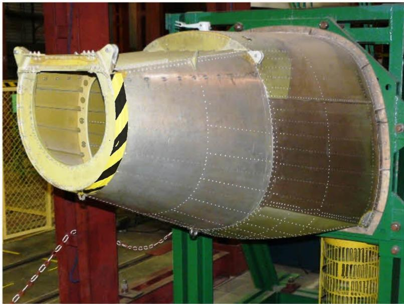
*Fig. 8. PZL M28 05 empennage fatigue test fixture. The fuselage part used in test is visible on the photo (empennage is dismantled).*
