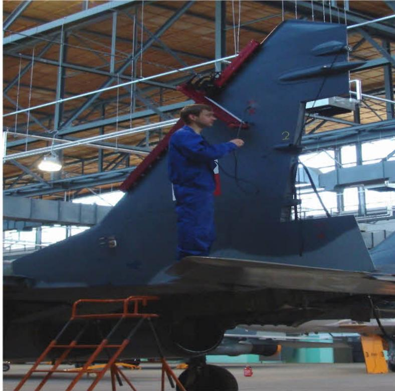
*Fig. 3. Composite Vertical Stabilizer Inspection*
