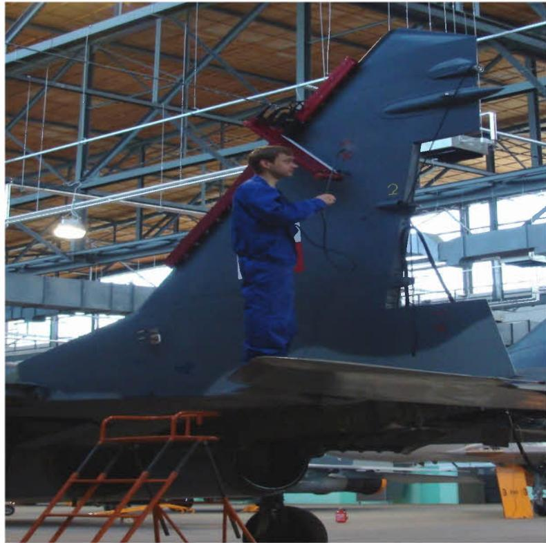
*Fig. 3. Composite Vertical Stabilizer Inspection*
