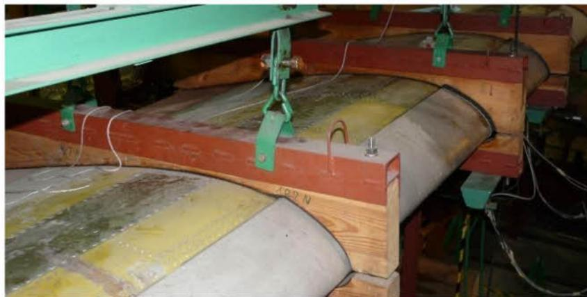
*Fig. 4. PZL M28 05 wing and wing load carry-through structure fatigue test fixture. Clamps introducing loads to the wing are shown.*
