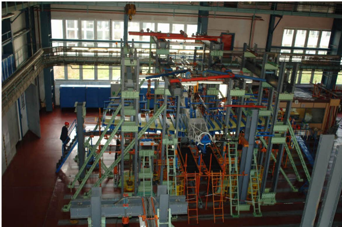
Fig. 16 Full Scale Fatigue Test Bed
