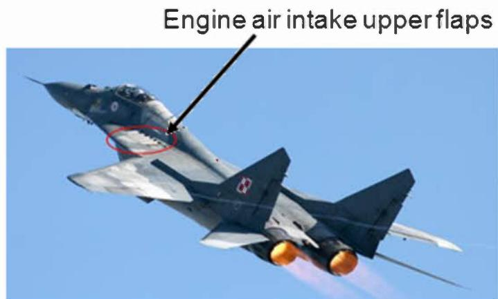
*Fig. 10. Engine air intake upper flaps location*
