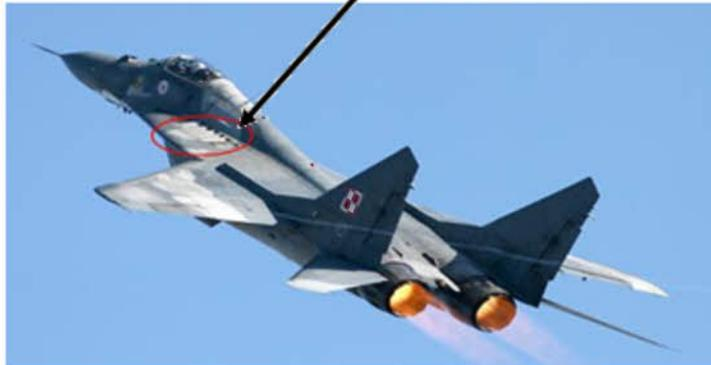
*Fig. 10. Engine air intake upper flaps location*
