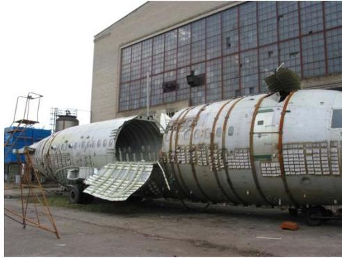
Figure 5. Durability tests of pressurized fuselage.
