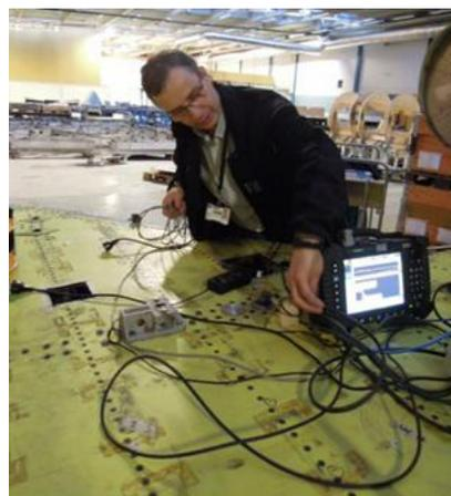
Figure 1. Canard wing lower skin, zone sections Figure 2. Testing of Pitch Catch equipment
