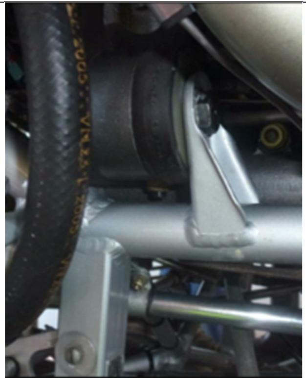
**Figure 37:** Detailed picture of aft engine mount fairing
