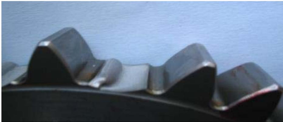
(a) Root Failure (RF)
