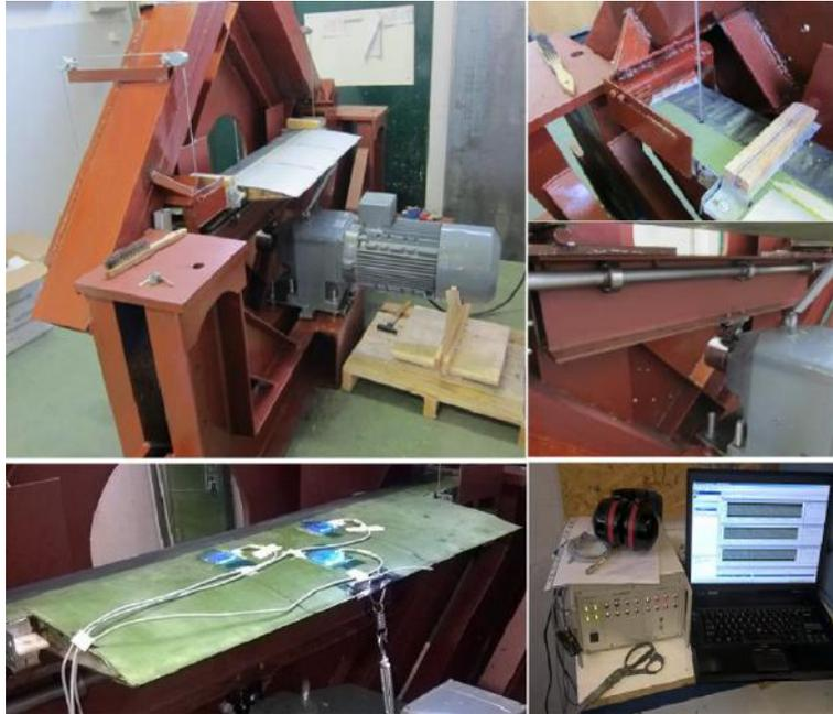
**Figure 5. Test rig for fatigue test of rotor blade sample.**
