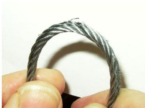
*The damaged cable KSAN 3,5 removed from the aircraft*
