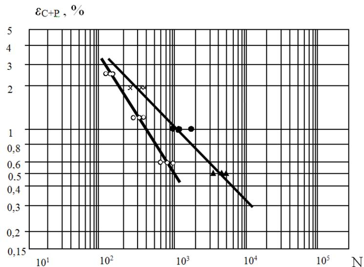
Figure 11.2.2 Influence of vibration loads on the thermal fatigue durability of ZhS6U alloy: x - 2 % ; • - 1%, ▲ - 0,5 %; ○ – with imposed vibration.
