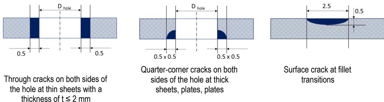
Figure 2.1 Typical damages or initial manufacturing defects recommended for considerations while analysis
