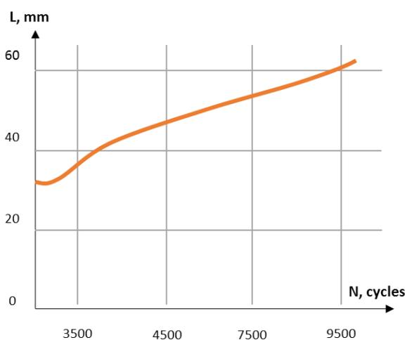
Figure 8.2.2 Crack growth in cargo door edge obtained from test
