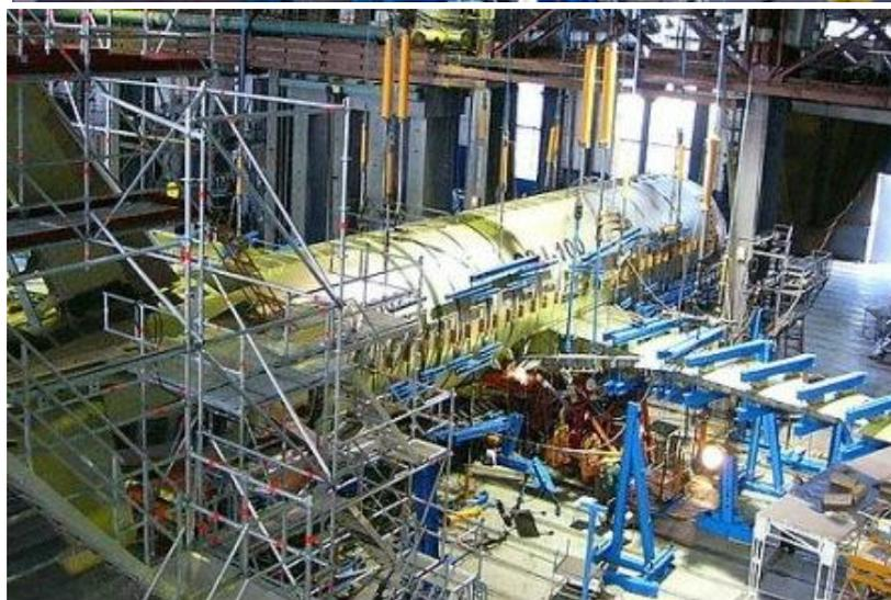
Figure 11.1.1 Tests of SSJ structure and elements
