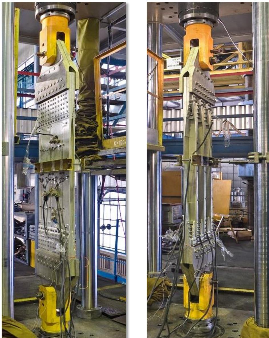
Figure 10.1.4 Fatigue tests of "3-stringer" panel specimens representing wing structure of IL-76MD-90A aircraft
