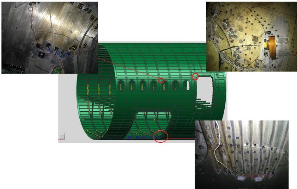
Figure 8.2.1 Fuselage full-scale section of MC-21 -300 airplane used for damage tolerance tests followed by residual strength tests
