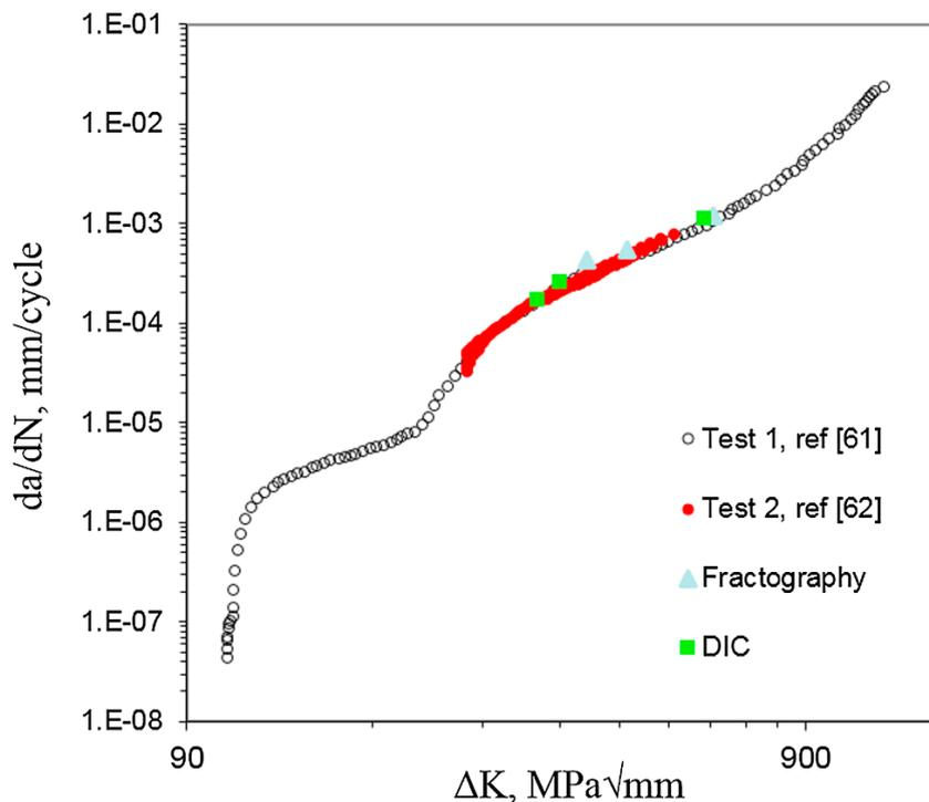
Figure 3.2.2 Crack propagation data from different sources plotted together with data obtained the SEM fractographies and the DIC estimations of the SIF.
