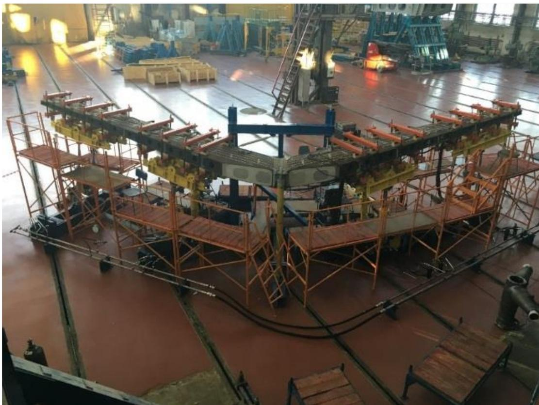
Figure 6.3.1 Composite structures of MC-21-300 empennage surfaces at fatigue tests
