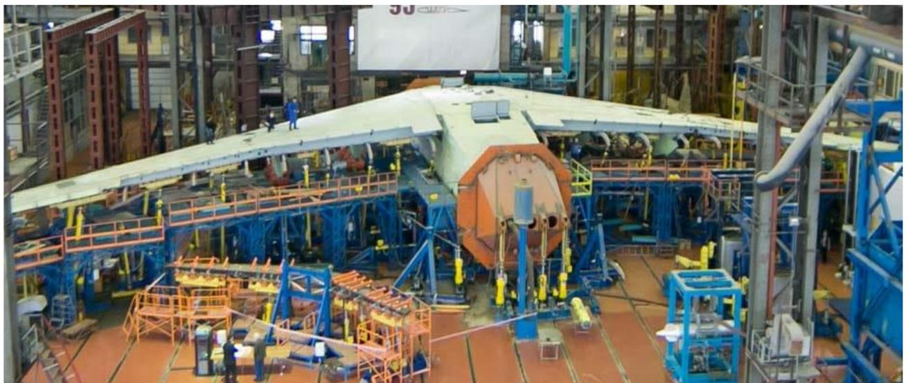
Figure 10.1.3 Static test of wing - central fuselage section with main landing gear in TsAGI lab
