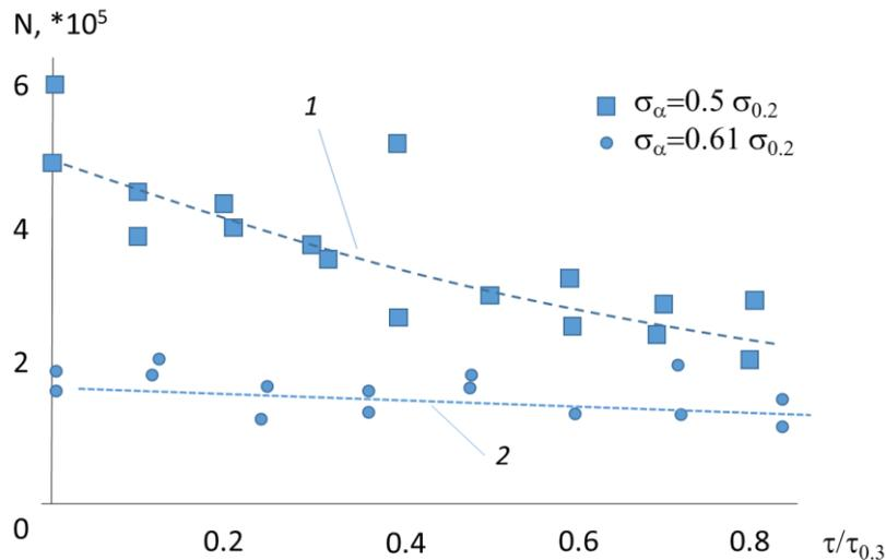
Figure 3.3.1 Dependence of fatigue life of 2024 alloy ta cyclic tension with amplitudes  $\sigma_a = 0.5\sigma_{0.2}$  (1) and  $\sigma_a = 0.61\sigma_{0.2}$  (2) versus constant component of shear stresses
