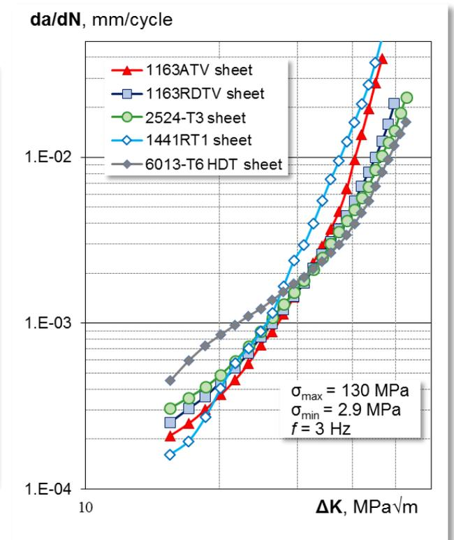
Figure 3.1.6 Crack growth curve of the fuselage skin material
