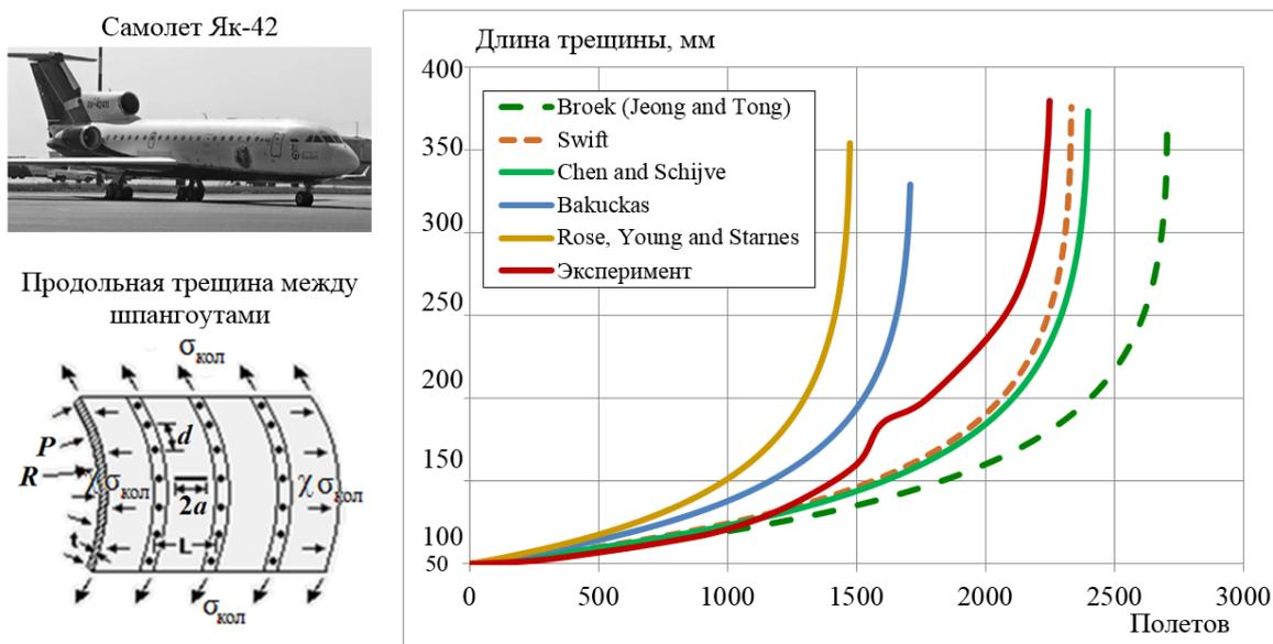
Figure 8.1.1 Comparison of computed and experimental results of longitudinal crack growth between ribs obtained using the various buckling models (Yak-40 airplane)
