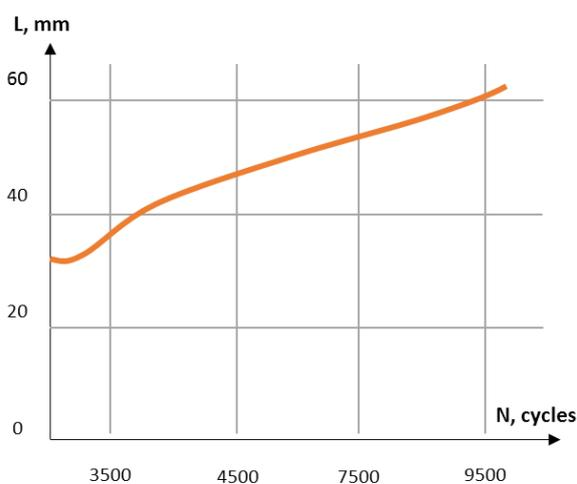
Figure 8.2.2 Crack growth in cargo door edge obtained from test
