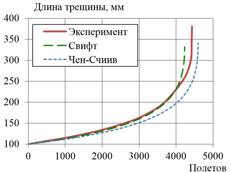
Figure 8.1.2 Comparison of computed and experimental results of growth of two –bay longitudinal crack in case of broken frame
