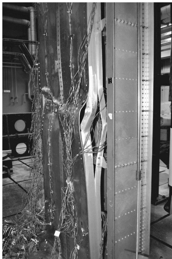
Figure 8.2.2 The panel after general loss of stability
