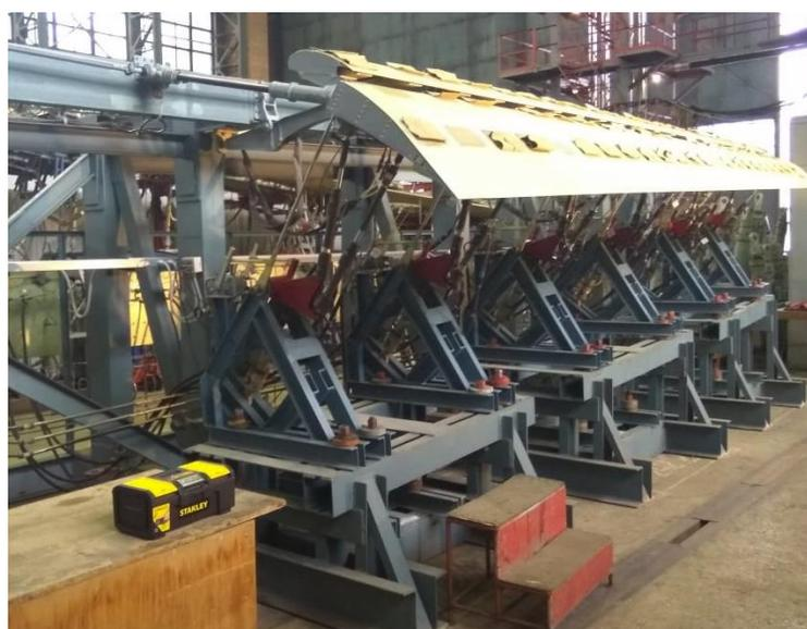
Figure 10.2.2 Test of IL-112 flap mechanisms for operation & functionality
