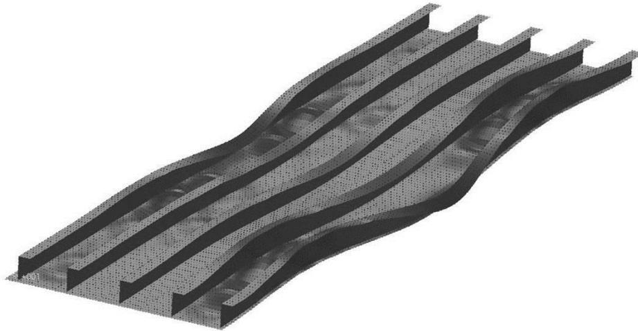
Figure 8.2.3 . Buckling of for monolithic panels obtained by calculation
