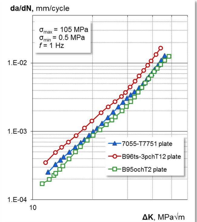
Figure 3.1.4 Crack growth curve of the wing upper surface material
