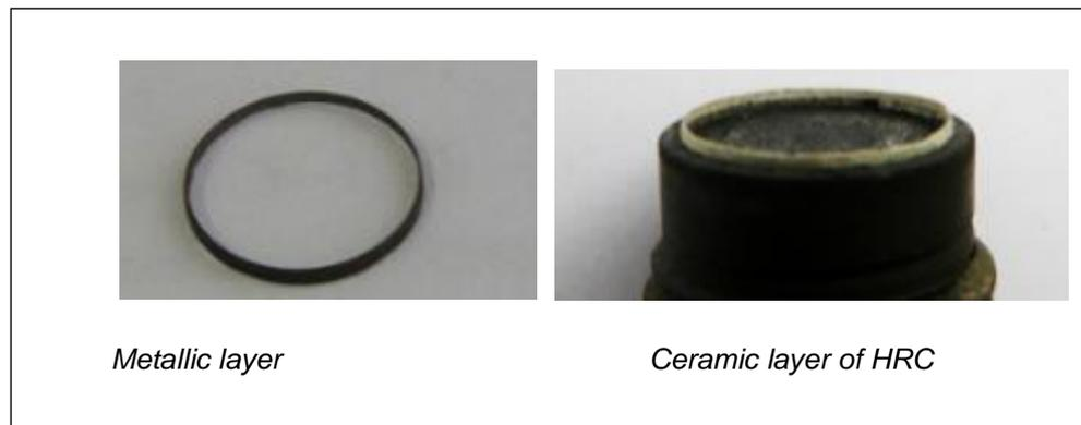
Figure 11.1.2 Sublayer and ceramic layer of HRC after tests
