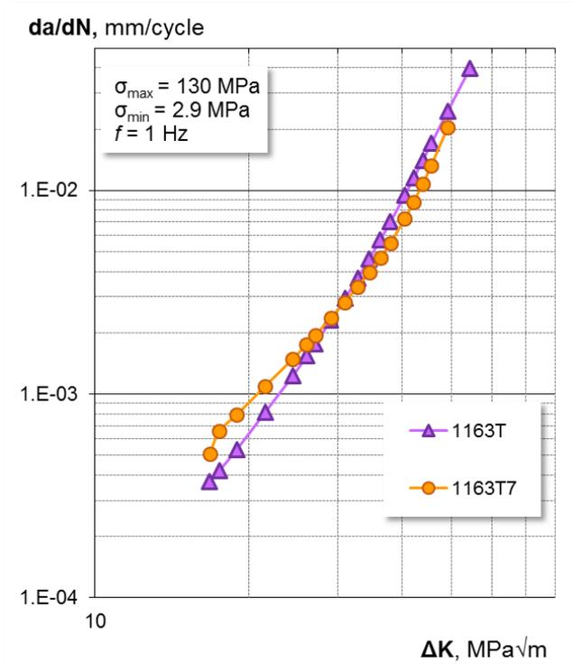
Figure 3.1.3 Crack growth curve of the wing lower surface material
