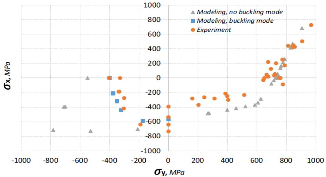
Figure 4.6.2 Biaxial failure envelope (0/ ± 45/90) AS4/3501–6 epoxy laminate under combined  $\sigma_x$  and  $\tau_{xy}$  stresses
