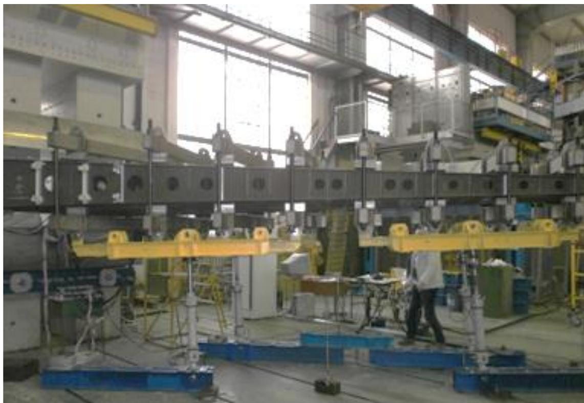
Figure 6.3.2 MC-21-300 airplane vertical fin composite structure at fatigue tests
