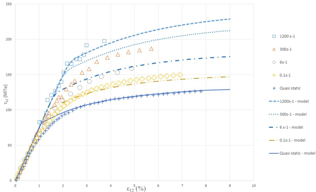
Figure 4.5.1 Experimental and predicted inplane shear loading diagrams
