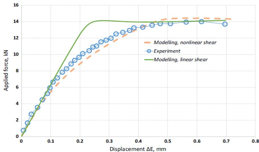
Figure 4.6.3 Experimental and predicted loading diagrams with linear and nonlinear shear stiffness
