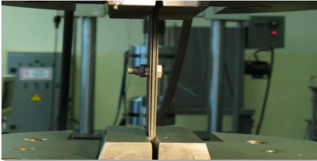
Figure 4.3 Photo of the tested strip CFRP specimen installed in the test rig
