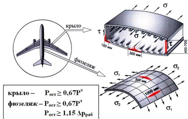
Figure 2.2 Airframe regulated damages
