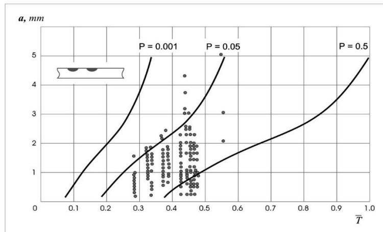
Figure 9.3 The relative growth of MSD cracks in IL-62 wing panel joint, upper surface, found in operation
