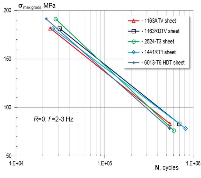
Figure 3.1.5 Fatigue curve of the fuselage skin material
