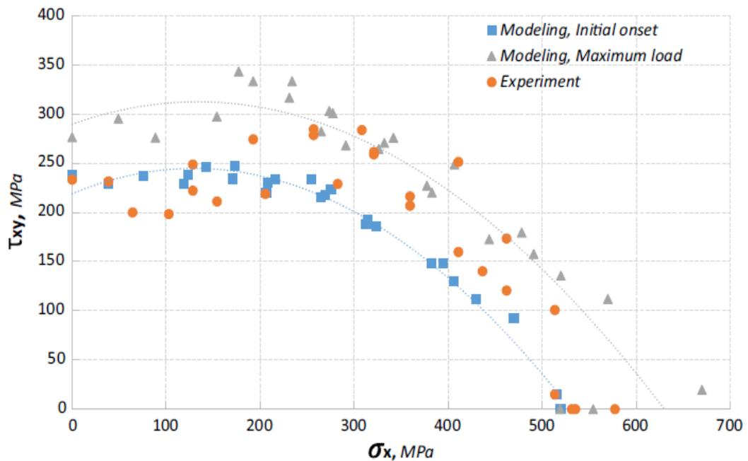
Figure 4.6.1 Biaxial failure envelope for [90/±30/90] E-glass/LY556 epoxy laminate under combined  $\sigma_x$  and  $\tau_{xy}$  stresses
