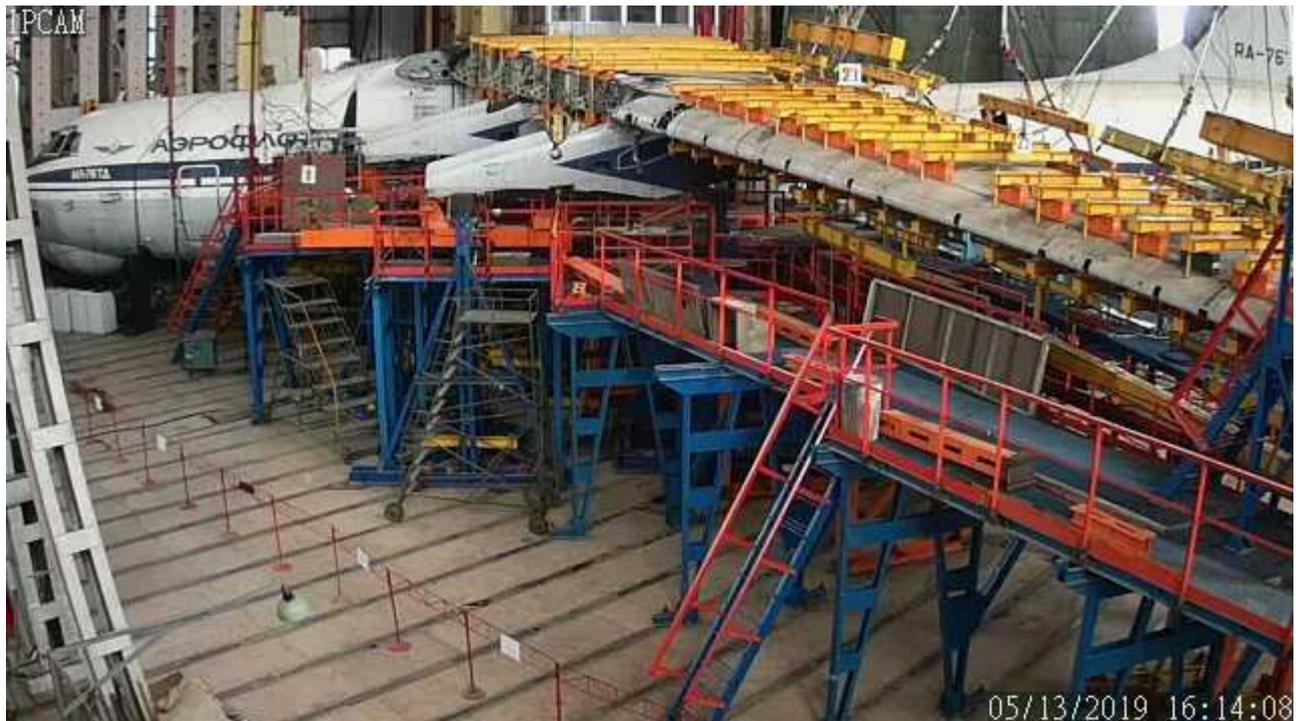
Figure 10.1.2 IL-76MD Fatigue tests of aircraft structure elements in lab
