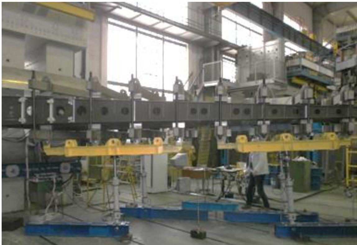
Figure 6.3.2 MC-21-300 airplane vertical fin composite structure at fatigue tests
