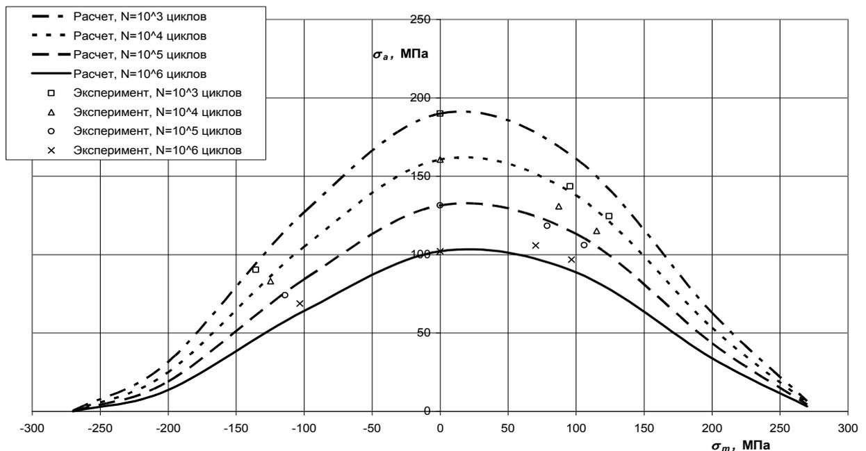
Figure 4.2 Cycle limit amplitude diagrams based on the Beheshti-Harris-Adam equation for the open hole specimen made of AS4-PW carbon fiber
