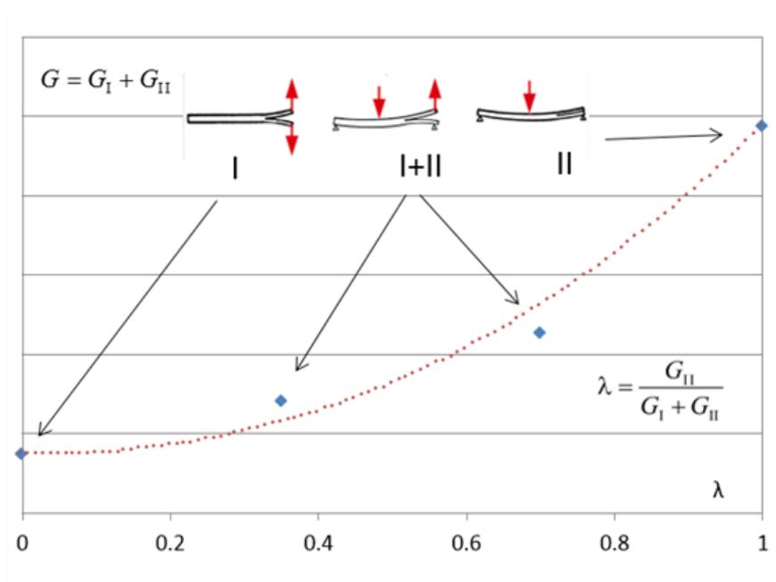
Figure 4.4.1 The average values of fracture toughness for different fracture modes of advanced CFRP material applied in the structure of transport aircraft
