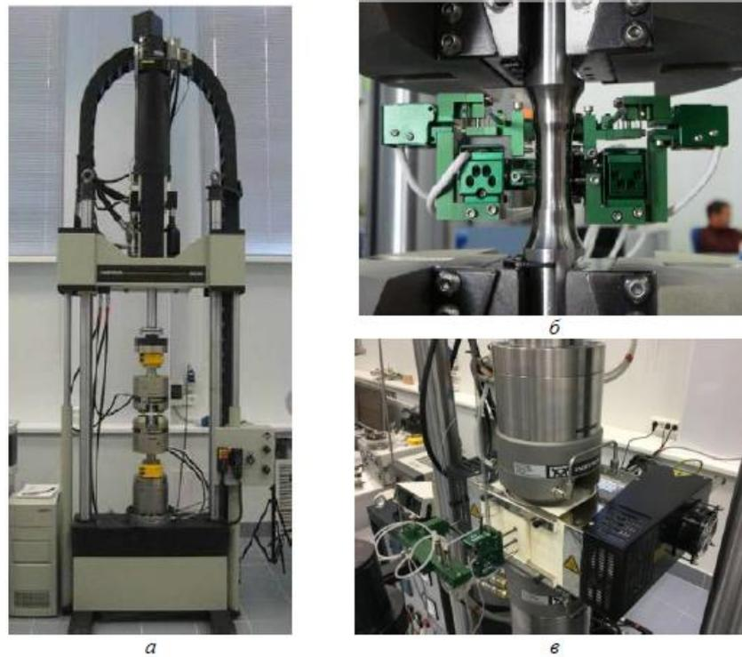
Figure 3.4.1 Servohydraulic test system Instron 8850 (a). Dual-axis strain sensors installed on the sample for testing at normal (b) and high temperatures (c)
