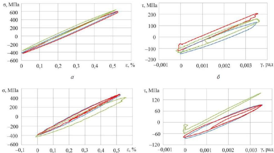
Figure 3.4.3 Characteristic hysteresis loops of low-cycle fatigue at room (a and b) and high temperatures (c and d) and three different cyclic deformation diagrams (blue – simple loading with a triangular cycle mode, red is simple loading with M- the figurative cycle mode, green color – complex loading)
