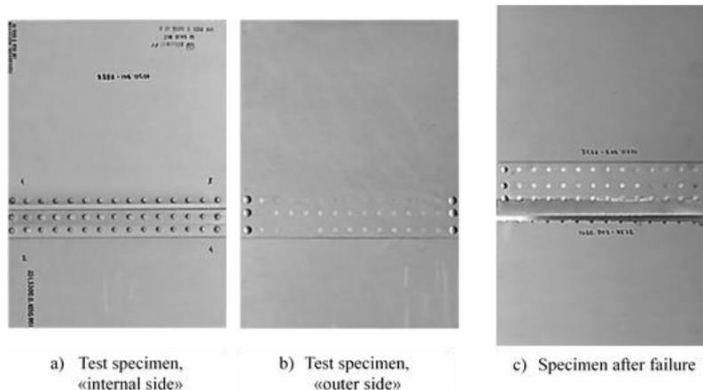
Figure 9.4 Specimen of longitudinal fuselage skin joint made of 1163RDTV alloy
