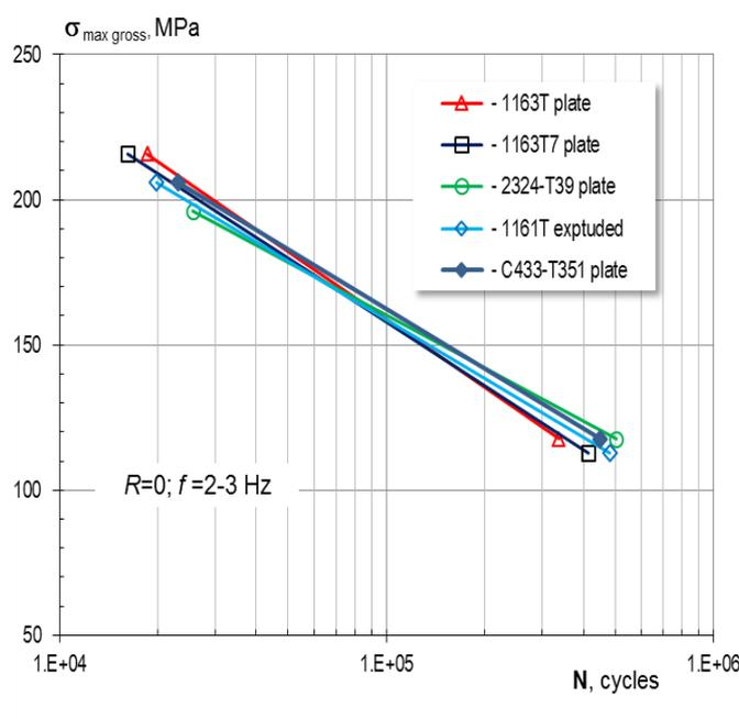
Figure 3.1.1 Fatigue curve of the wing lower surface material
