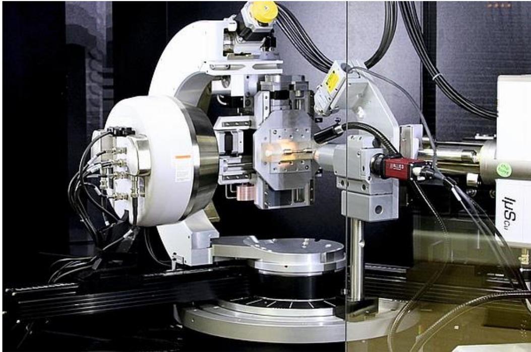
Figure 12.2.2 Bruker D8 Advance X-Ray Diffraction Meter
