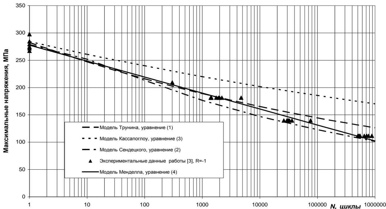
Figure 4.1 Approximation of test data for specimens with open holes. AS4-PW laminate
