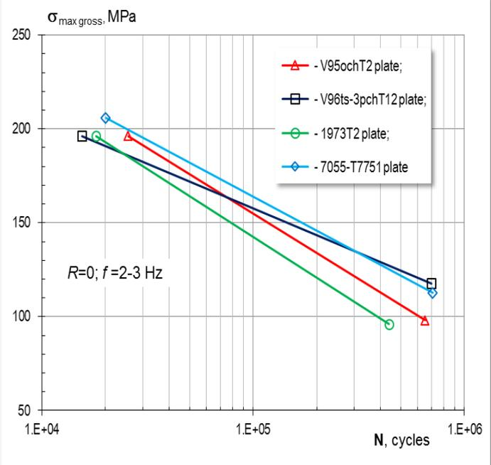
Figure 3.1.2 Fatigue curve of the wing upper surface material
