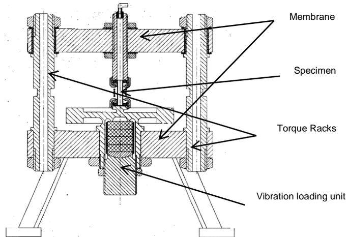
Figure 11.2.1 P926 test rig allowing independent axial cyclic loading at various levels in combination with thermal stresses
