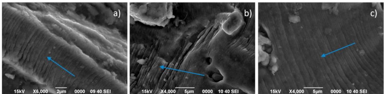
Figure 3.2.1 SEM fractographs of samples (a) S1, (b) S2 and (c) S3. The blue arrow indicates the direction of crack growth.
