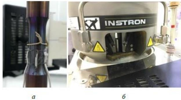
Figure 3.4.2 Samples with attached thermal couples (a) and heat insulation laid down on the upper surface of the high-temperature furnace (b)
