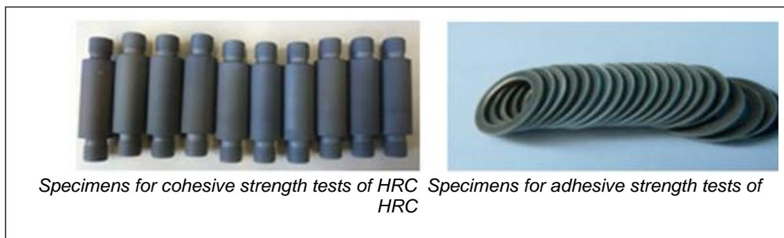
Figure 11.1.1      Specimens to determine the strength properties of HRC layers
