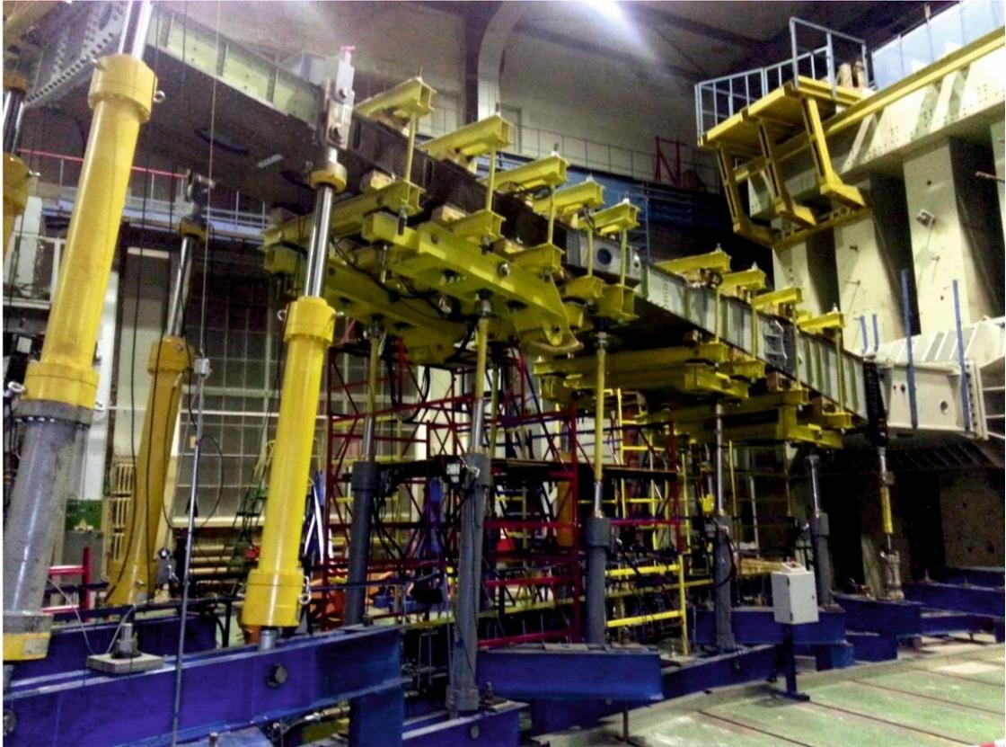
Figure 6.2 Fatigue tests and residual strength test of composite wing box structures
