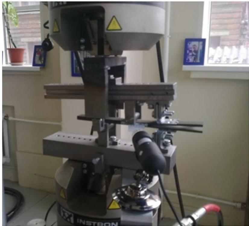
Figure 4.4.1 Test rig for fatigue and crack resistance characteristics studies, advanced CFRP material. Mixed mode testing at TsAGI lab.
