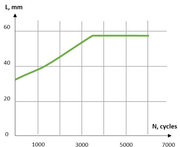
Figure 8.2.3 Crack growth in emergence door frame obtained experimentally
