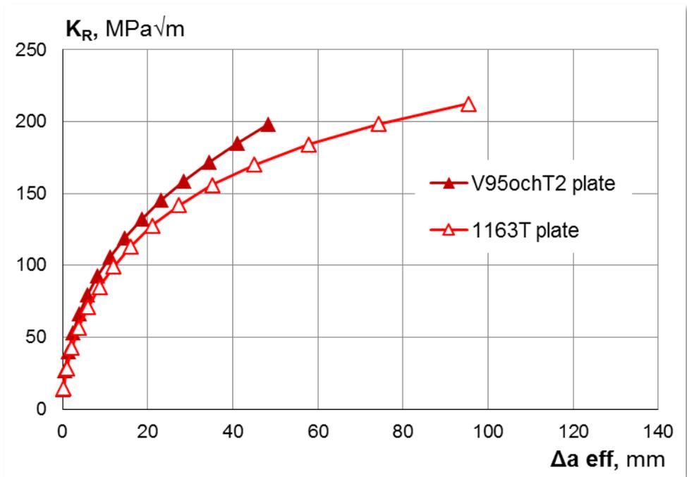
Figure 3.1.7 R-curves of the wing upper and lower surface material
