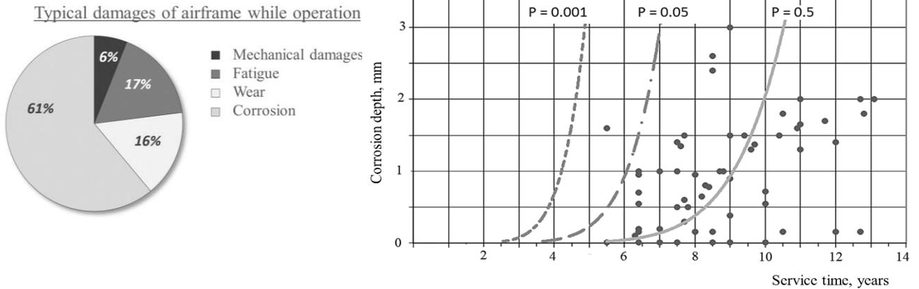
Figure 9.2. Operational damages of IL86 airframe and propagation of layer corrosion in aluminum wing lower surface panels at operation conditions
