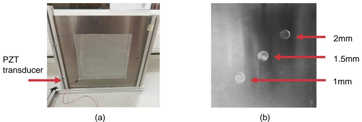
*Figure 1: (a) scan surface and driving PZT sensor (b) Back face of test specimen with thinning*
