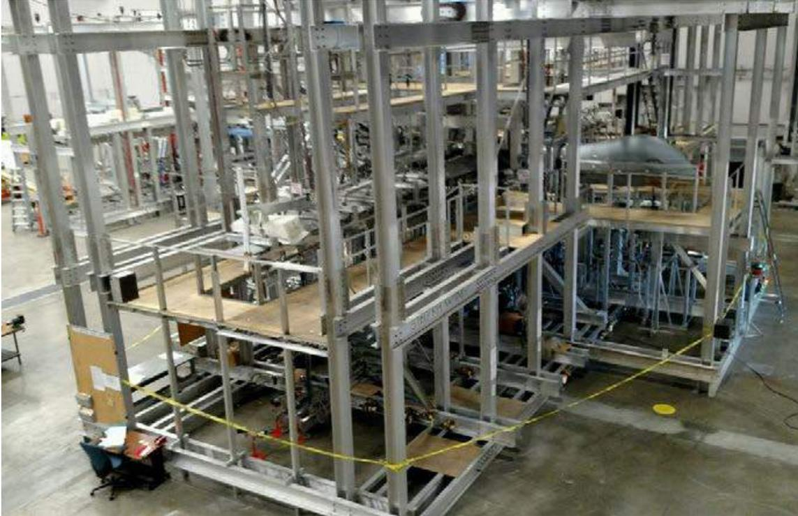
**Figure 9.11-14. Full-Scale Fatigue Test**
