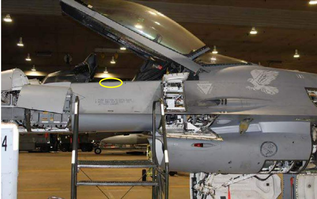
Figure 9.11-41. Canopy Sill Longeron Ladder Damage Area
