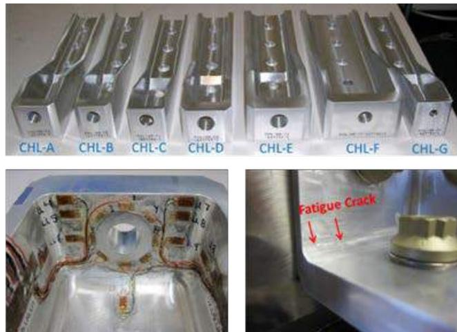
**Figure 9.6-100. Fatigue and Residual Strength Testing and Analysis of Tension Fittings**
