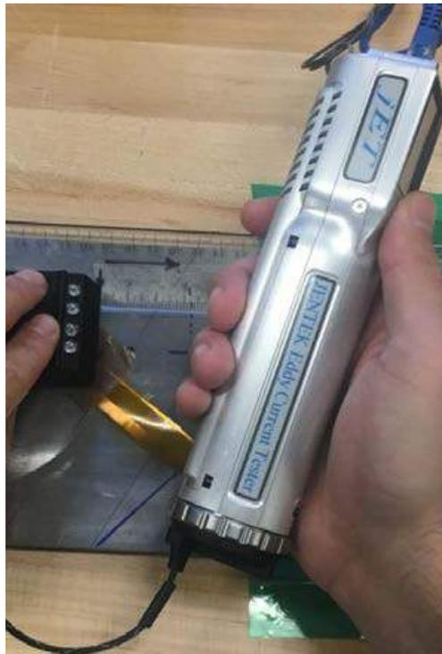
**Figure 9.2-18. MWM-Array Eddy Current Sensor**
