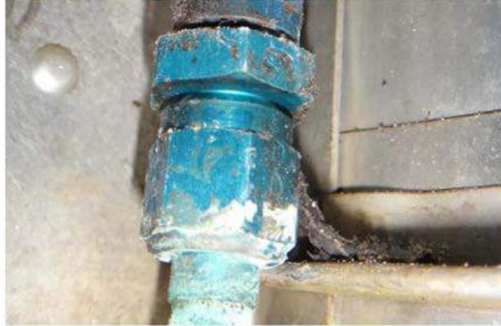
Figure 9.11-2. Example of a Minor Corrosion Finding
