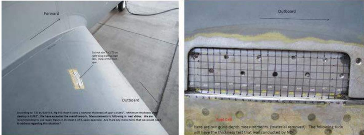
Figure 9.11-4. Example of a Severe Corrosion Finding
