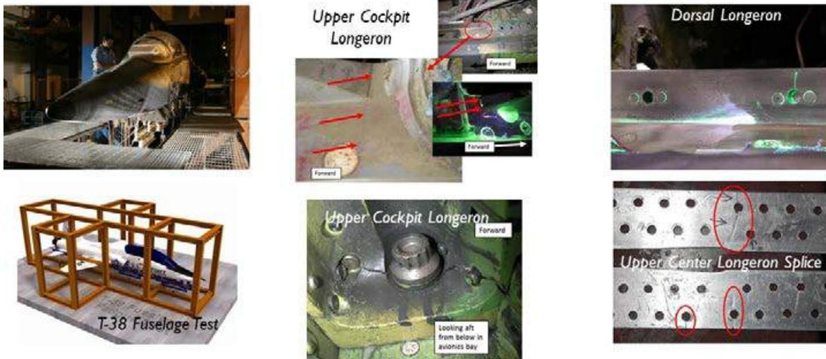
Figure 9.11-15. T-38 Full-Scale Fatigue Test Findings
