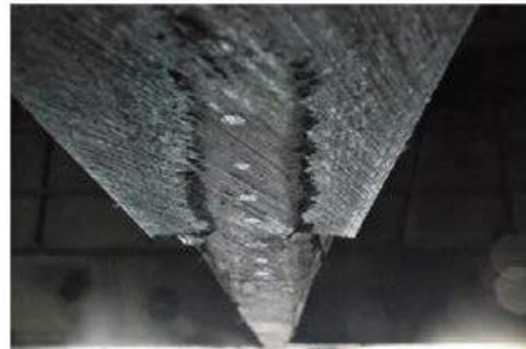
Wear to the centerline keel on the underside of the aircraft
