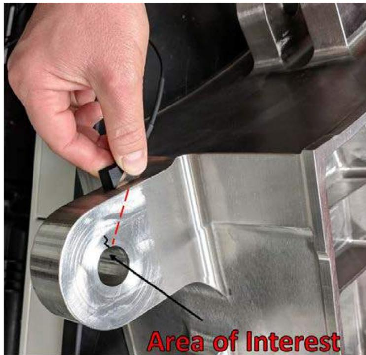
Figure 9.2-11. Shear Wave Applications - Lugs
