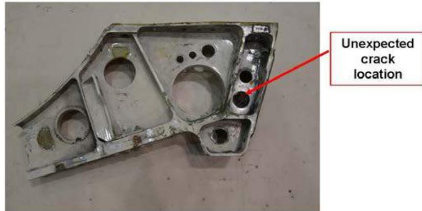
Figure 9.11-23. Unexpected Cracking at 16B5245 Lower Bulkhead at FS 325
