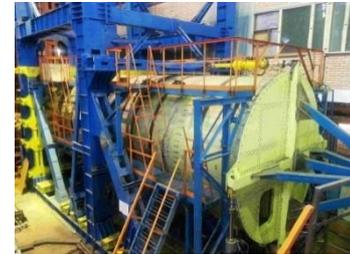
Full scale fatigue test of fuselage section
