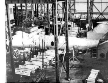
Full scale fatigue test of Yakovlev 40
