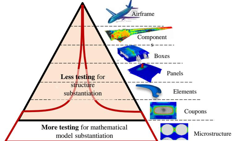
From the “Testing Pyramid” to the “Virtual-testing pyramid”
