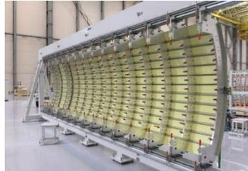
More than 30 fuselage panels of different configuration have been tested to support certification
