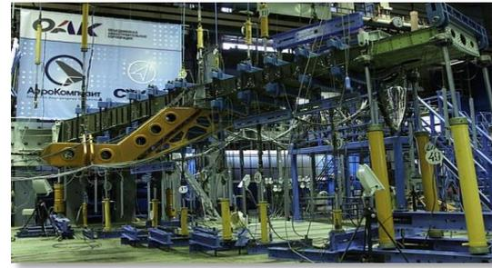
Number of various configuration wing panels have been tested to be followed by full-scale wing tests
