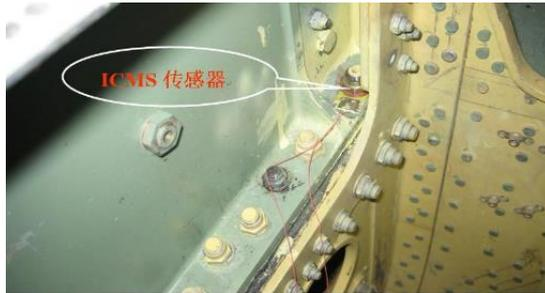
**Intellective Coating Monitoring System in Full-Scale Fatigue Test of Aircraft**
