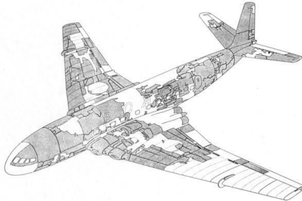
FIG. 2. DIAGRAM SHOWING AMOUNT OF WRECKAGE RECOVERED—G-ALYP.
