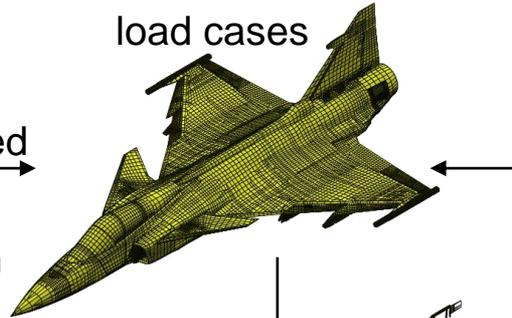
Selection and extraction of local load sequences for any structural part of the model
