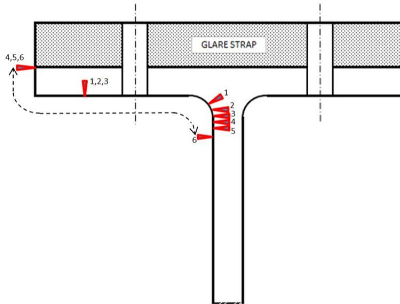
**Figure 10: Measurement Points of the relevant damage during FSFT**
