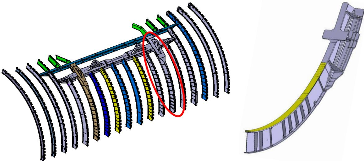
**Figure 2: Main Frame of wing load introduction**
