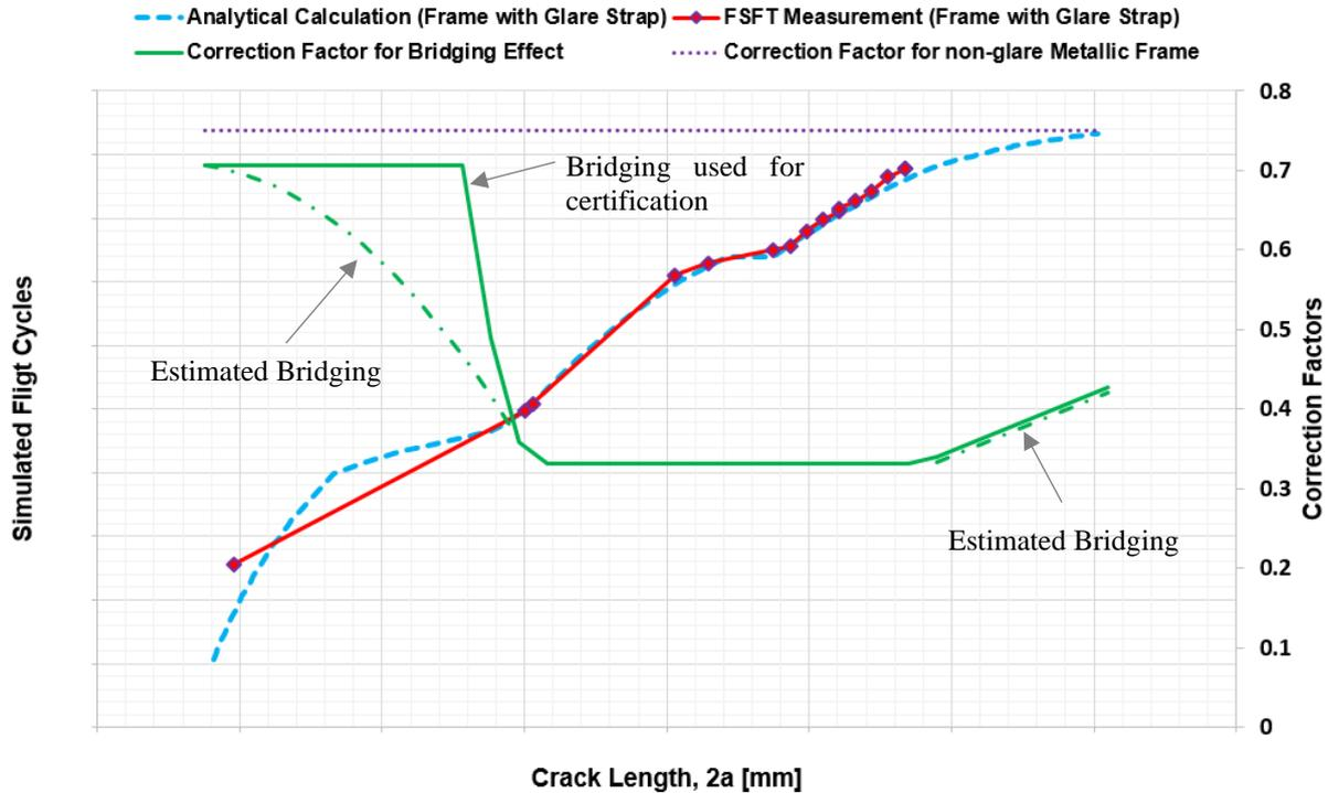
**Figure 12: Crack growth result vs bridging capability of GLARE®**
