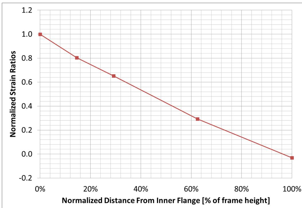
**Figure 8: Strain measurements in frame web**
