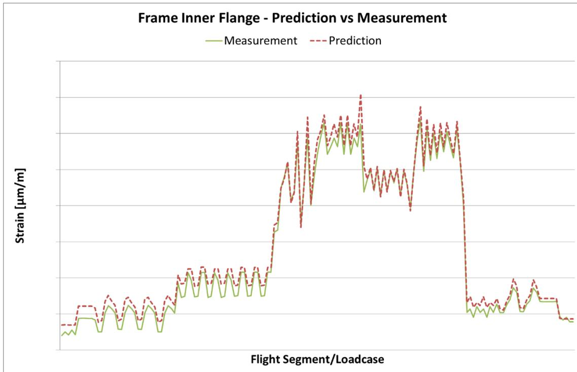
**Figure 6: Strain measurements vs prediction comparison**
