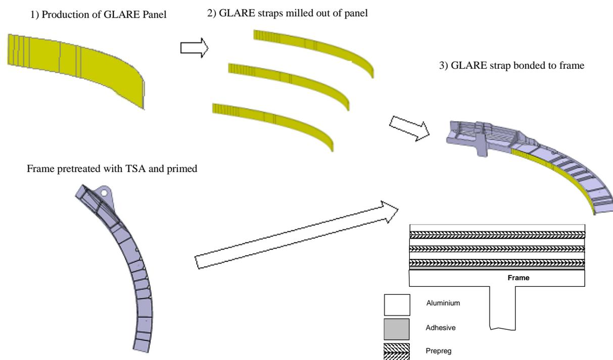
**Figure 3 GLARE® Strap manufacturing**
