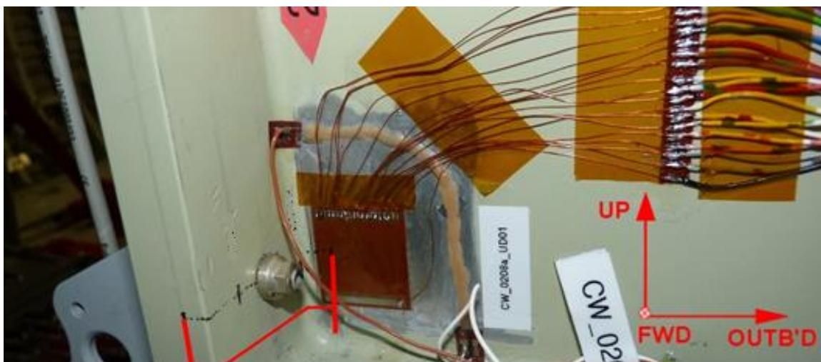
**Figure 9: Crack wire installation**
