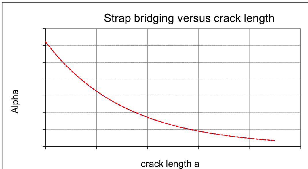
**Figure 4 Crack bridging correction used in design phase**
