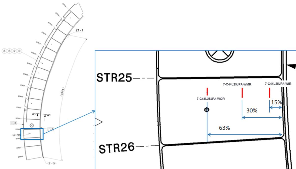
**Figure 7: Strain gauge installation in frame web**
