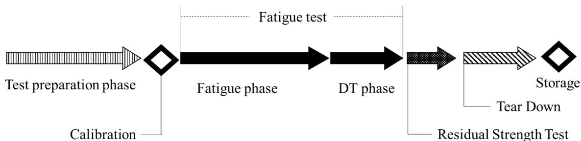
**Figure 5: Description Airbus FSFT procedure**
