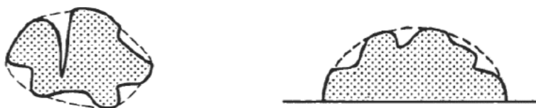
Figure 4: Irregularly Shaped Cracks
