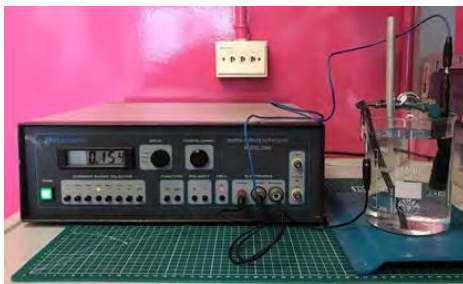
Figure 12: Setup of the Galvanostatic Test
