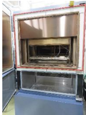
Figure 5: Thermal shock chamber used for the temperature controlled test
