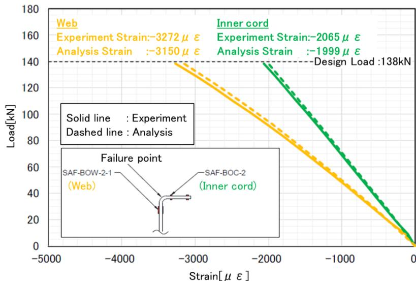
Figure 6: Load-Strain behaviour of conventional design frame
