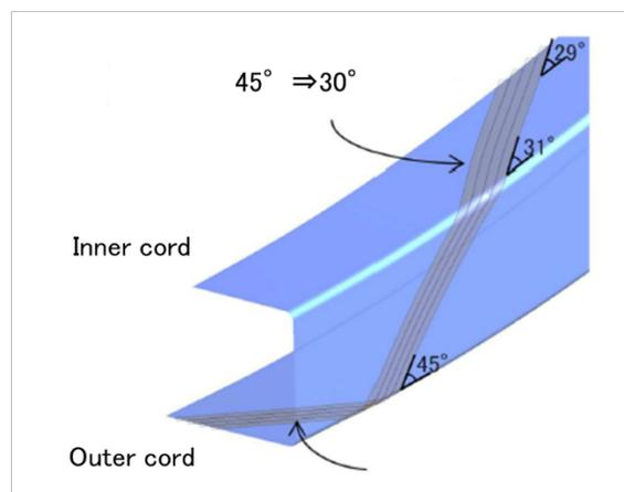
Figure 4: Ply table and steering ply of optimal design frame
