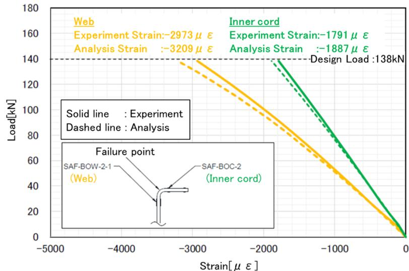
Figure 7: Load-Strain behaviour of optimal design frame
