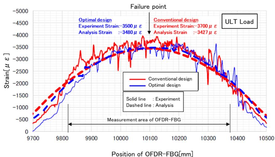
Figure 8: Strain distribution of corner of inner cord
