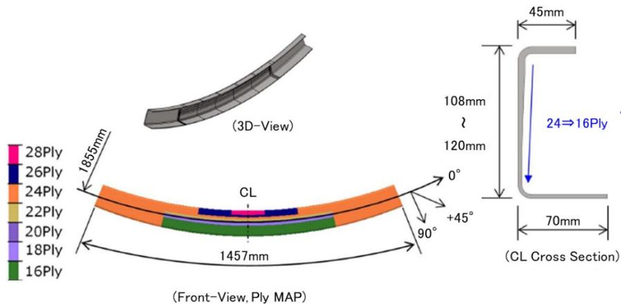
Figure 3: Optimal design frame
