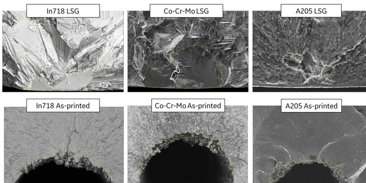
Figure 4: Example of anomaly size measurement on fracture surfaces of LSG and as-printed fatigue coupons.
