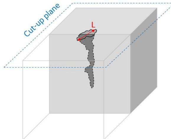
Figure 2: Example of measurement of anomaly size in the case of anomaly elongated perpendicular to cut-up plane.
