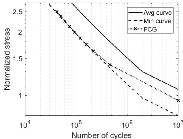
Figure 1: Comparison of FCG results based on calculated IFS against average and minimum fatigue allowable for L-PBF In718 tested at room temperature.
