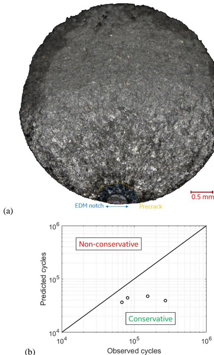
Figure 5: Validation tests on In718. (a) Fractography of one specimen for 25% knockdown verification; (b) Comparison of observed vs predicted life for precracked coupons.
