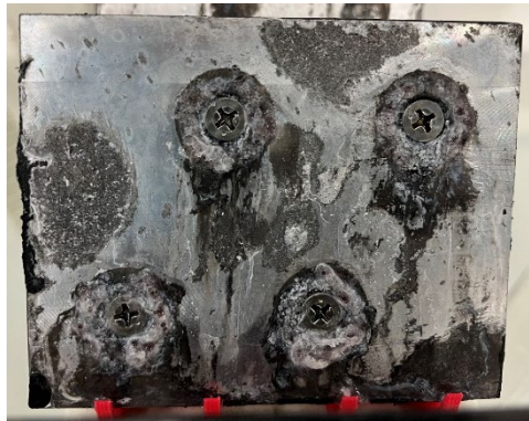
Figure 14: Repaired coupon after 168 hours of exposure.
