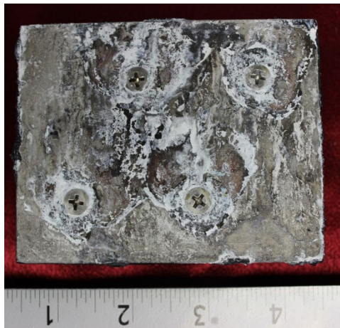
Figure 15: Repaired coupon after 1000 hours of exposure and clean water rinse.
