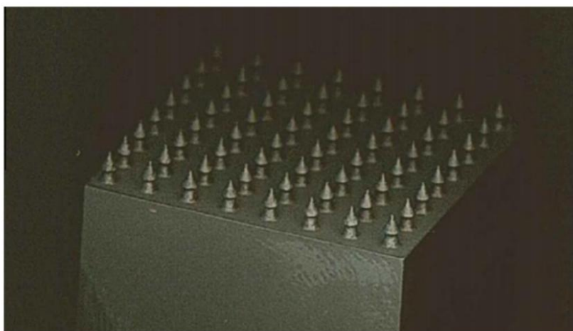
Figure 4. An array of additively manufactured, titanium HYPERS pins[20]
