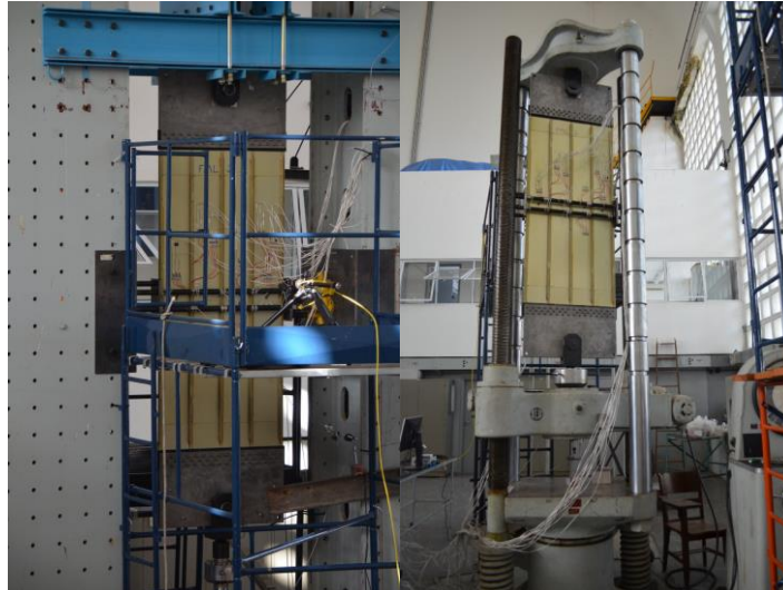
Figure 3 Experimental test setup for fatigue (left) and residual strength (right) characterization
