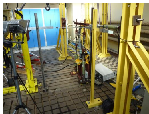
Figure 4. Example of L-ILOt modular test stand for landing gear testing (source: L-ILOt)
