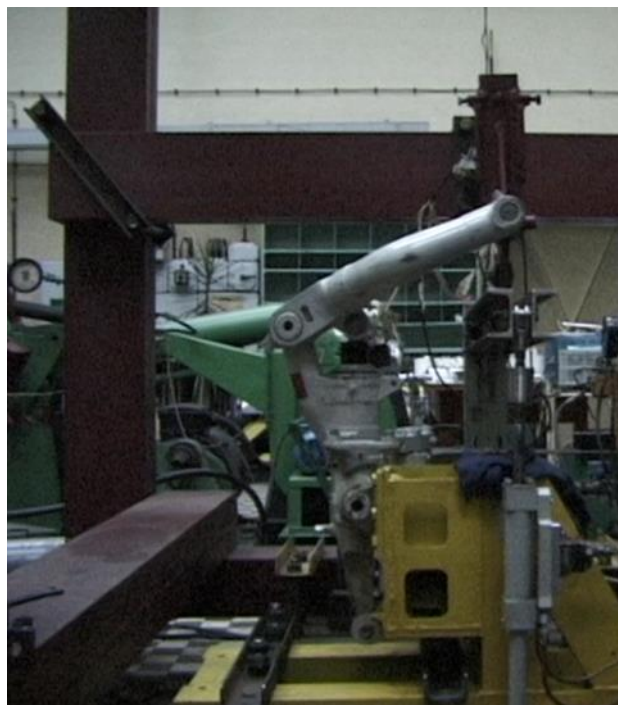
Figure 2. Example of multi component quasistatic fatigue test (source: L-ILOT).
