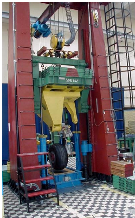
Figure 1. 10 Ton Drop Test Stand (Semi-Automatic) (source: L-ILOT).
